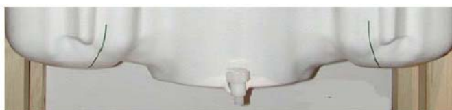
Figure 7.2 SAM Twin Phantom shell
