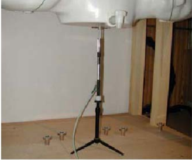
Figure 12.1 Dipole Validation Test Setup
