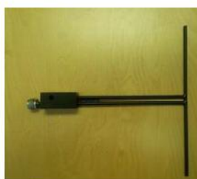
Figure 1 – MVG COMOSAR Validation Dipole
