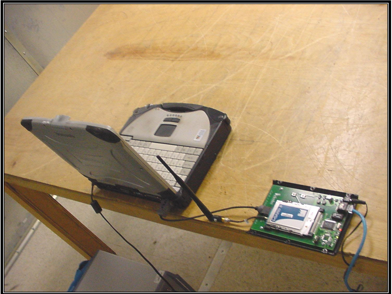
PHOTOGRAPH 12: CONDUCTED TEST CONFIGURATION ( \frac{1}{2} WAVE WHIP ANTENNA REAR VIEW)
