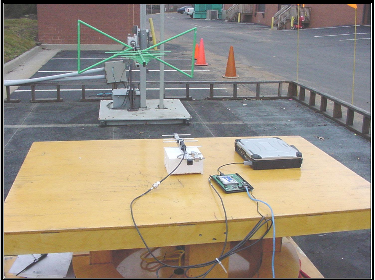
PHOTOGRAPH 8: RADIATED TEST CONFIGURATION (YAGI ANTENNA REAR VIEW)
