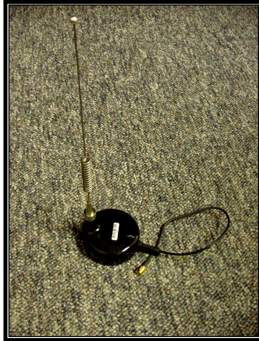
PHOTOGRAPH 14: MAGNETIC MOUNT WHIP ANTENNA
