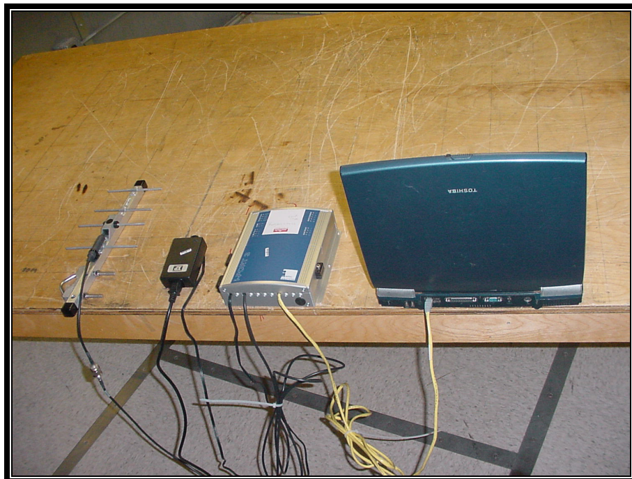
PHOTOGRAPH 13: CONDUCTED EMISSIONS TEST CONFIGURATION - YAGI ANTENNA BACK VIEW
