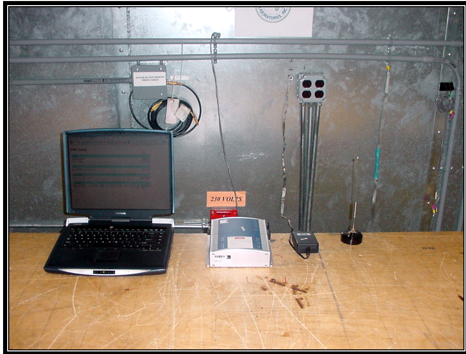
PHOTOGRAPH 8: CONDUCTED EMISSIONS TEST CONFIGURATION - MAGNETIC MOUNT WHIP ANTENNA FRONT VIEW
