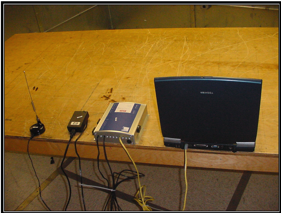
PHOTOGRAPH 9: CONDUCTED EMISSIONS TEST CONFIGURATION - MAGNETIC MOUNT WHIP ANTENNA BACK VIEW
