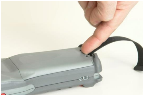
Figure 3: Inserting the Battery
