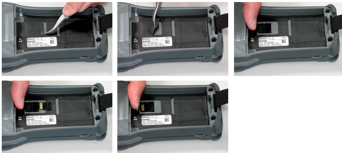
Figure 10: Insert the \mu SD card into the \mu SD card slot
