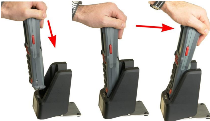
Figure 4: Inserting the M260SE into the DS260
