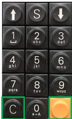
Figure 8: Switching off the M260SE
