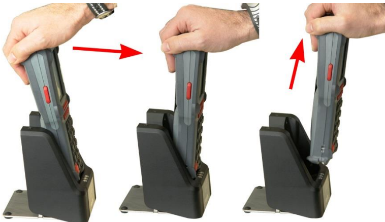
Figure 5: Removing the M260SE from the DS260
