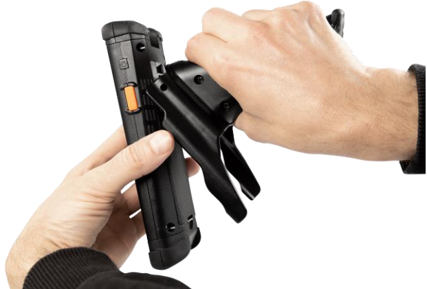
Figure 26: Removing M2Grip5 from M2Smart® SE (2/2)
