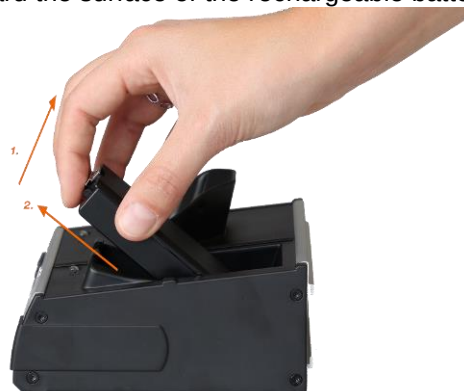
Figure 18: Removing replacement rechargeable battery in the docking station
