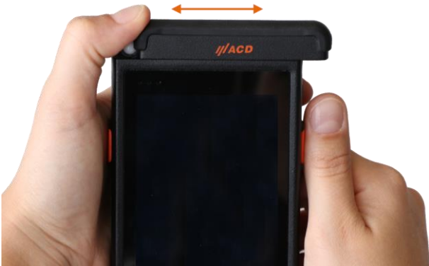
Figure 10: Attaching and removing the upper plug-in module
