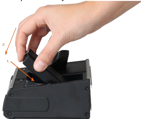
Figure 20: Inserting replacement rechargeable battery in the docking station
