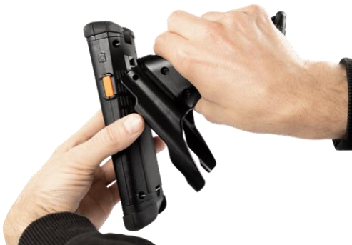
Figure 24: Attaching M2Grip5 to M2Smart® SE
