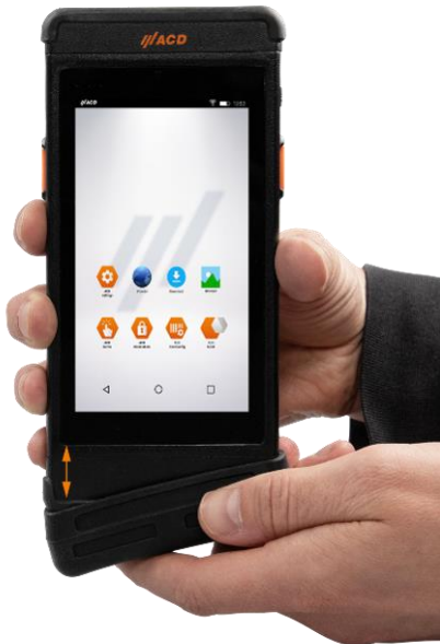
Figure 31: Removing the lower logistics protective cap
