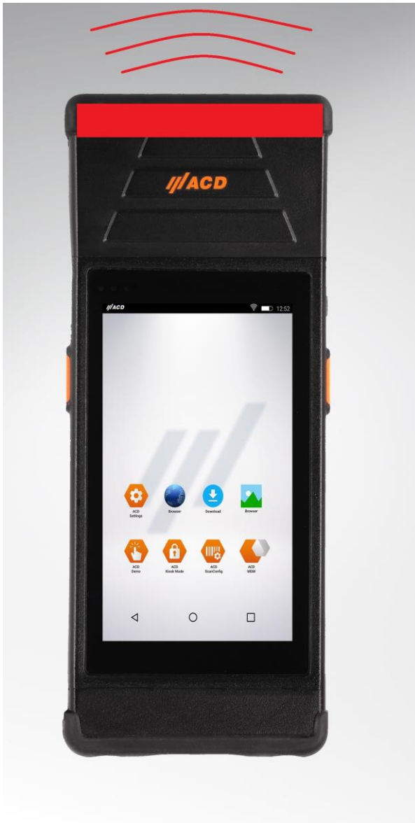
Figure 15: M2UHF-RFID Shortrange Antenna and Radiation
