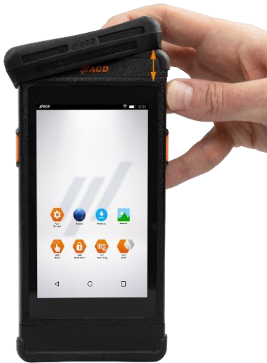
Figure 30: Removing the upper logistics protective cap
