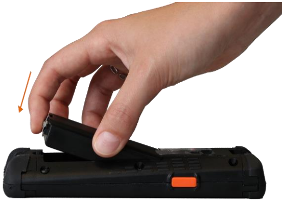
Figure 33: Inserting the rechargeable battery
