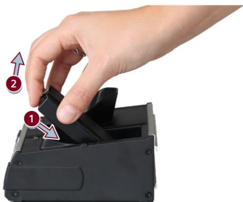
Figure 4-6 Removing a battery from the charging/docking station
