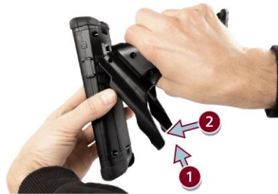
Figure 4-13 Attaching the pistol handle
