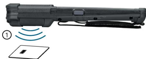
Figure 4-7 Radiation of the antenna field of the HF head module
