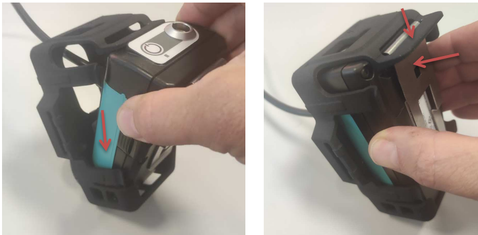
Figure 6: Inserting the Voxter VT5 into the Voxter Vehicle Mount
