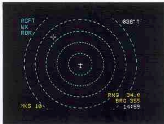
Range and Bearing To A Selected Target
