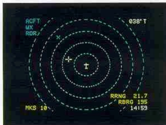
Range and Bearing Between Two Selected Targets
