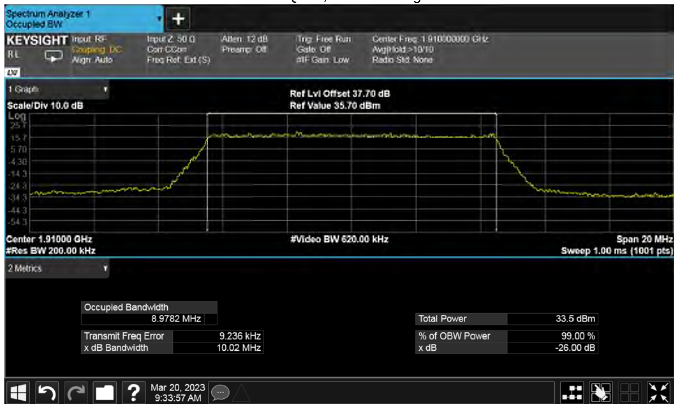
Plot for 99 % Bandwidth (MHz) Nominal Temp & Volts
