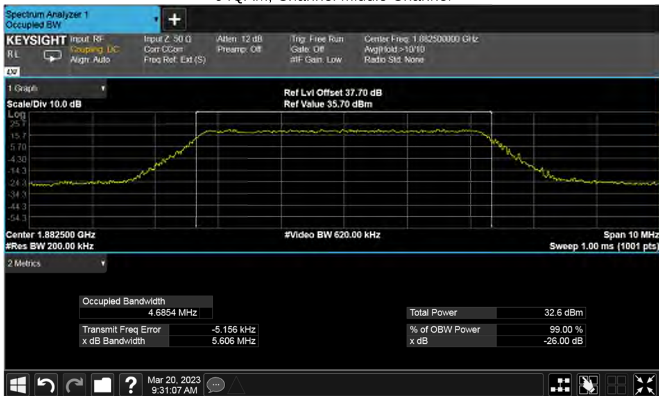
Plot for 99 % Bandwidth (MHz) Nominal Temp & Volts
