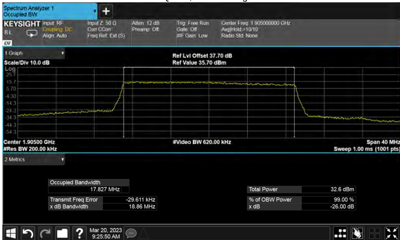
Plot for 99 % Bandwidth (MHz) Nominal Temp & Volts
