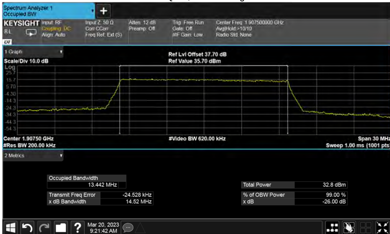
Plot for 99 % Bandwidth (MHz) Nominal Temp & Volts
