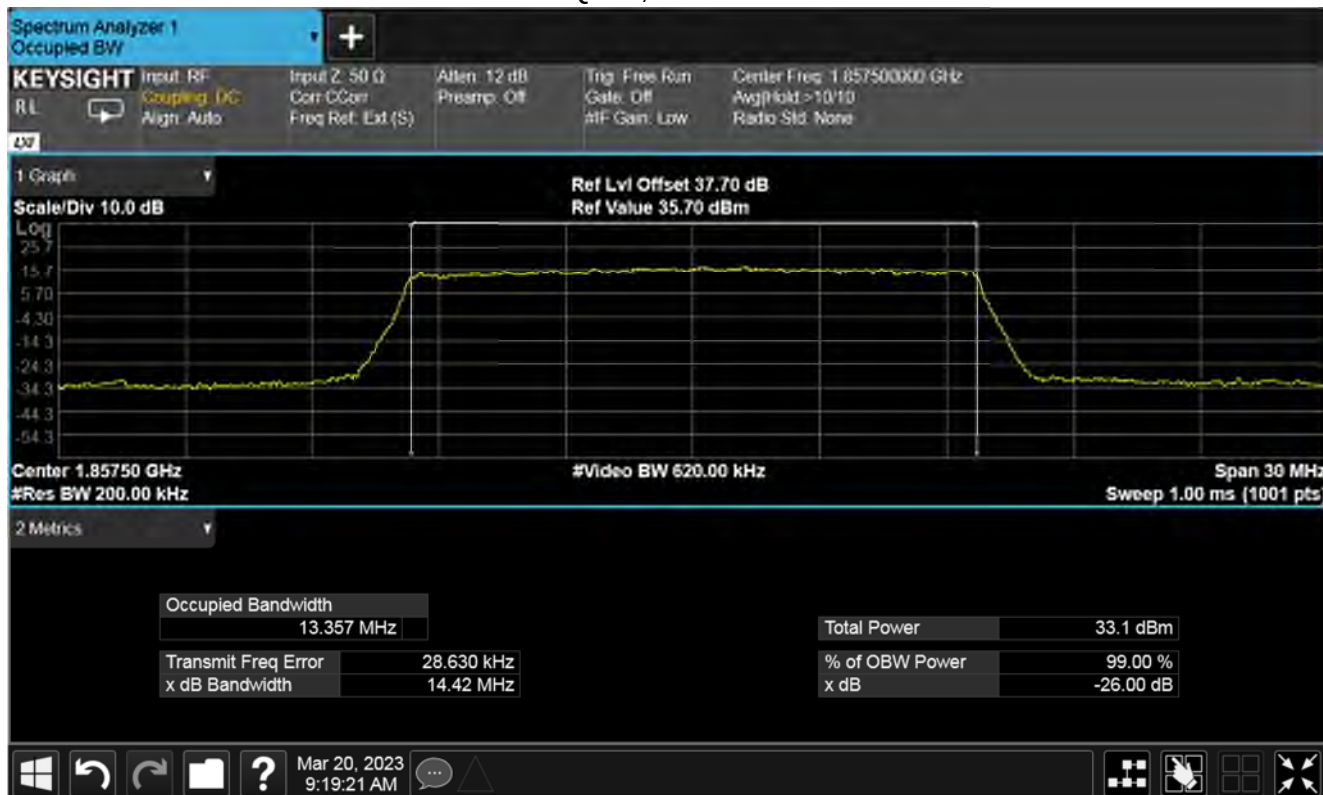
Plot for 99 % Bandwidth (MHz) Nominal Temp & Volts
