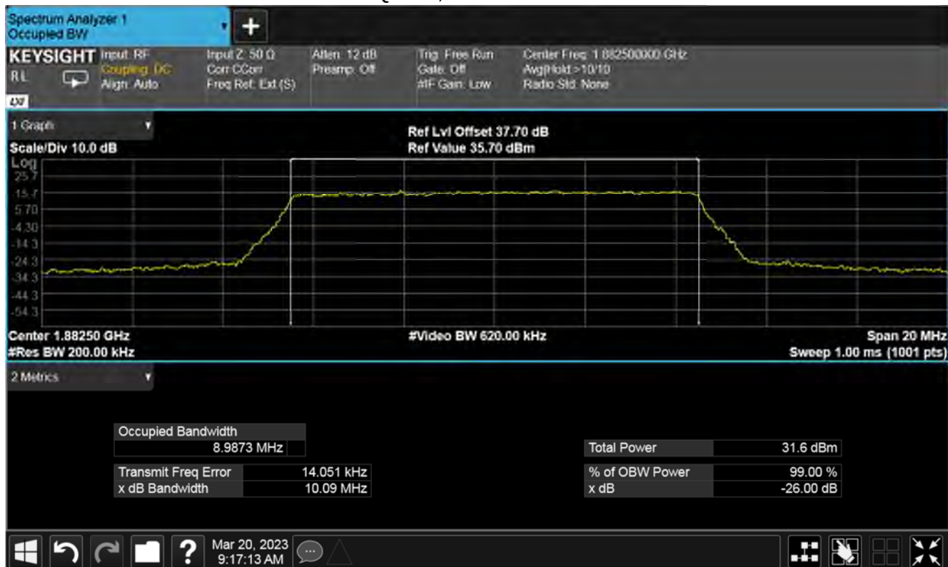
Plot for 99 % Bandwidth (MHz) Nominal Temp & Volts
