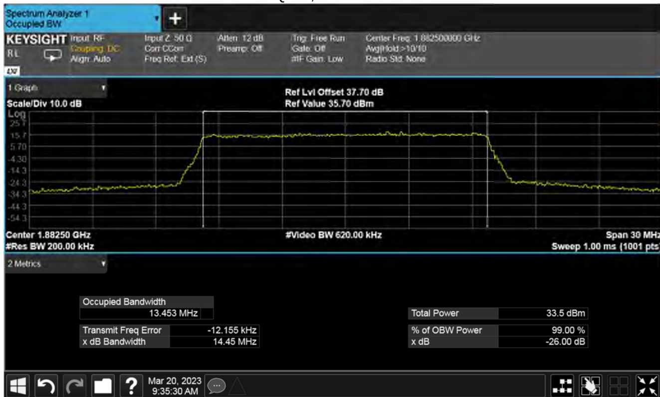
Plot for 99 % Bandwidth (MHz) Nominal Temp & Volts
