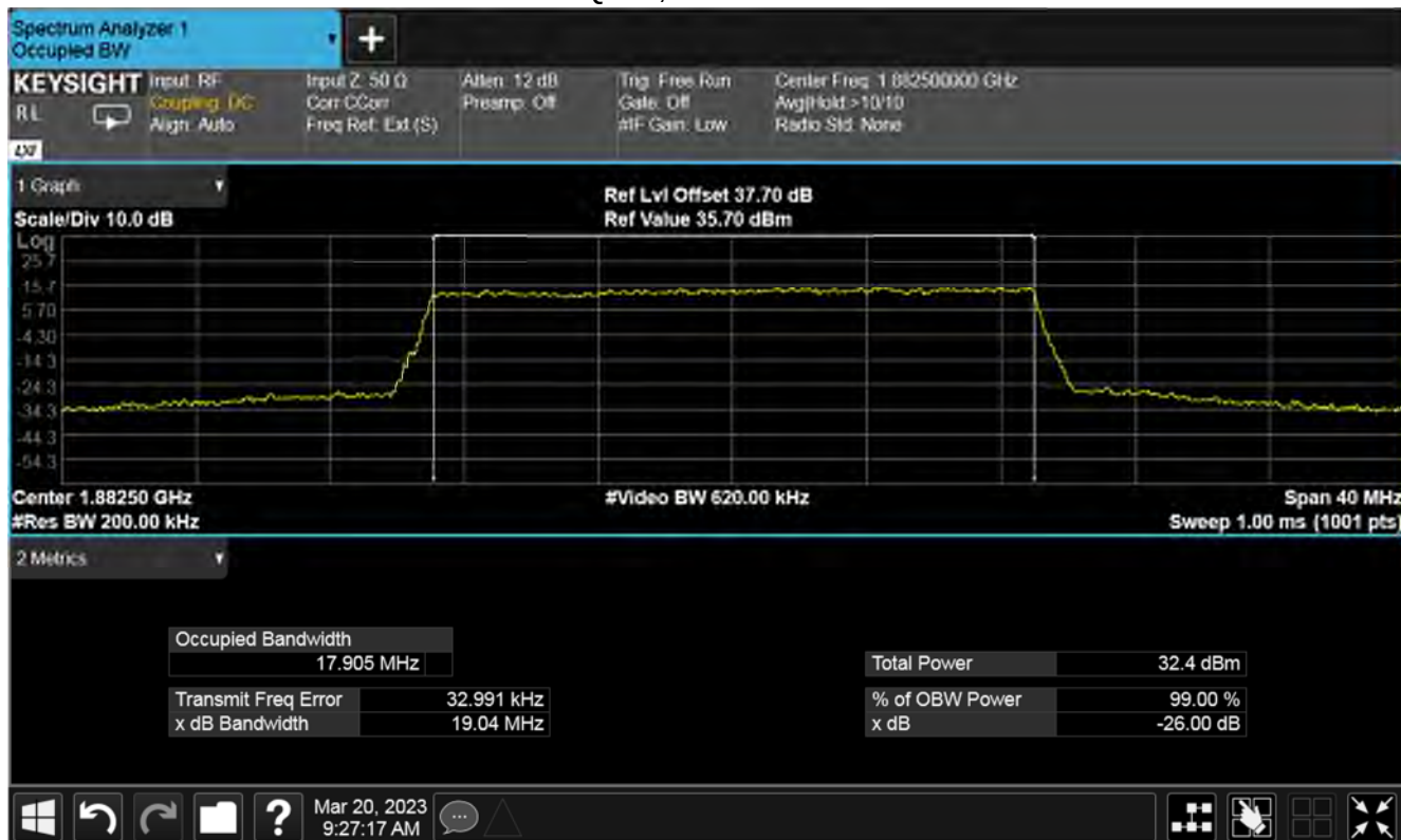
Plot for 99 % Bandwidth (MHz) Nominal Temp & Volts
