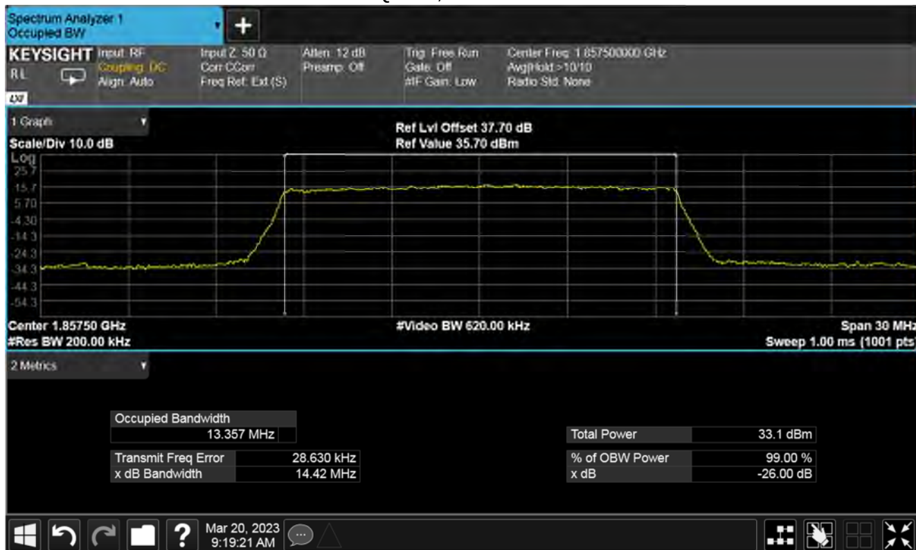
Plot for 99 % Bandwidth (MHz) Nominal Temp & Volts
