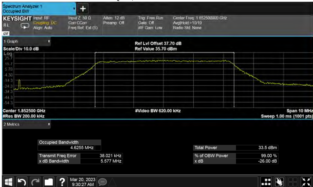
Plot for 99 % Bandwidth (MHz) Nominal Temp & Volts
