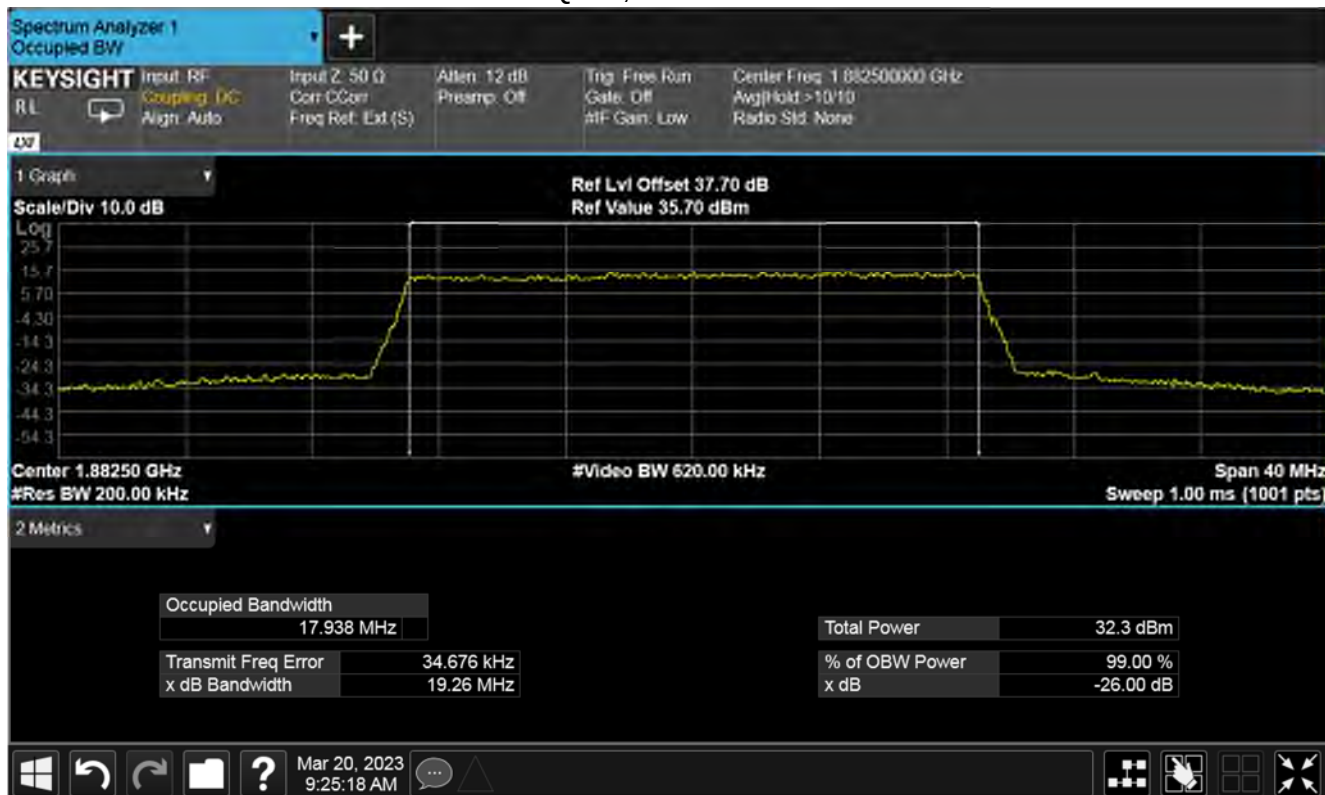
Plot for 99 % Bandwidth (MHz) Nominal Temp & Volts
