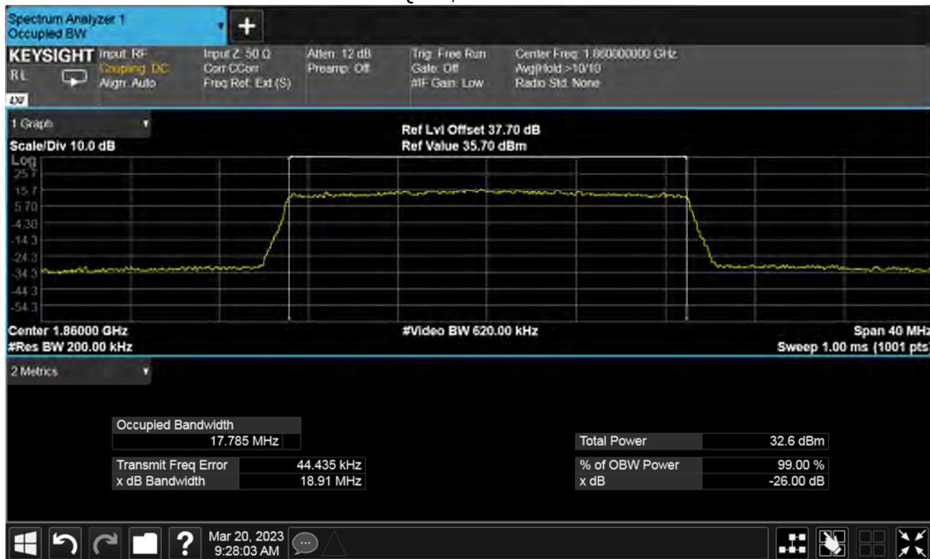
Plot for 99 % Bandwidth (MHz) Nominal Temp & Volts
