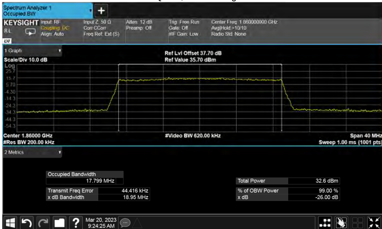
Plot for 99 % Bandwidth (MHz) Nominal Temp & Volts
