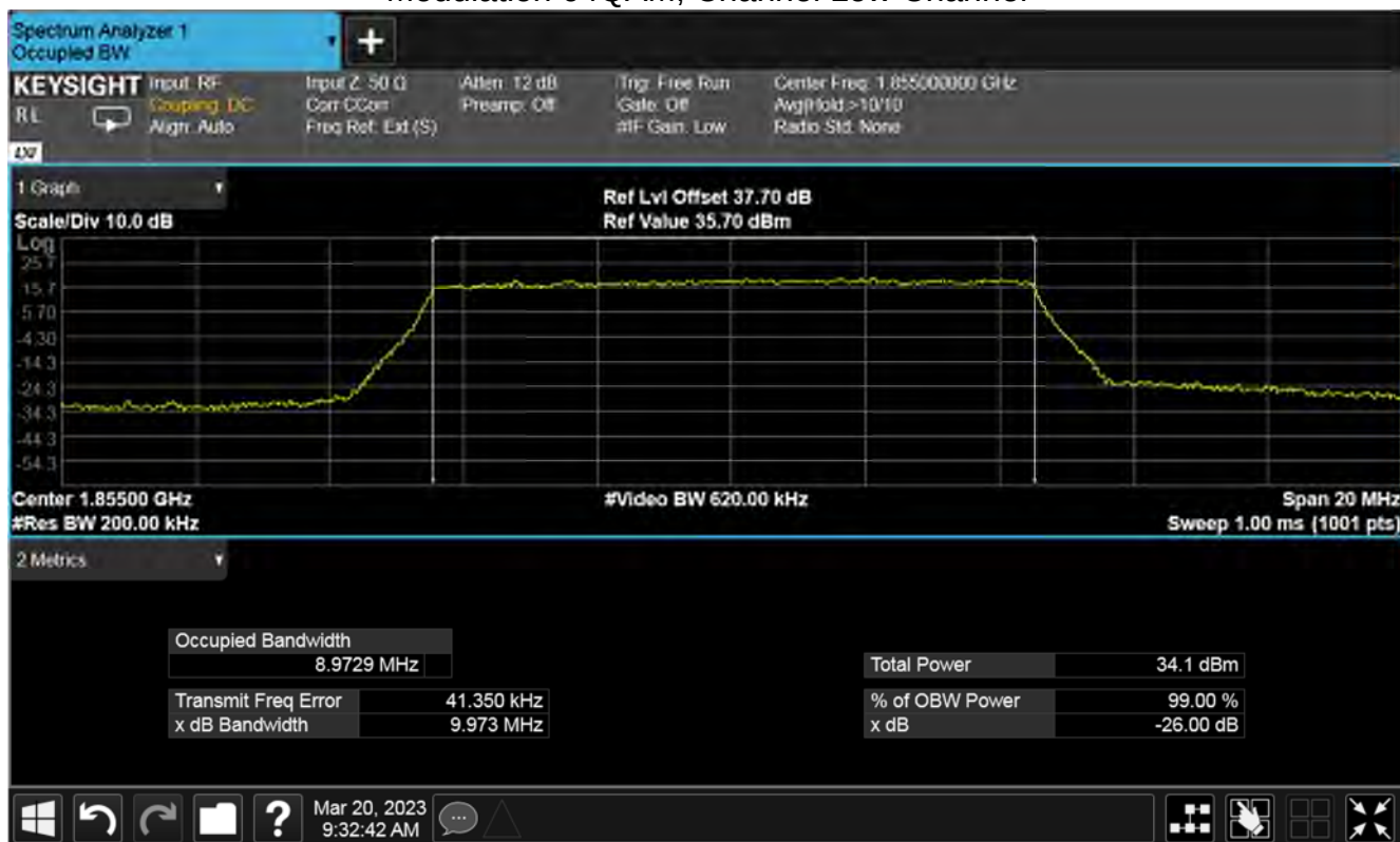
Plot for 99 % Bandwidth (MHz) Nominal Temp & Volts
