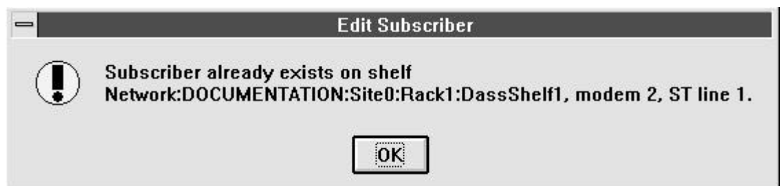
Figure 2-4. Existing Subscriber Warning
