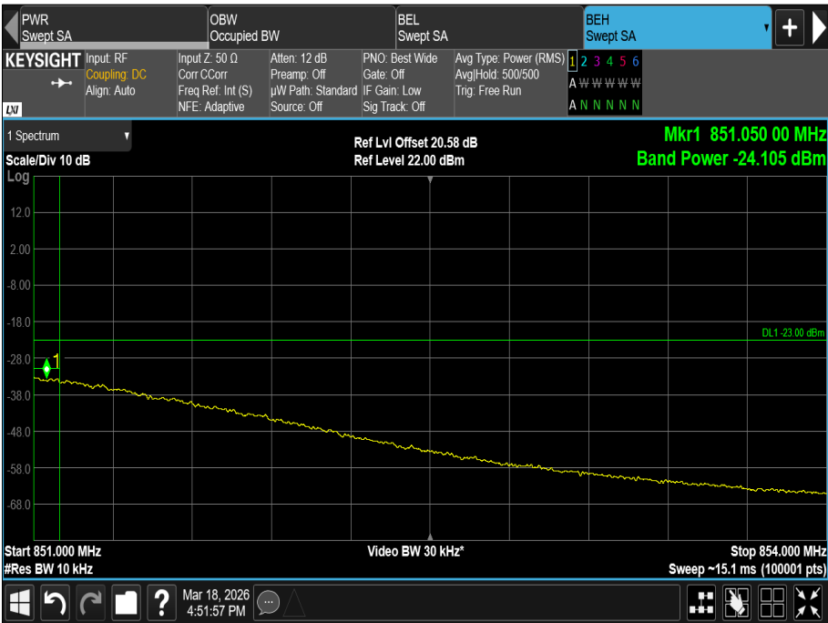
Figure 8 - 850.0 MHz, QPSK, Band Edge Frequency: 851 MHz. Sector 1 (Port V)
