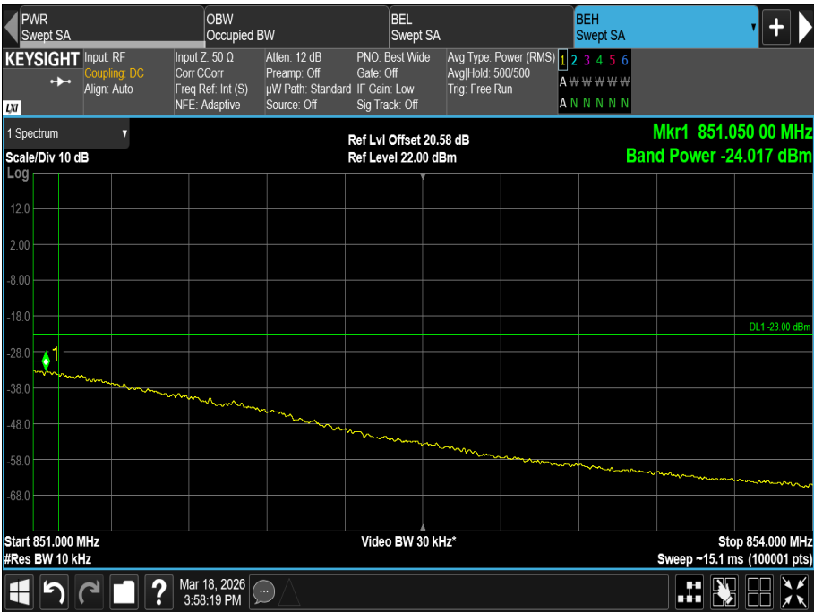
Figure 10 - 850.0 MHz, 16-QAM, Band Edge Frequency: 851 MHz. Sector 1 (Port V)
