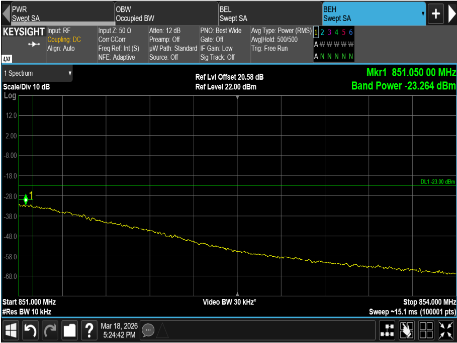
Figure 18 - 850.0 MHz, 64-QAM, Band Edge Frequency: 851 MHz. Sector 1 (Port H)
