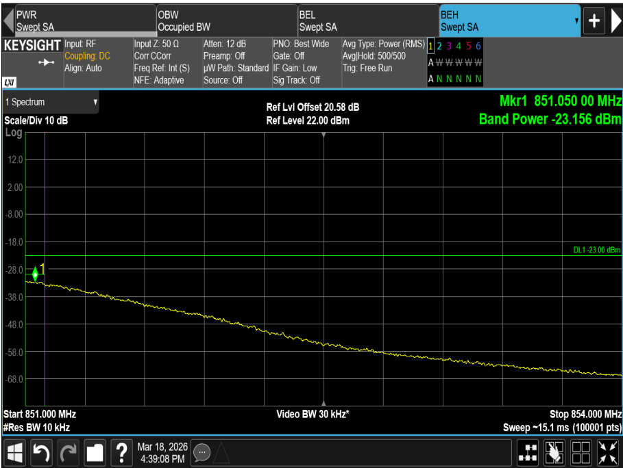
Figure 14 - 850.0 MHz, QPSK, Band Edge Frequency: 851 MHz. Sector 1 (Port H)
