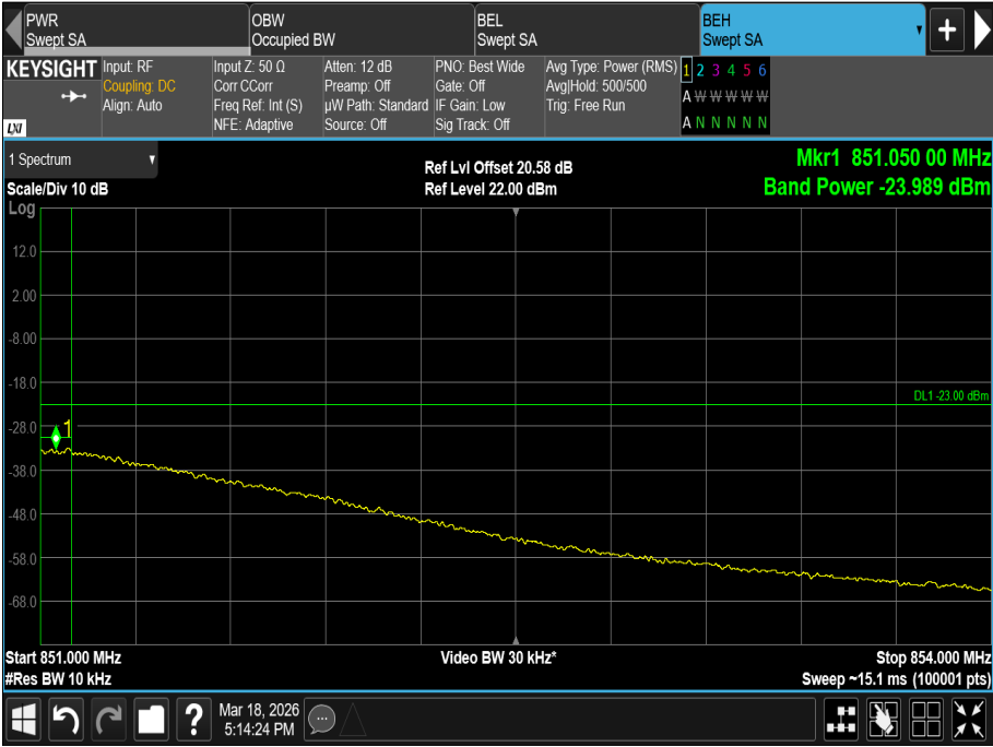
Figure 12 - 850.0 MHz, 64-QAM, Band Edge Frequency: 851 MHz. Sector 1 (Port V)
