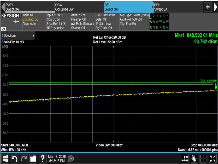
Figure 11 - 850.0 MHz, 64-QAM, Band Edge Frequency: 849 MHz. Sector 1 (Port V)
