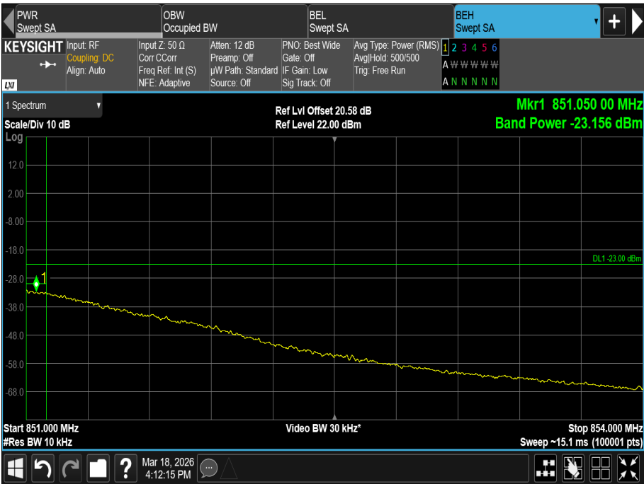
Figure 16 - 850.0 MHz, 16-QAM, Band Edge Frequency: 851 MHz. Sector 1 (Port H)
