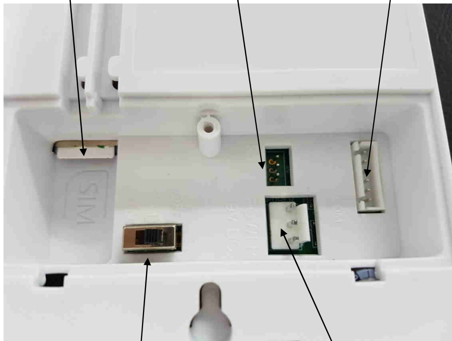
Battery ON-OFF Switch
