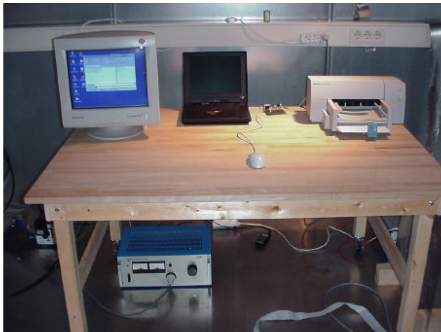
Picture 5 : Setup for conducted emission test on the AC mains
