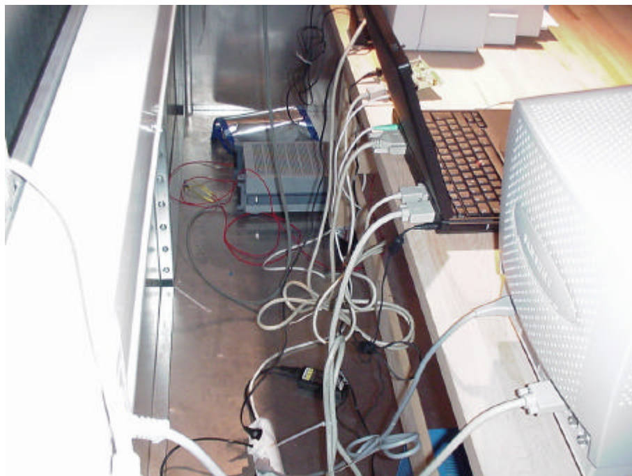
Picture 6 : Setup for conducted emission test on the AC mains (rear side)
