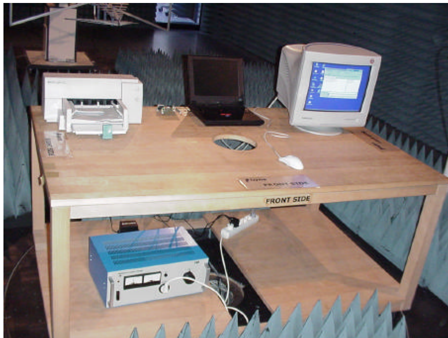
Picture 3 : Setup for radiated emission measurements above 1 GHz
