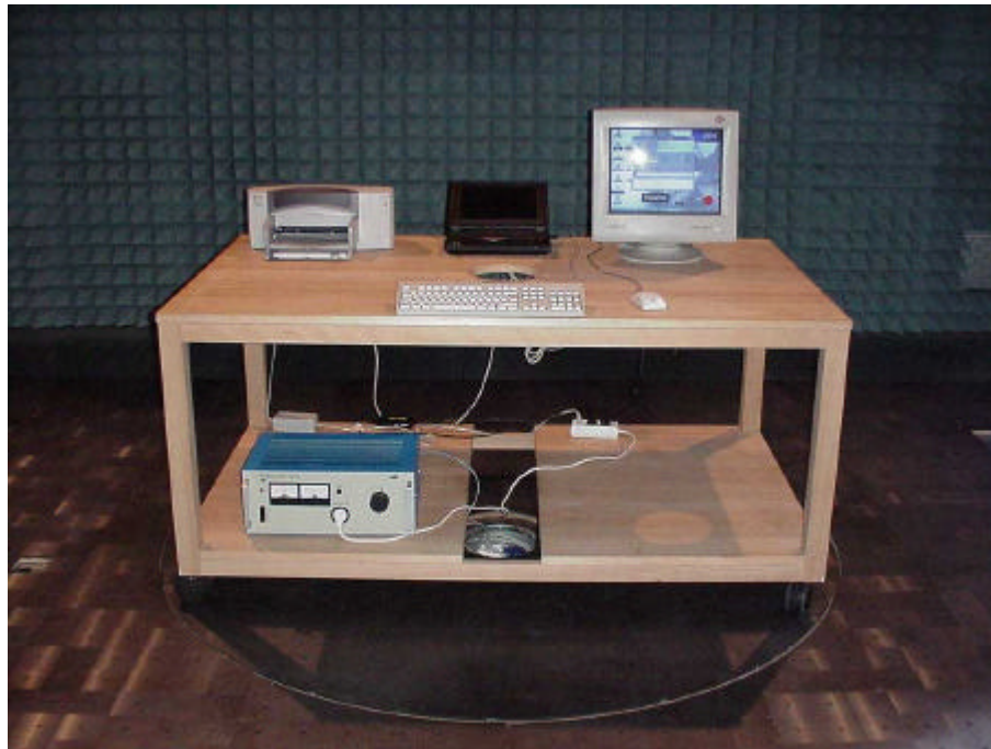
Picture 1 : Setup for radiated measurement, front view
