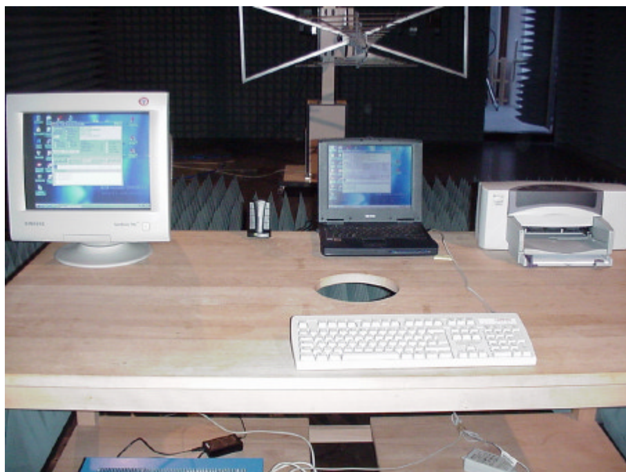
Picture 2 : Test set-up for radiated emissions
