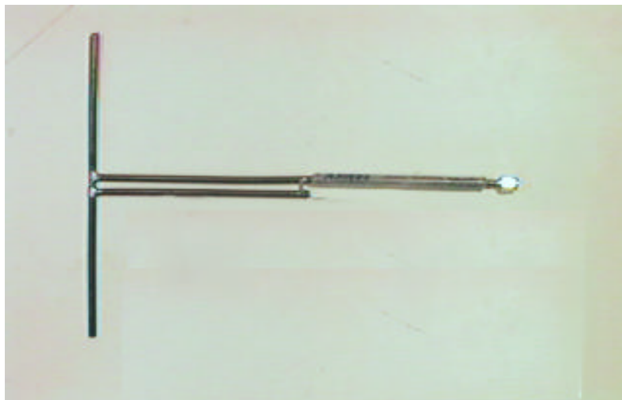
Reference Dipole Antenna Used for ERP Measurement
