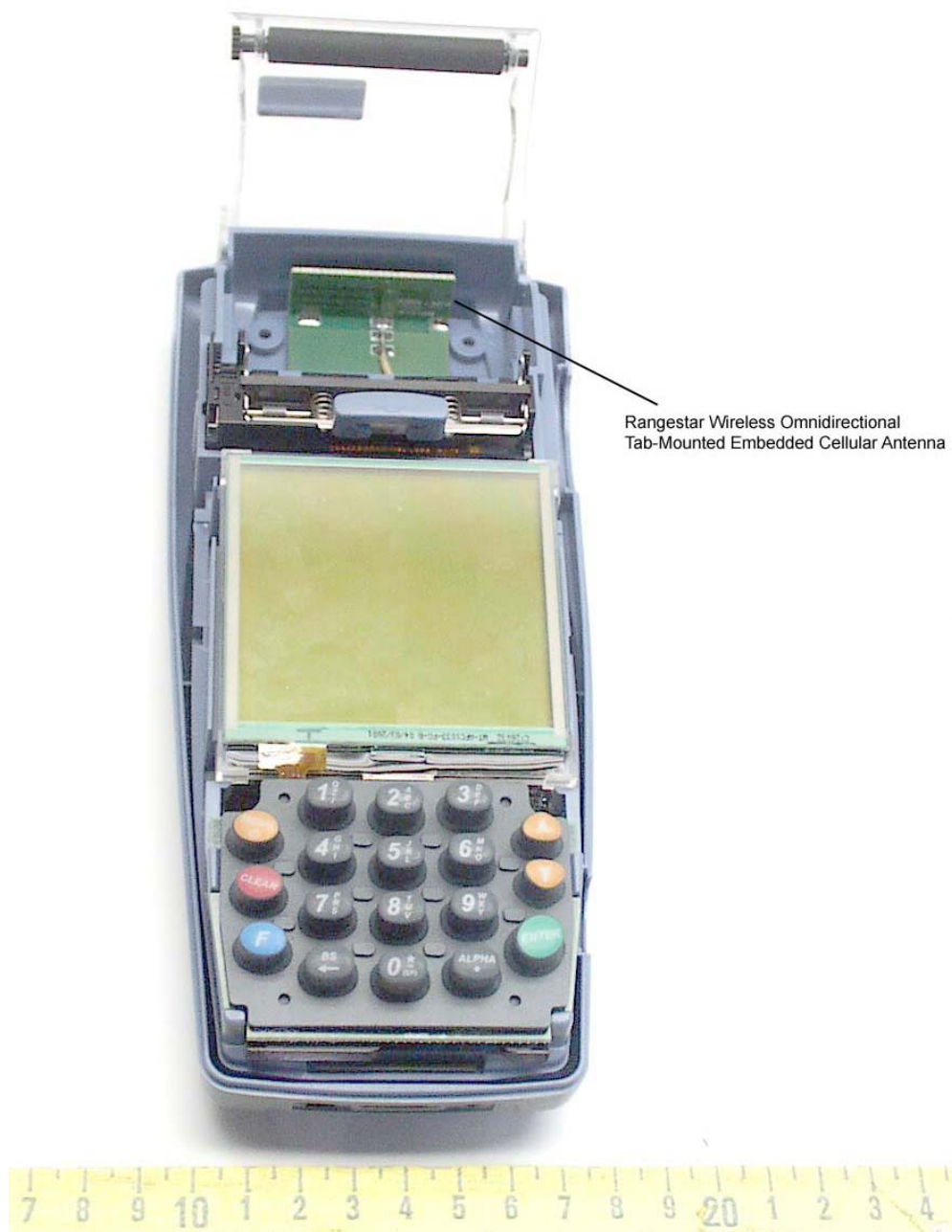
<Front View – Showing Internal Integral Antenna>
