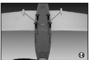
14. Use four screws \phi 2.0 \times 8PB to fix the main wing as shown.(Fig.14)
