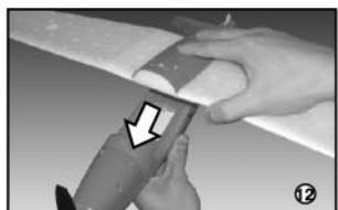
12. Put the main wing on the fuselage as shown.(Fig.12)
