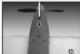
11.Installed by Screw \phi 2.0 \times 6PB
