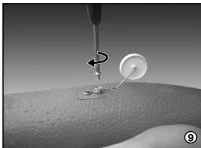
9. Insert the rear landing gear with the screw of \phi 2.3 \times 6 PWB into the back of the plane.(Fig.9)
