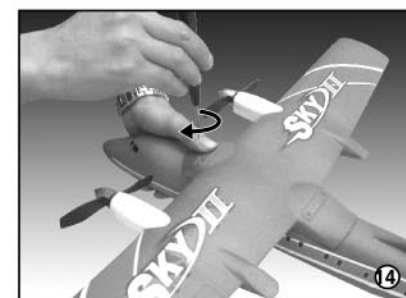
14. Put the main wing on top of the plane and fix it with the \phi 2.0 \times 8 PB screws.(Fig.14)
