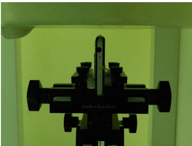
Right Side of the DUT with Phantom 1 cm Gap
