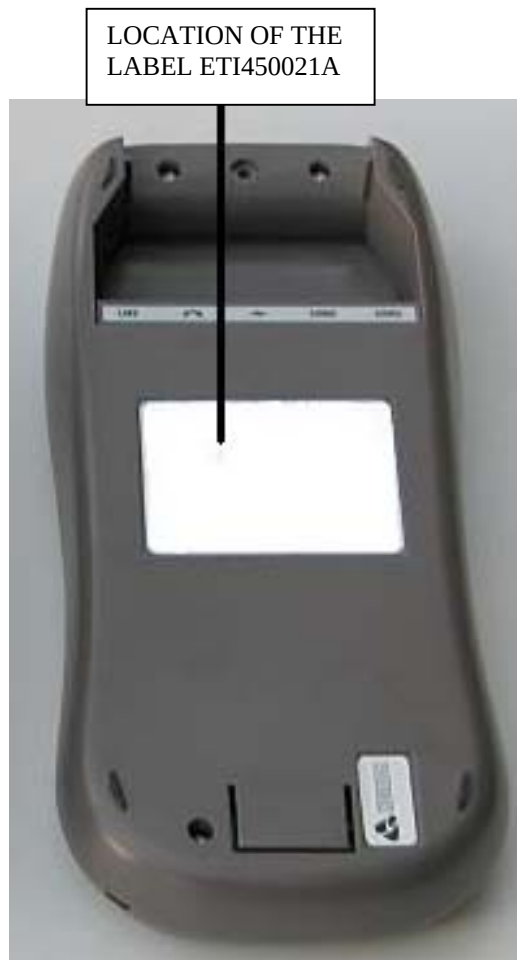
Diagram 2: Position of the product label on i7770 Radio Base with BTv2.
