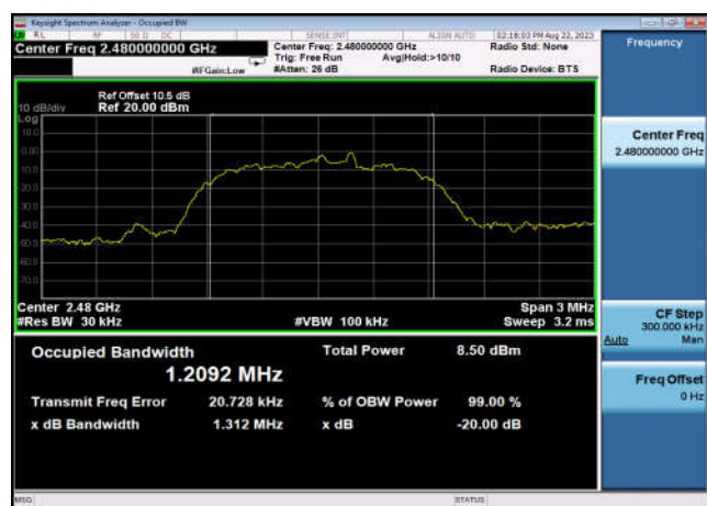
20dB Bandwidth: 8DPSK,2480MHz,3DH5
