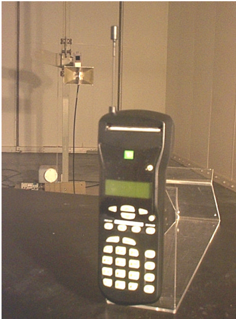
Spurious Emission Testing (for frequencies above 1 GHz)
