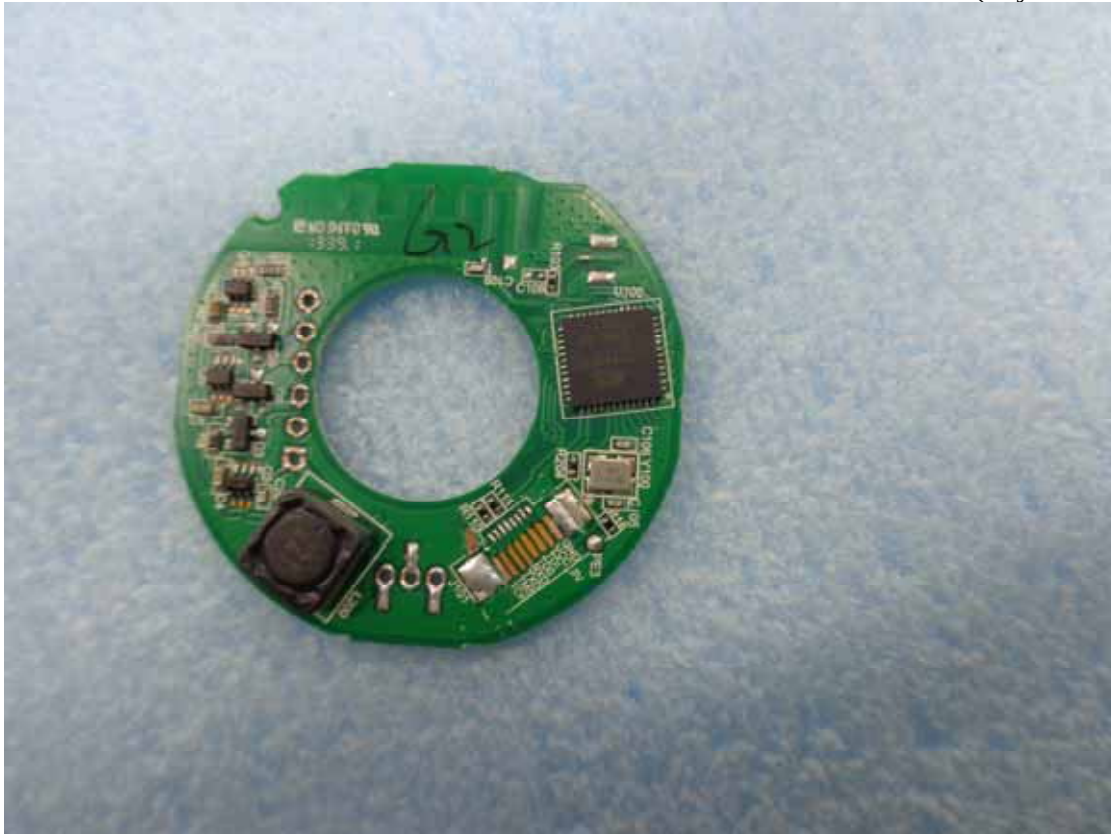
Figure 9 Wireless Board (Crystal Oscillator)
