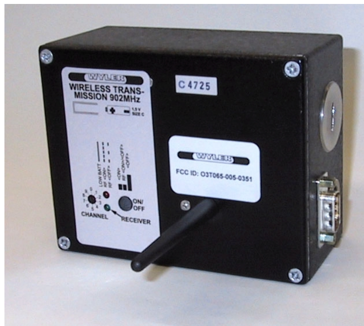
Radio Box with integrated Radio Transmission Module labeled with FCC ID
