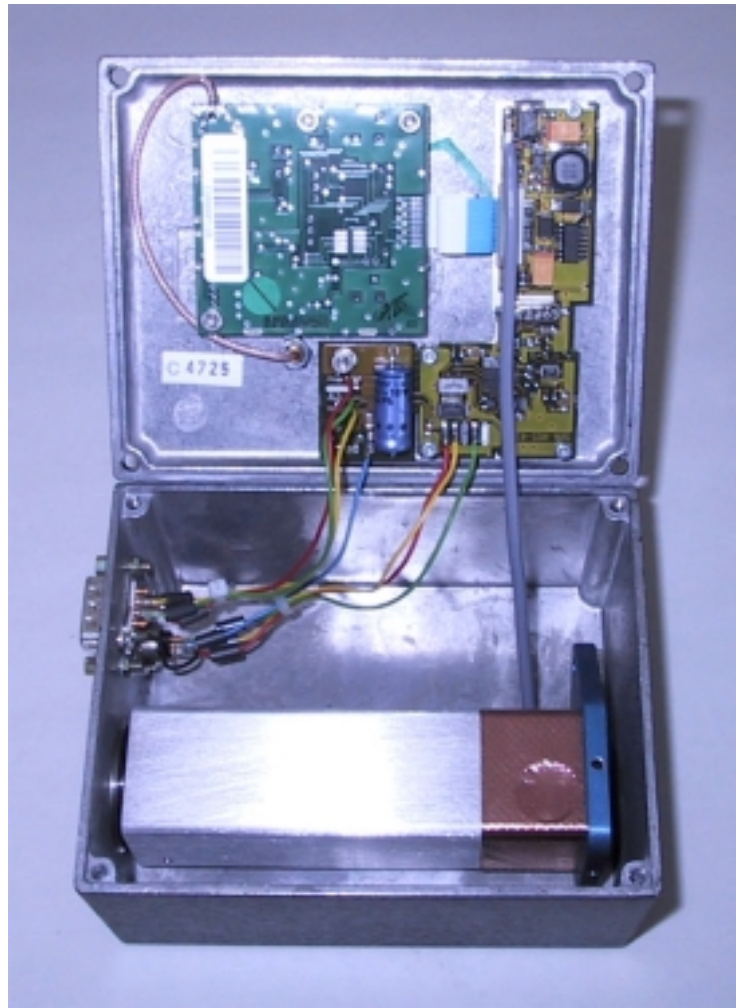
Opened Radio Box with integrated Radio Transmission Module
