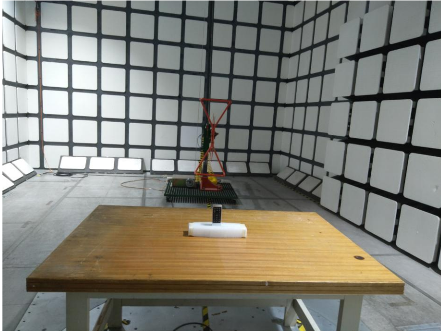
Radiated Emissions View (Below 1 GHz)
