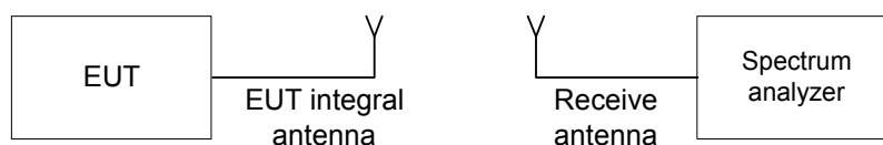
Figure 7.1.1 Setup for transmitter shut down test
