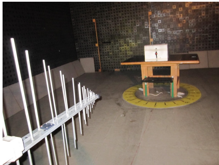
Photograph 8.1.1 Setup for radiated emission measurements
