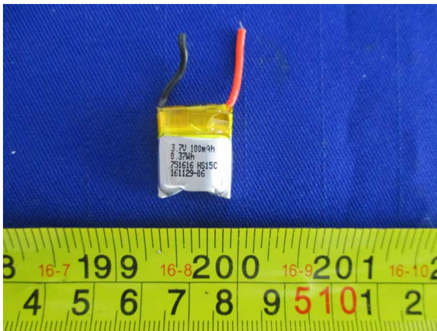
EUT – Battery Top View
