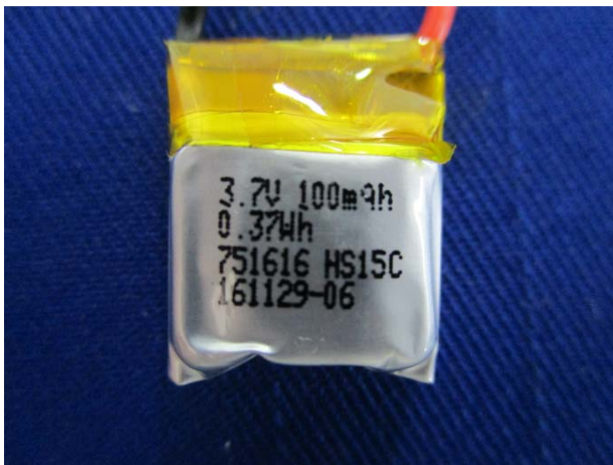
EUT – Battery Label View
