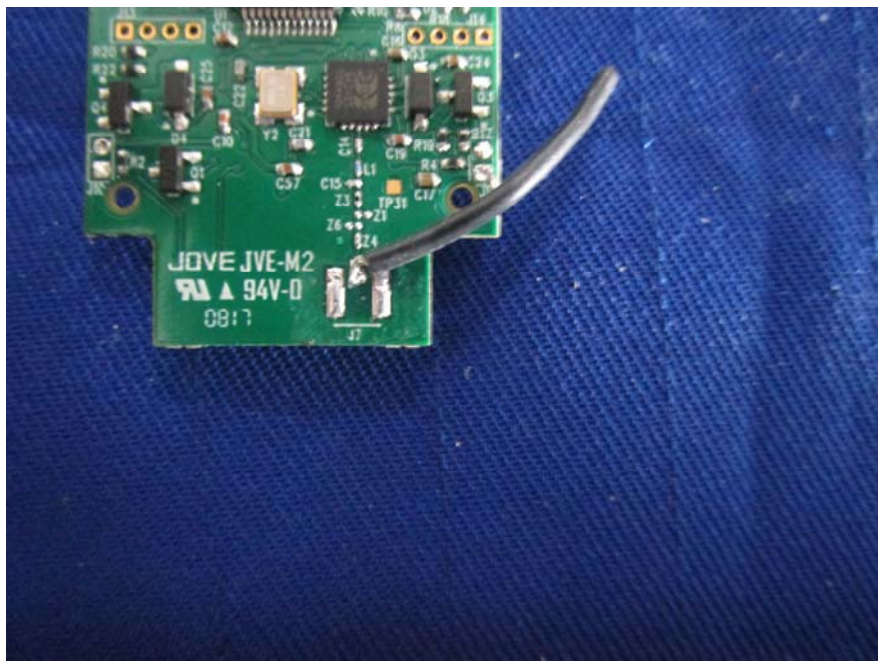
EUT – FHSS Antenna View
