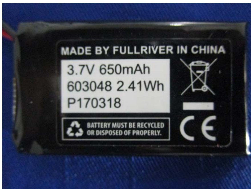
EUT – Battery Label View
