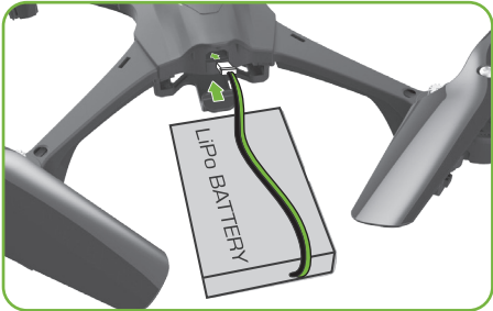
Insert fully charged LiPo battery into the underside of drone, then connect the battery to back of the drone. [See reverse.]
