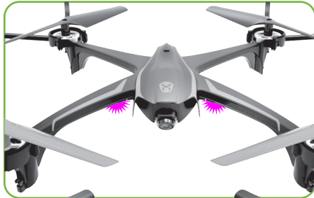
Remove plastic film from lens before use. Once lights turn solid, drone is ready to fly.
