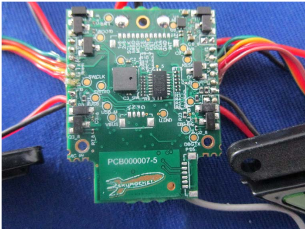
EUT – Main Board Bottom View
