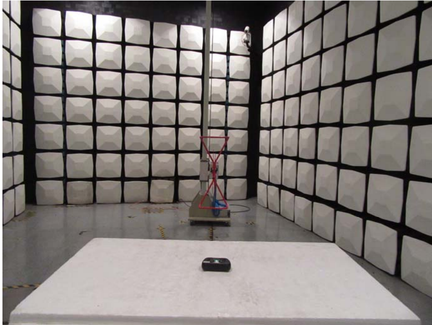
Radiated Emission Below 1GHz View
