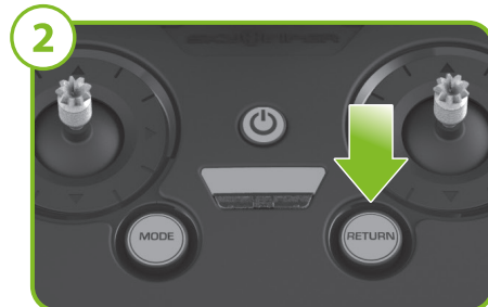
When flying in INDOOR mode, the RETURN button will cause the drone to LAND at its current location.
