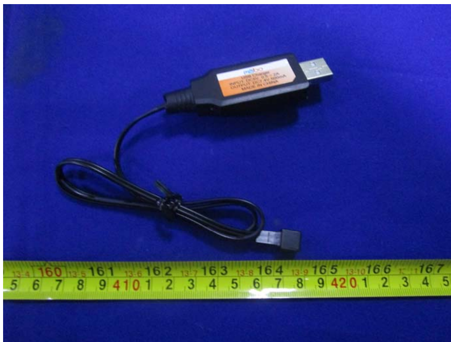
EUT – Charger Cable View
