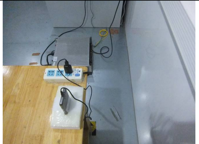
Conducted Emissions Test Setup Side View
