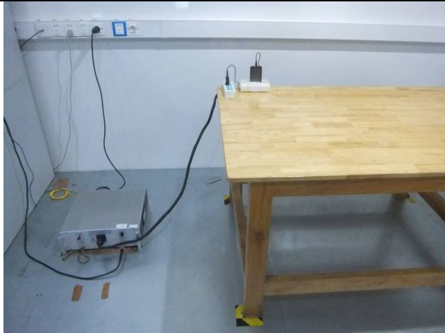
Conducted Emissions Test Setup Front View
