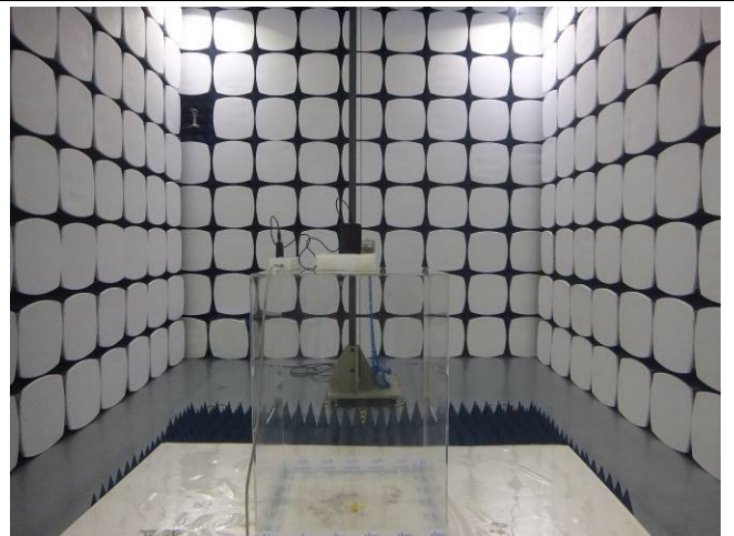
Radiated Spurious Emissions Test Setup Above 1GHz
