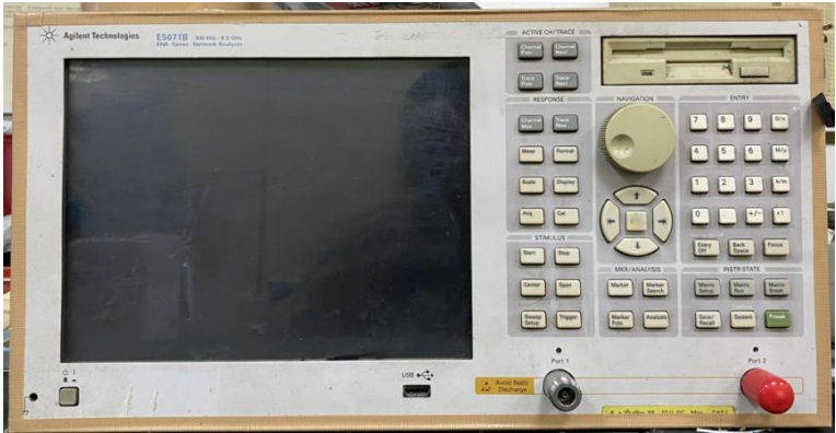
Agilent 5071B (S Parameter (RL/VSWR) Test Equipment)
