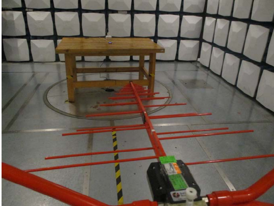
Radiated Emission View (Below 1GHz)
