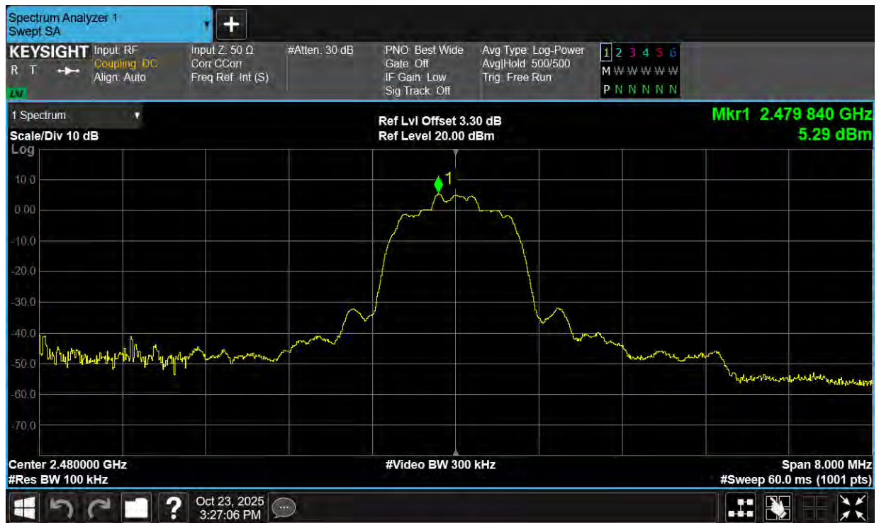
Band Edge NVNT 3-DH1 2480MHz Ant1 No-Hopping Emission
