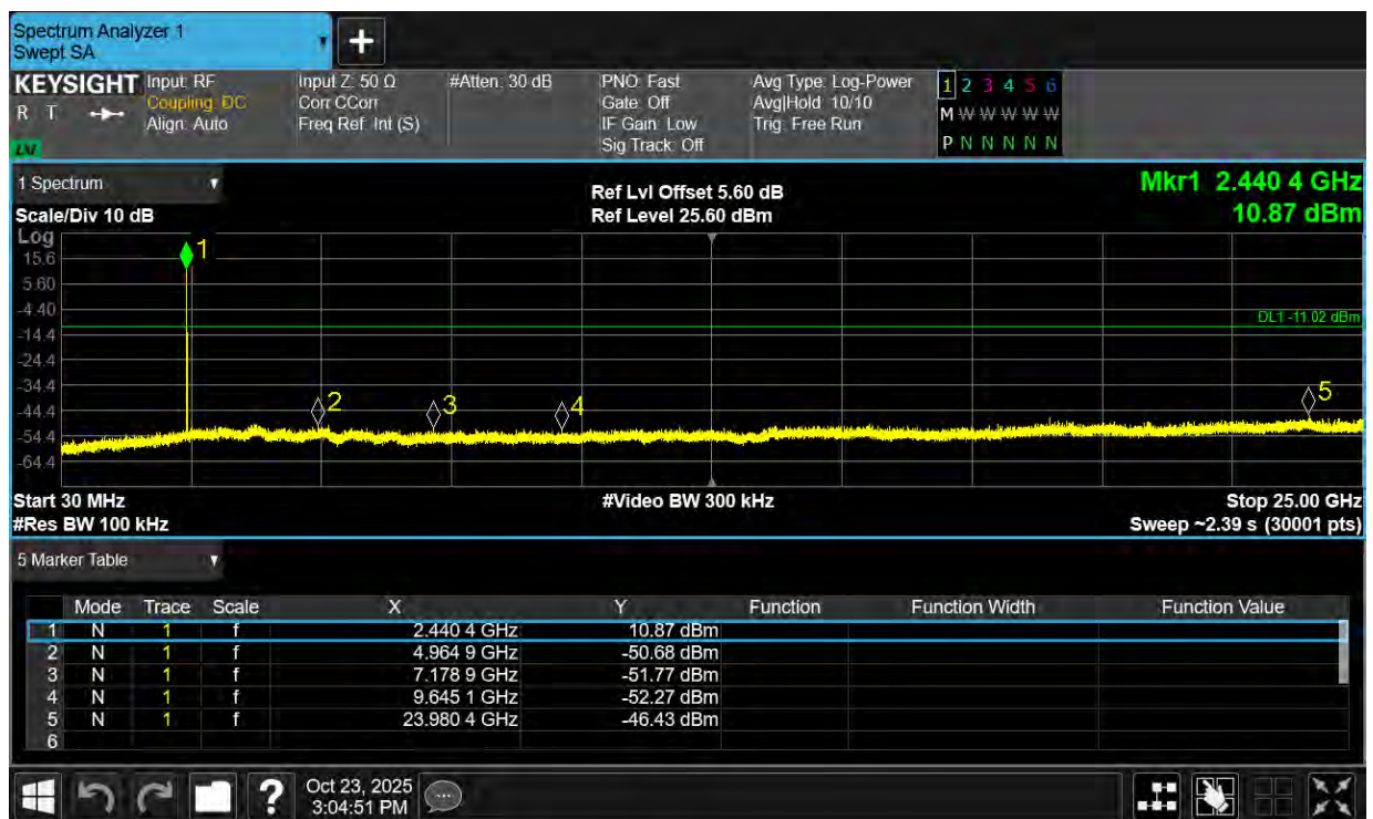
Tx. Spurious NVNT 2-DH1 2480MHz Ant1 Ref
