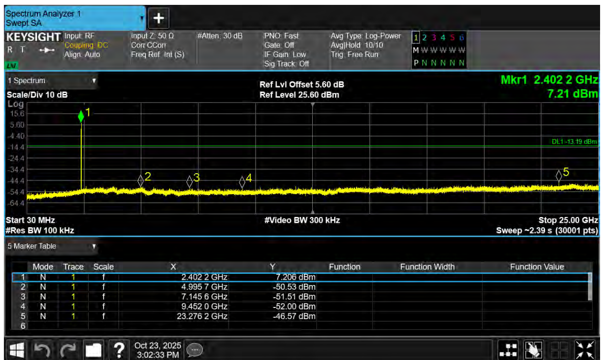
Tx. Spurious NVNT 2-DH1 2441MHz Ant1 Ref
