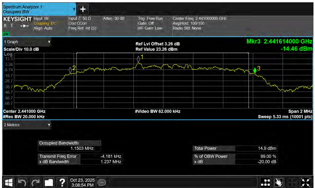
-20dB Bandwidth NVNT 2-DH1 2480MHz Ant1
