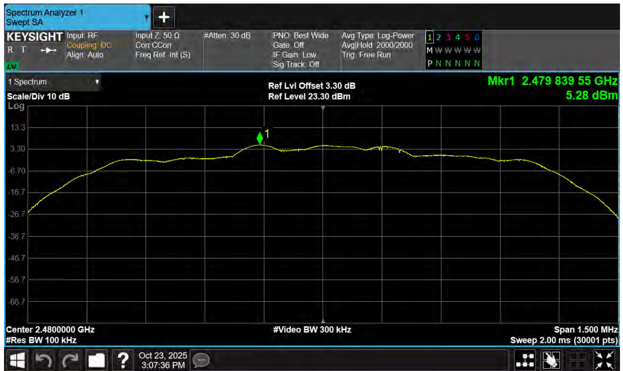
Tx. Spurious NVNT 2-DH1 2480MHz Ant1 Emission
