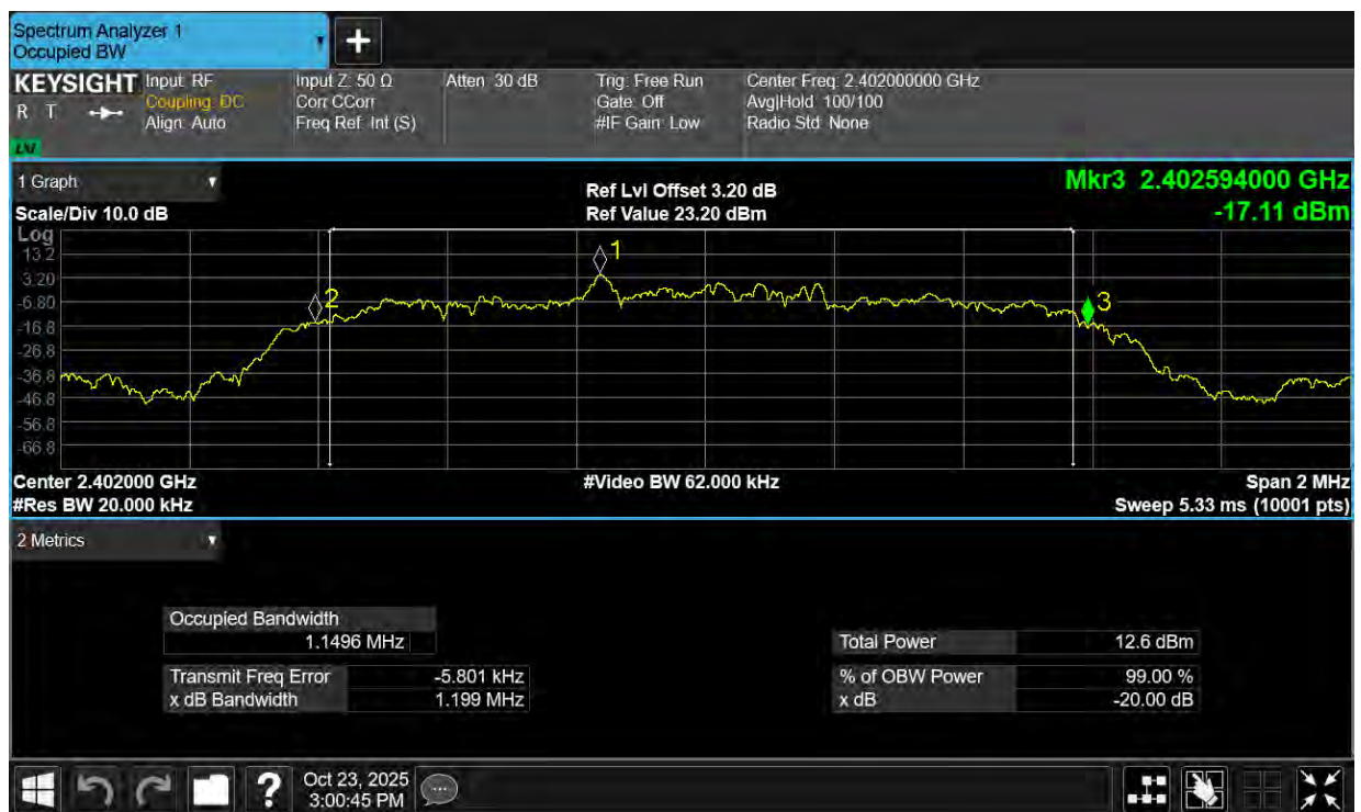
-20dB Bandwidth NVNT 2-DH1 2441MHz Ant1
