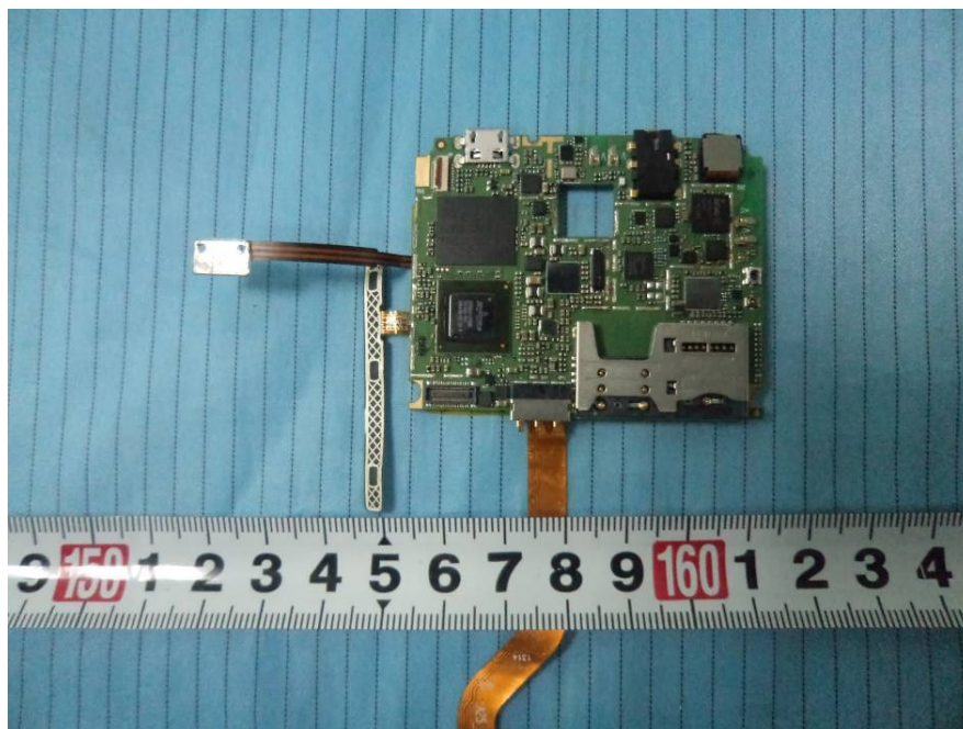
EUT – Main Board Bottom Shielding Off View
