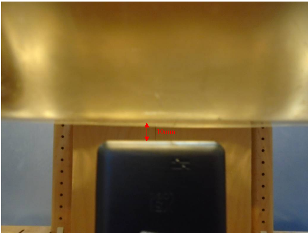
Body-worn Bottom Setup Photo (10mm)
