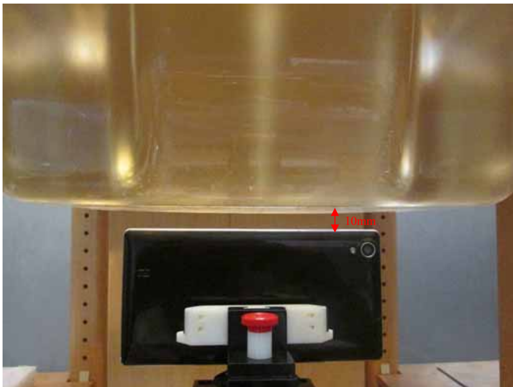
Body-worn Right Setup Photo (10mm)
