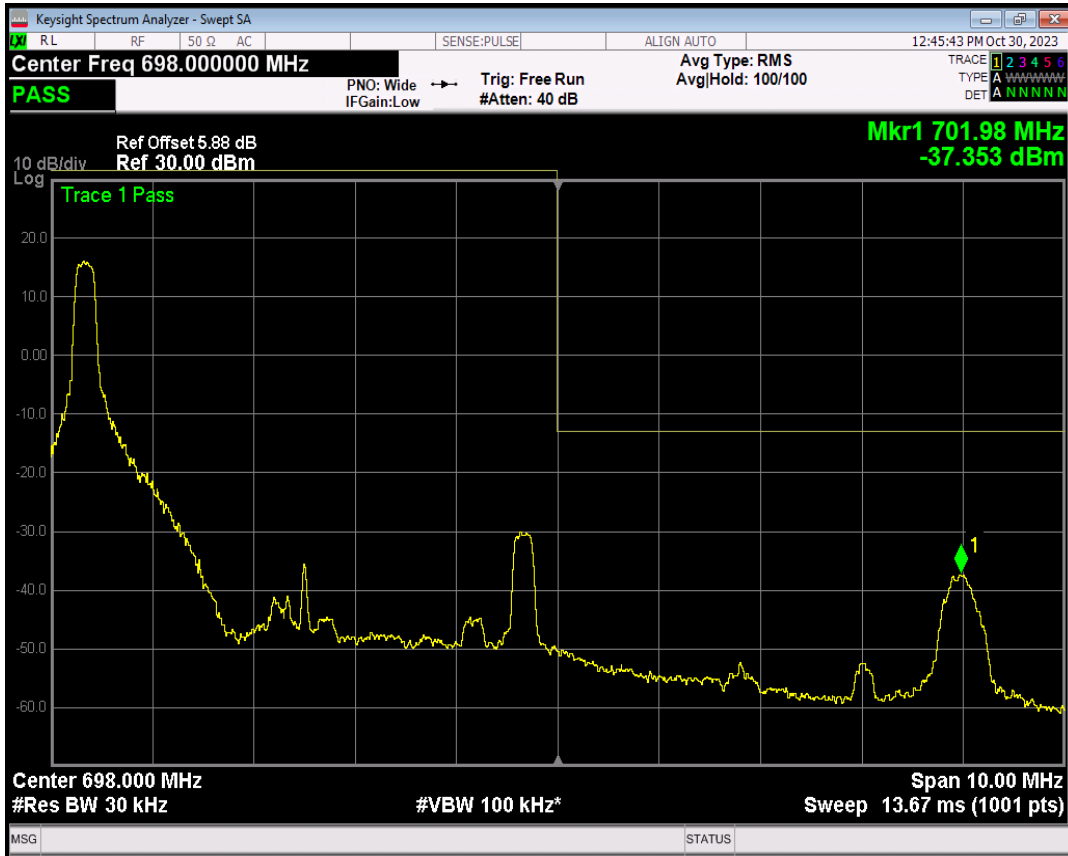
Band71 QPSK BW=5MHz Channel=133447 RB Size=1 Position=#Max
