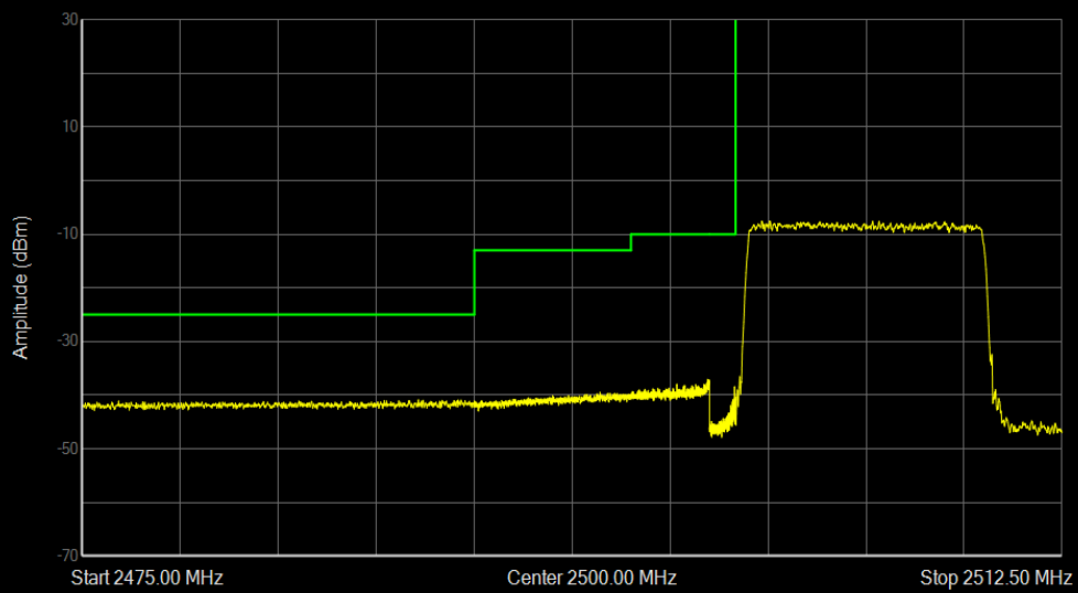
Band7 16QAM BW=10MHz Channel=20800 RB Size=50 Position=#0
