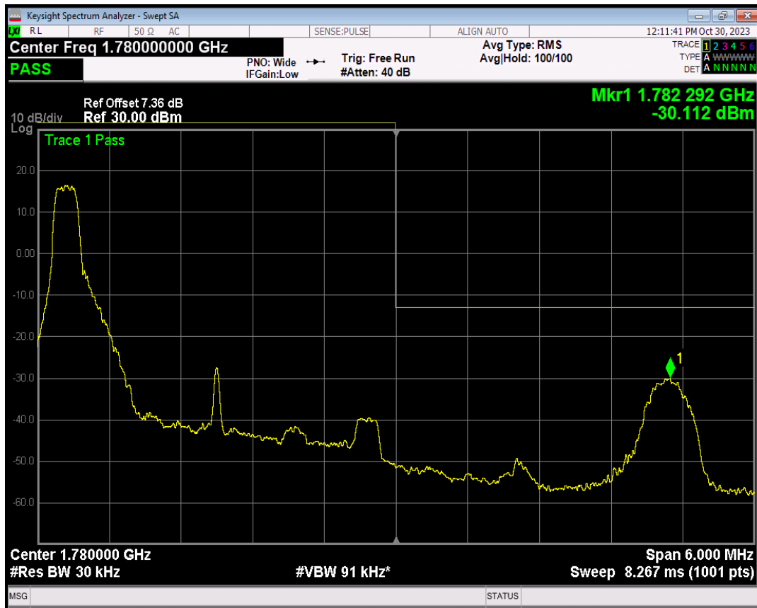
Band66 QPSK BW=3MHz Channel=132657 RB Size=1 Position=#Max
