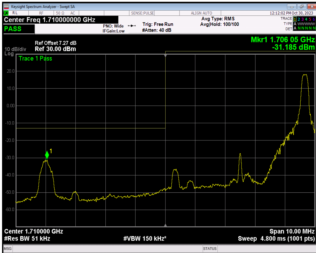
Band66 QPSK BW=5MHz Channel=131997 RB Size=25 Position=#0
