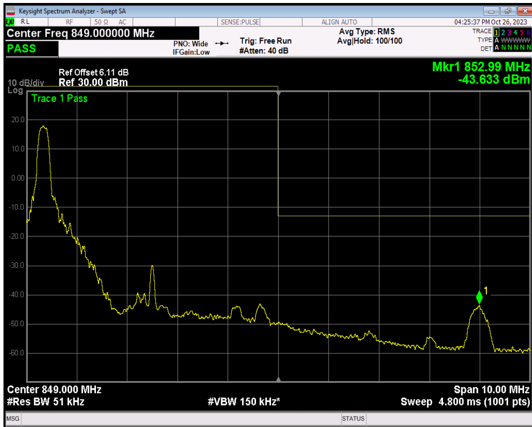
Band5 QPSK BW=5MHz Channel=20625 RB Size=1 Position=#Max
