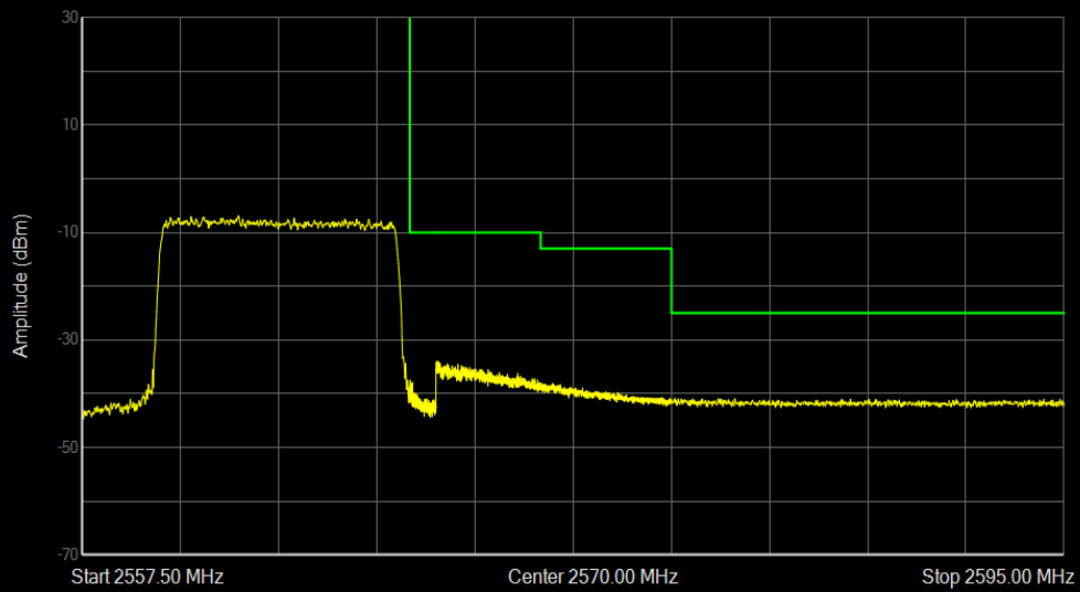
Band7 16QAM BW=10MHz Channel=21400 RB Size=50 Position=#0
