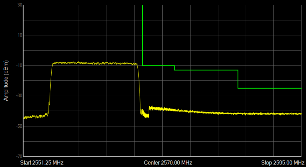
Band7 16QAM BW=15MHz Channel=21375 RB Size=75 Position=#0
