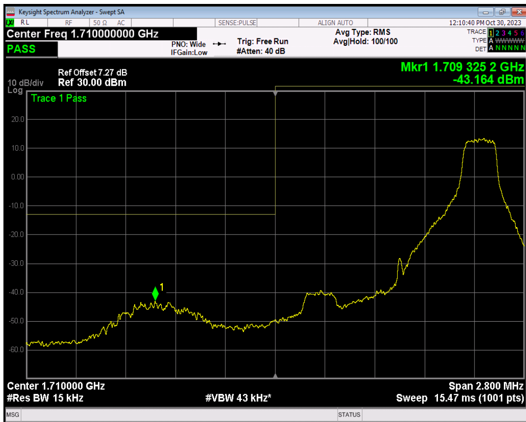
Band66 QPSK BW=1.4MHz Channel=131979 RB Size=6 Position=#0
