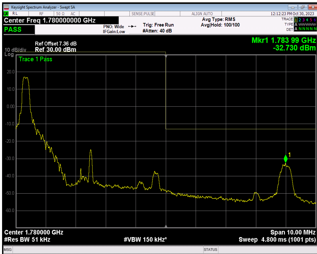
Band66 16QAM BW=5MHz Channel=132647 RB Size=1 Position=#Max
