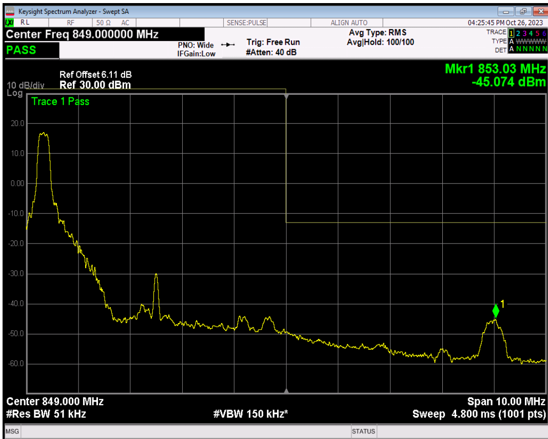
Band5 16QAM BW=5MHz Channel=20625 RB Size=1 Position=#Max
