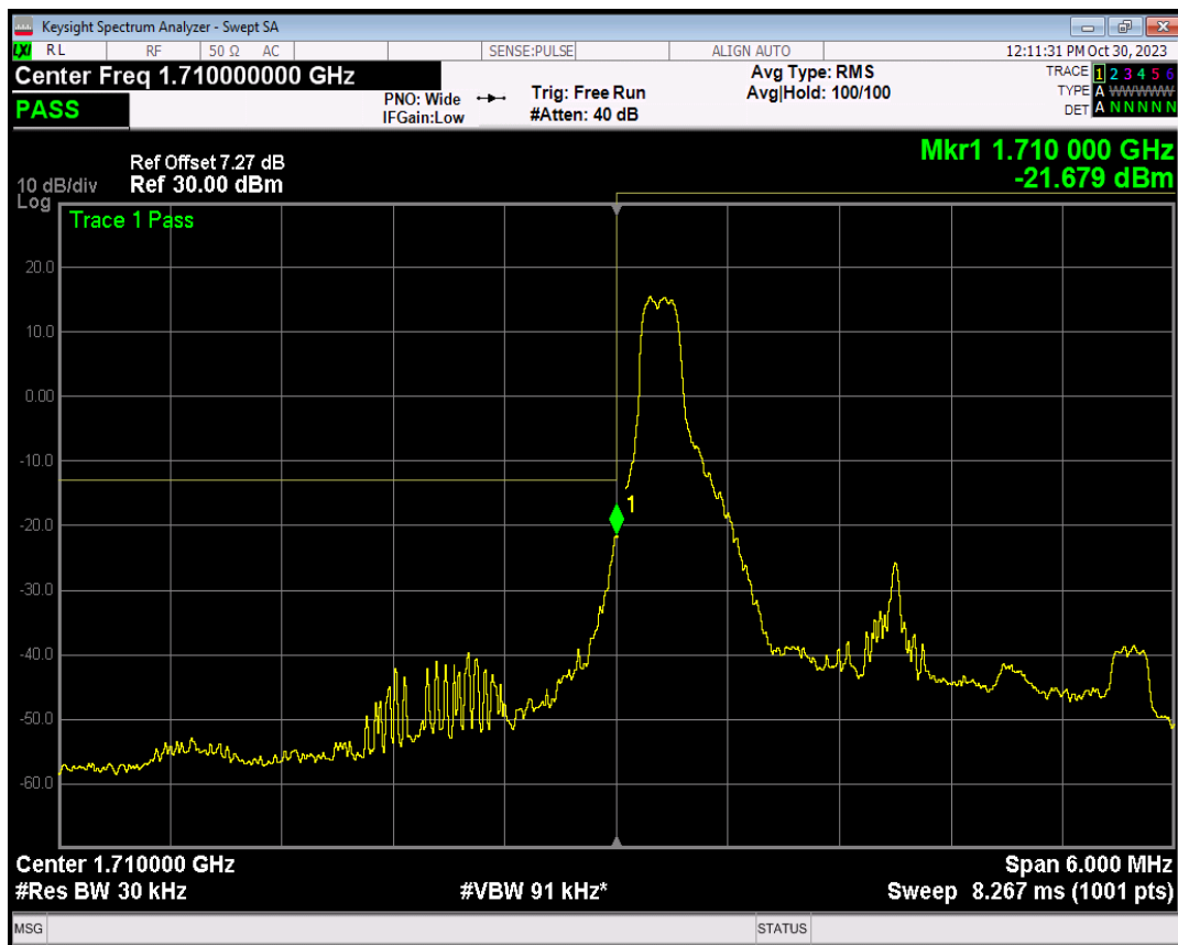
Band66 16QAM BW=3MHz Channel=131987 RB Size=1 Position=#Max
