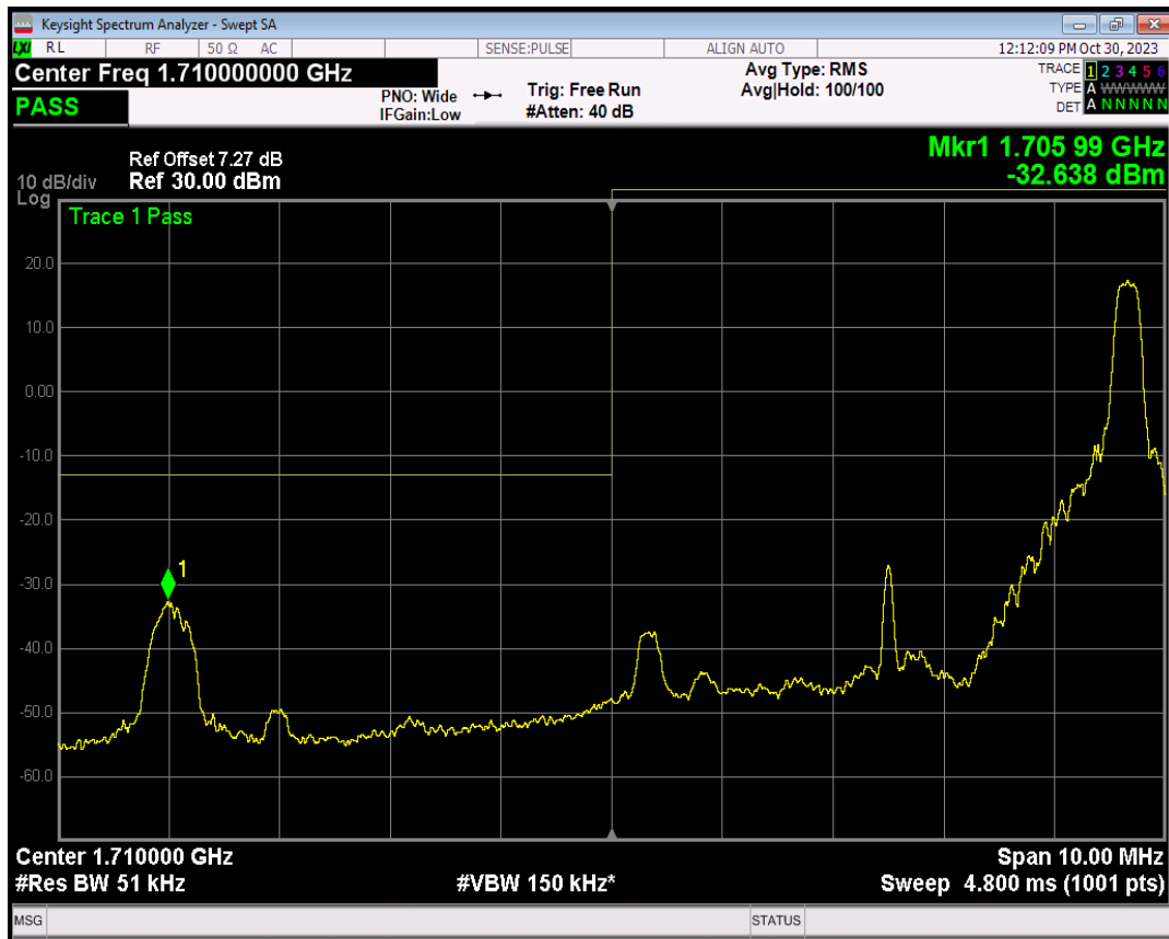
Band66 16QAM BW=5MHz Channel=131997 RB Size=25 Position=#0
