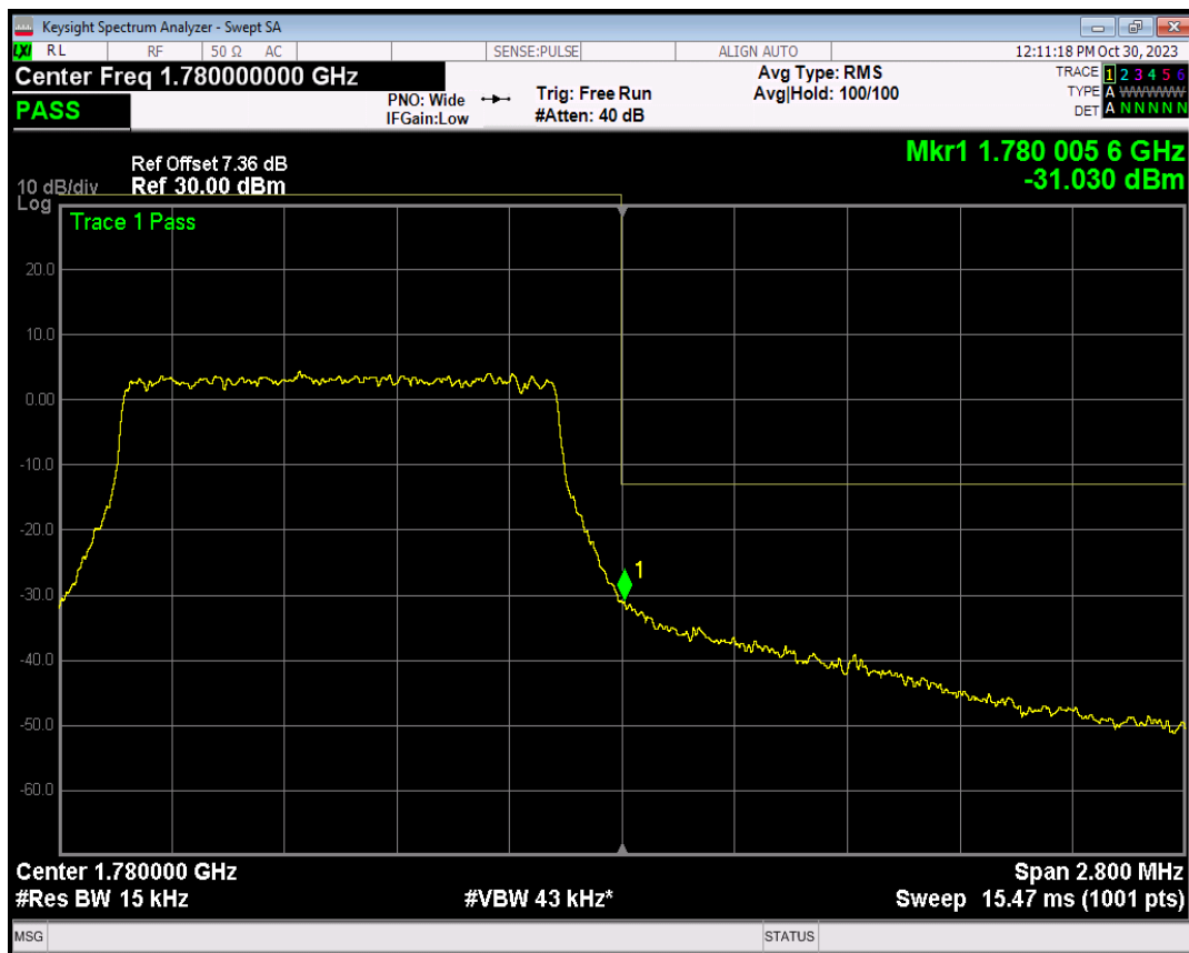
Band66 QPSK BW=3MHz Channel=131987 RB Size=1 Position=#0
