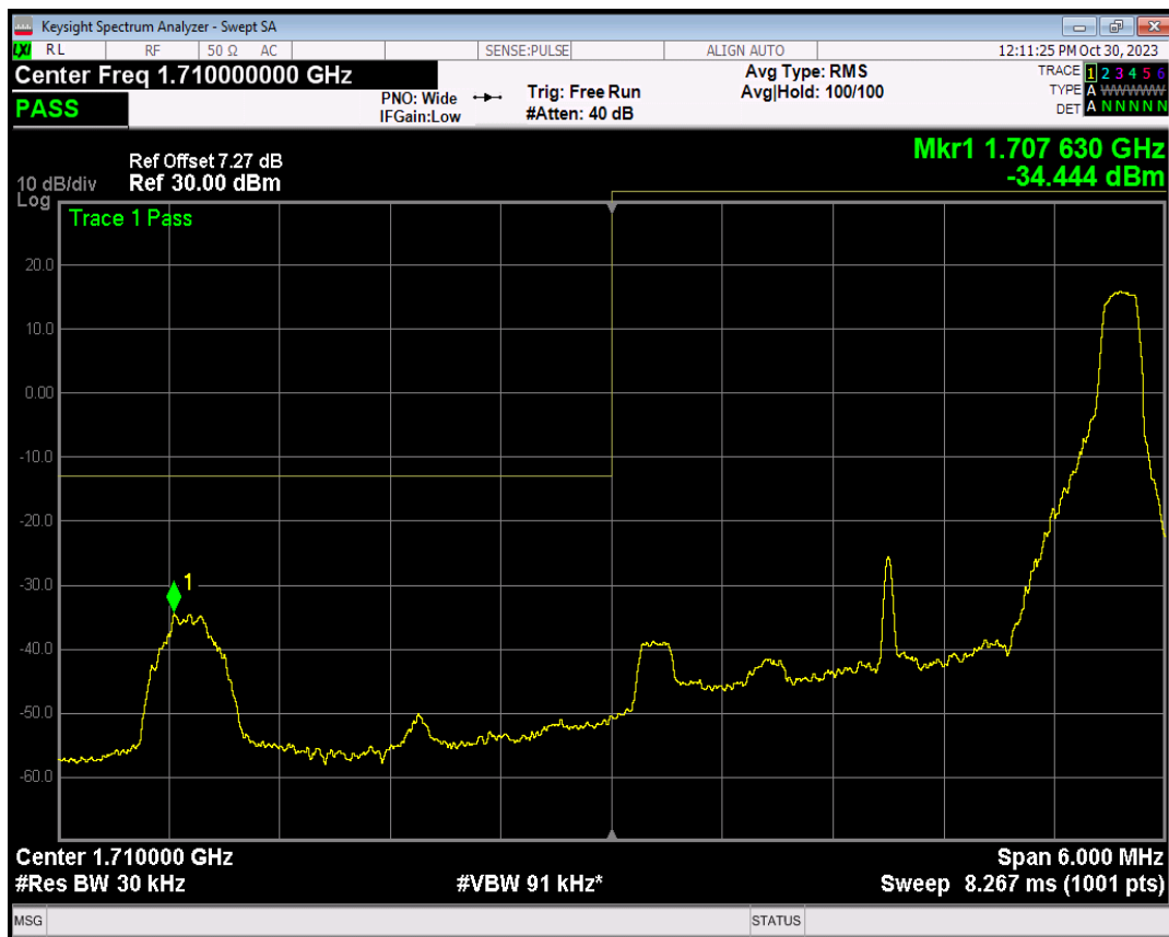
Band66 QPSK BW=3MHz Channel=131987 RB Size=15 Position=#0
