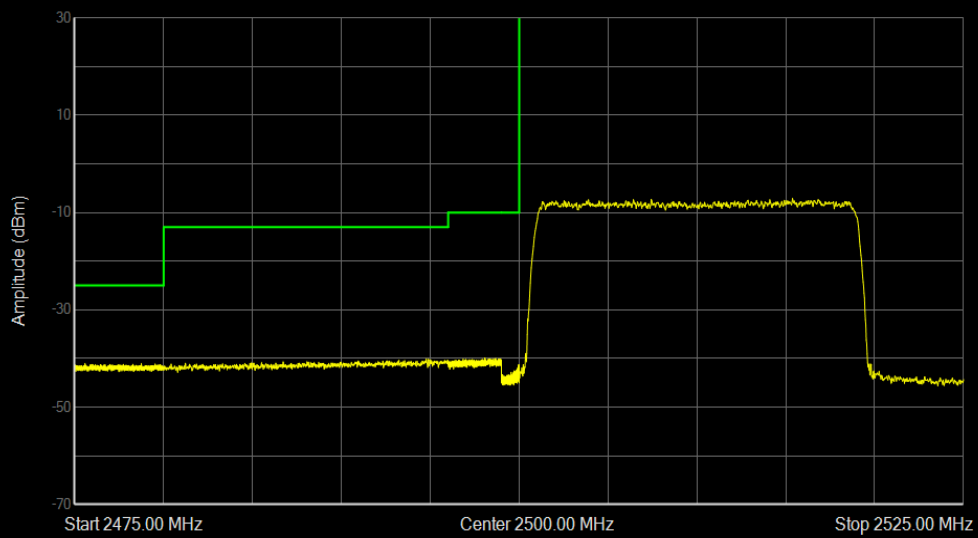
Band7 16QAM BW=20MHz Channel=20850 RB Size=100 Position=#0
