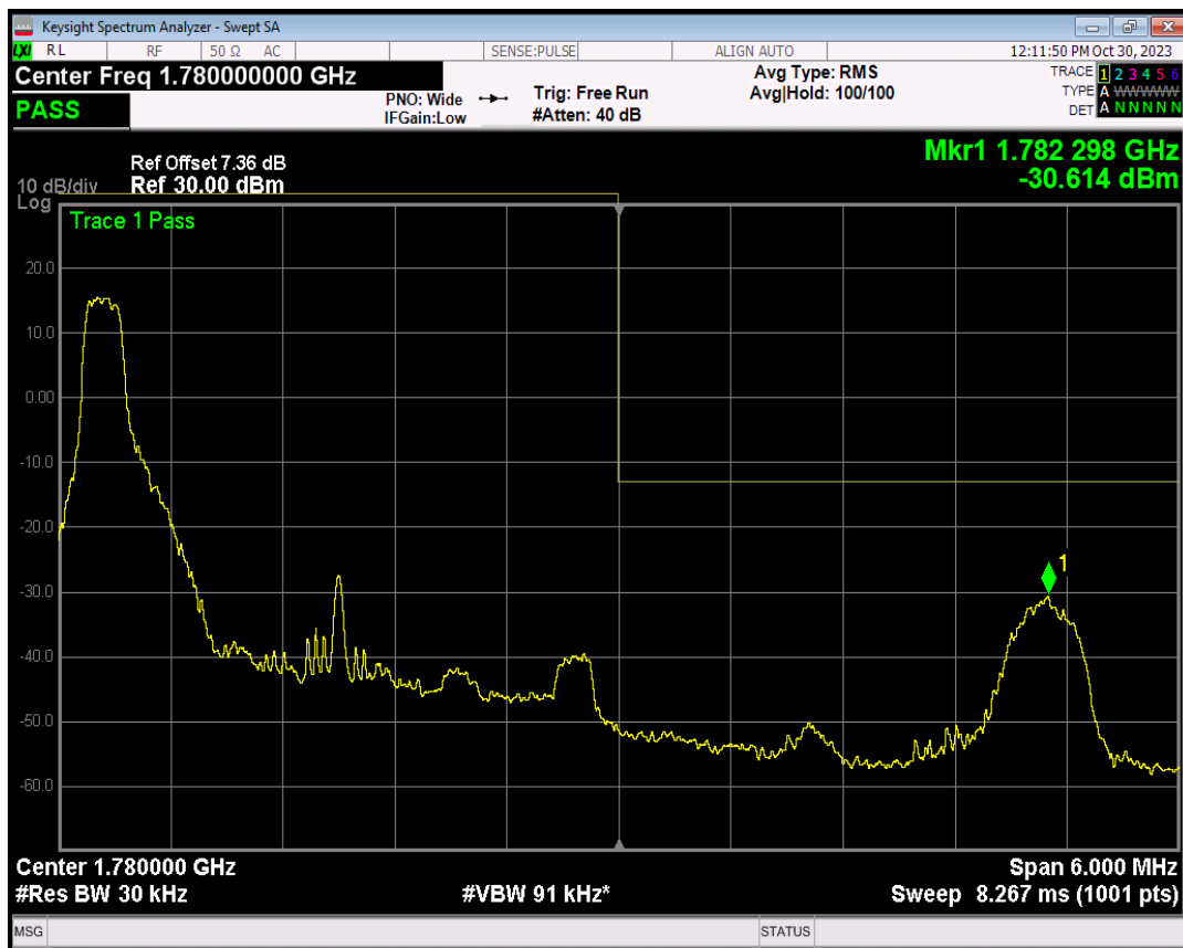
Band66 16QAM BW=3MHz Channel=132657 RB Size=1 Position=#Max
