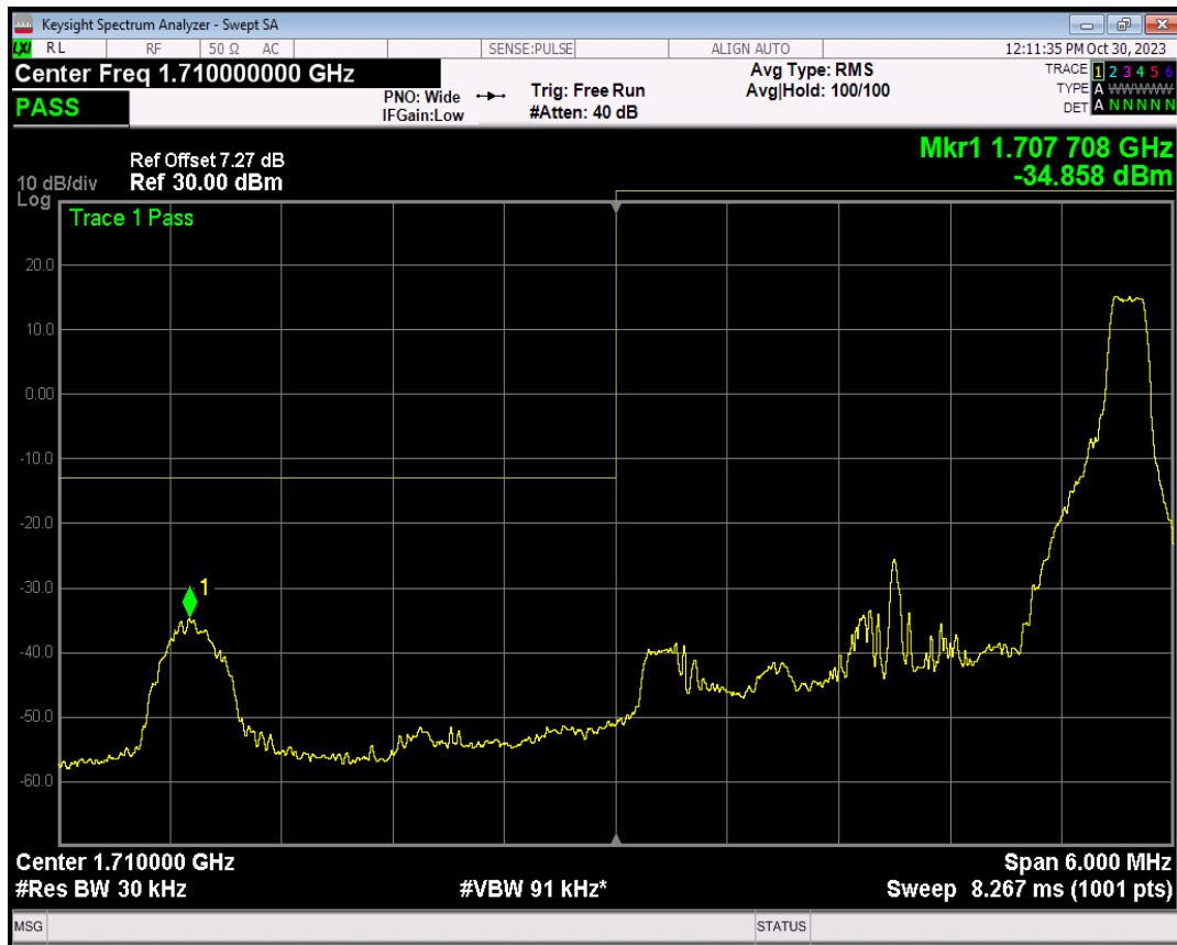
Band66 16QAM BW=3MHz Channel=131987 RB Size=15 Position=#0
