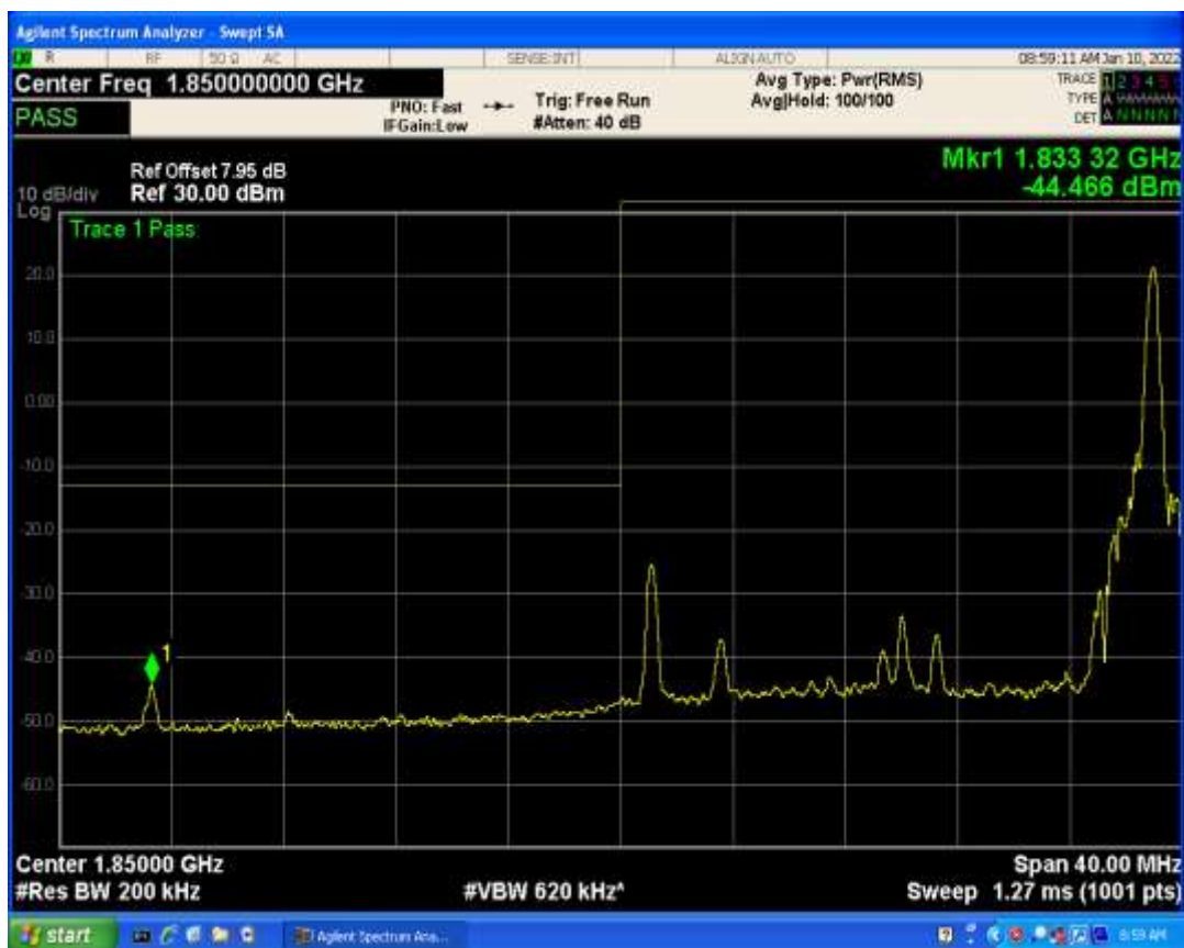
Band2 QPSK BW=20MHz Channel=19100 RB Size=1 Position=#0
