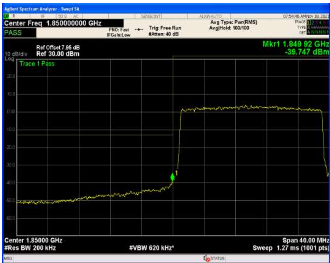
Band25 QPSK BW=15MHz Channel=26615 RB Size=1 Position=#0
