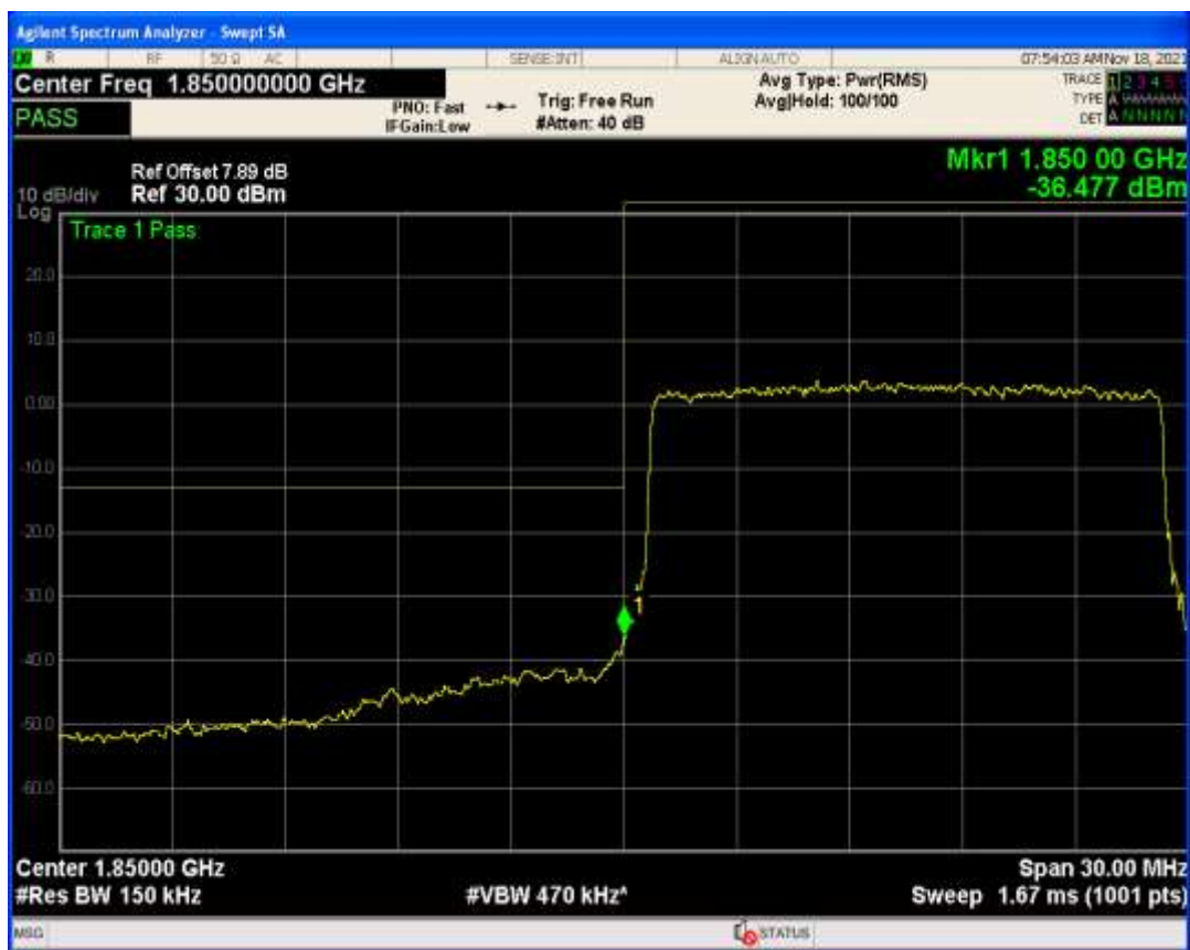
Band25 QPSK BW=15MHz Channel=26115 RB Size=1 Position=#Max
