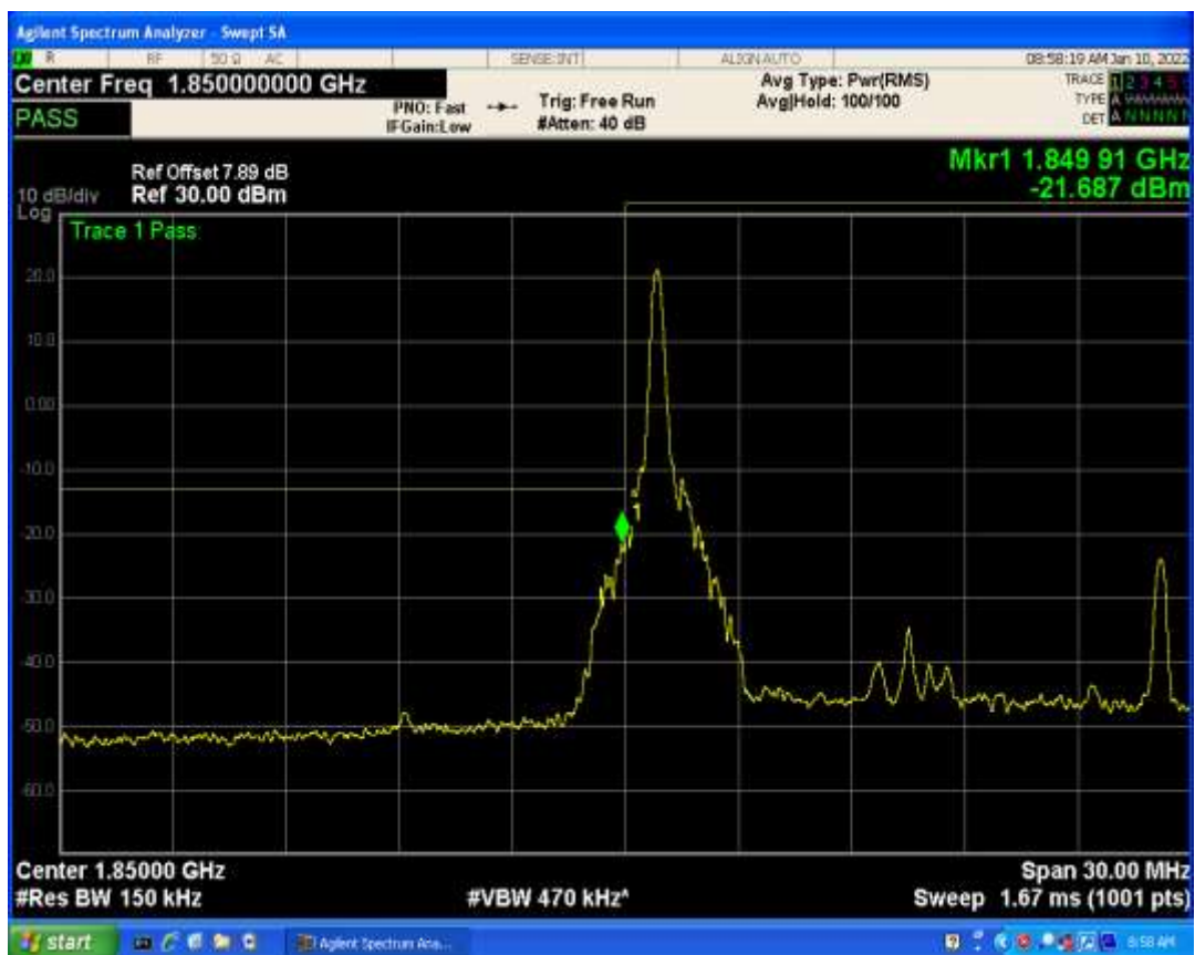
Band2 QPSK BW=3MHz Channel=18615 RB Size=15 Position=#0
