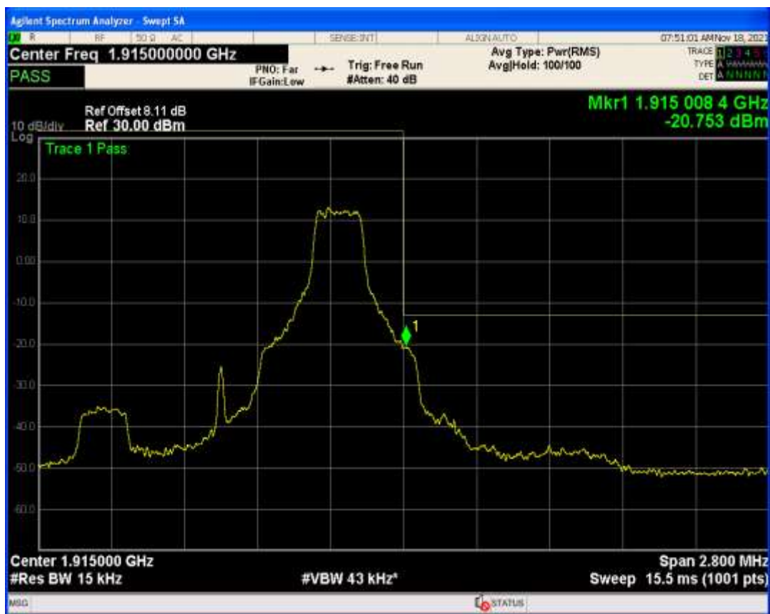
Band25 QPSK BW=1.4MHz Channel=26683 RB Size=1 Position=#0
