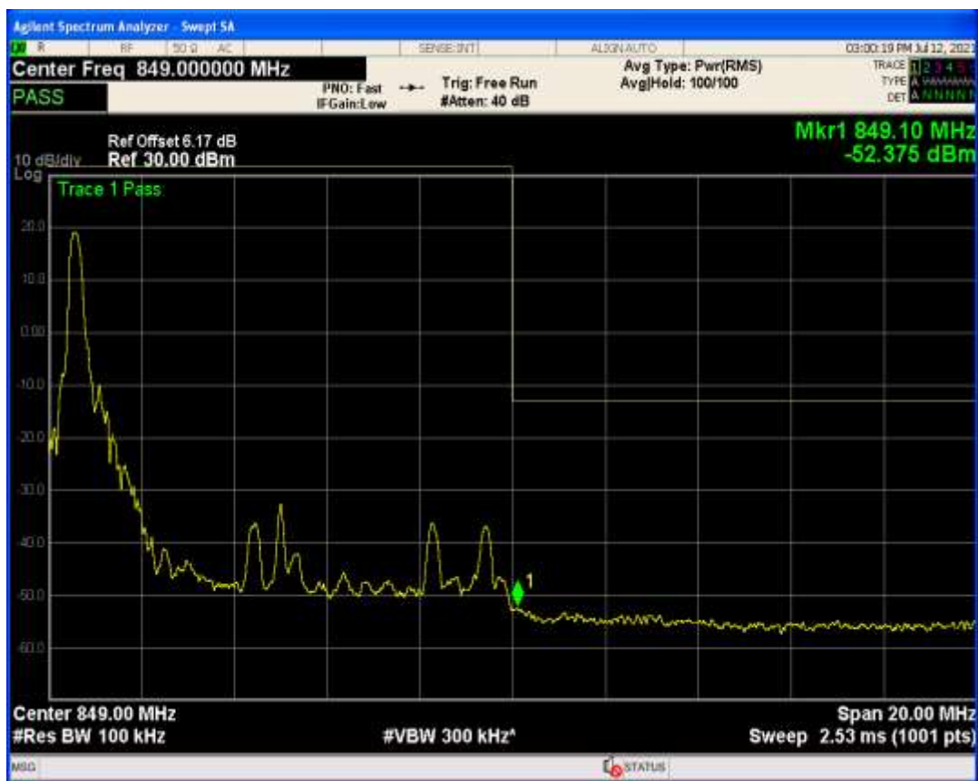
Band26b QAM16 BW=10MHz Channel=26840 RB Size=50 Position=#0
