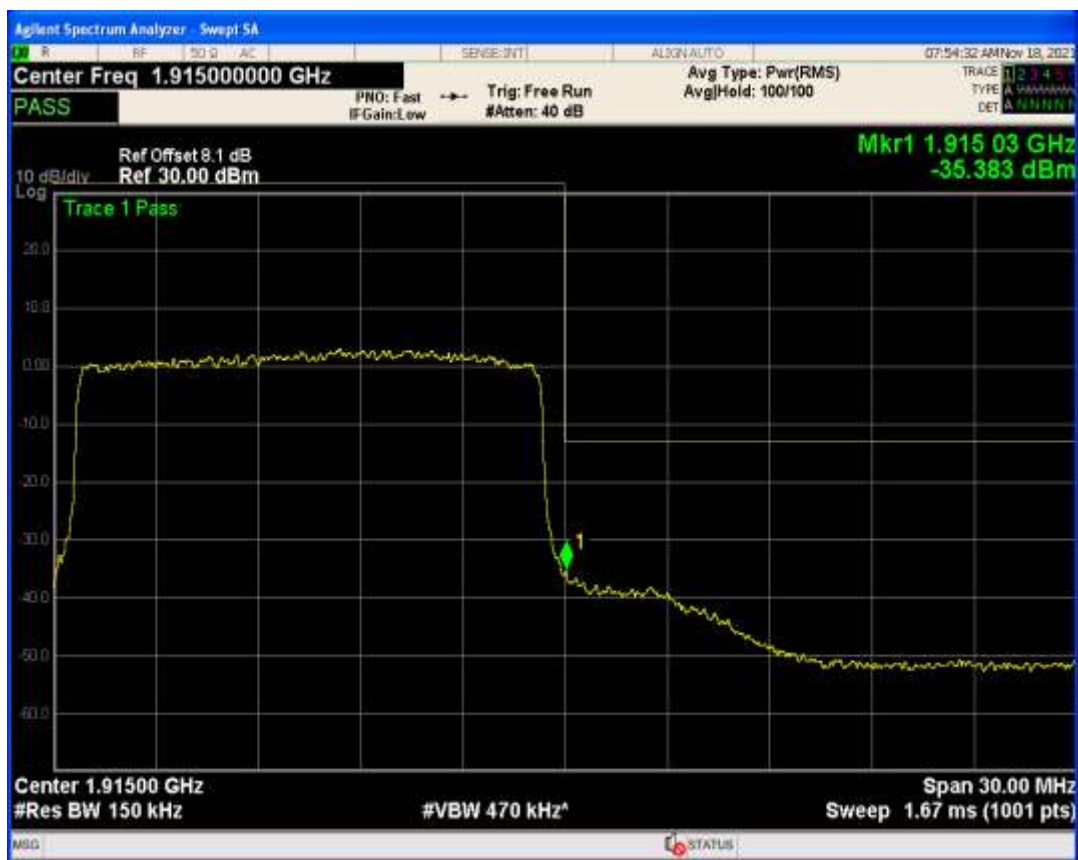
Band25 QAM16 BW=15MHz Channel=26115 RB Size=1 Position=#0
