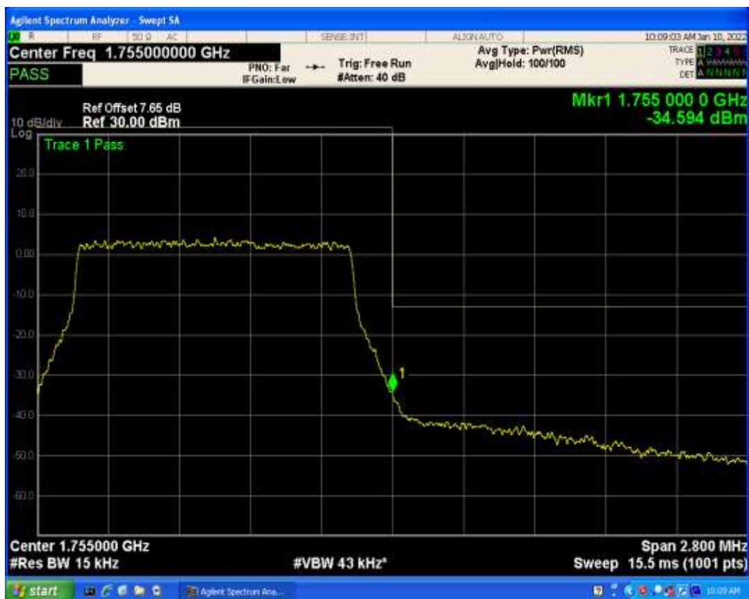
Band4 QAM16 BW=1.4MHz Channel=20393 RB Size=1 Position=#Max
