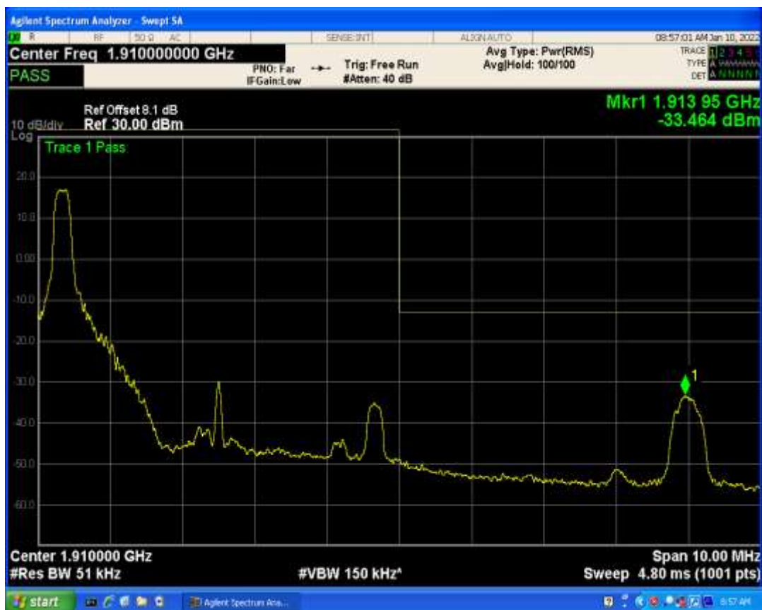
Band2 QPSK BW=5MHz Channel=19175 RB Size=1 Position=#Max
