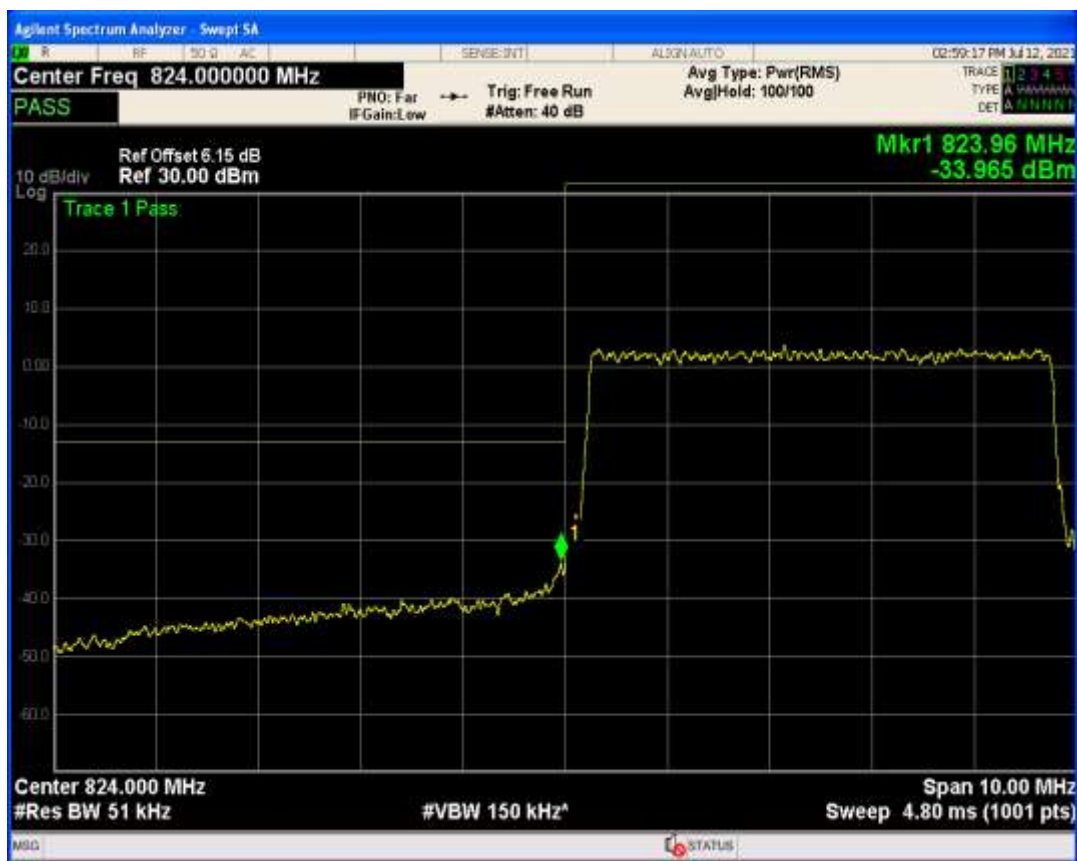
Band26b QAM16 BW=5MHz Channel=26815 RB Size=1 Position=#Max
