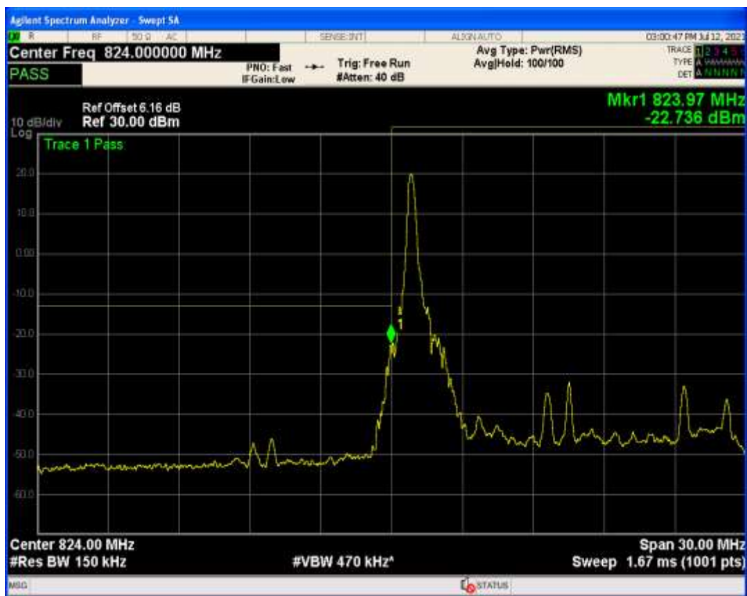
Band26b QAM16 BW=10MHz Channel=26990 RB Size=50 Position=#0
