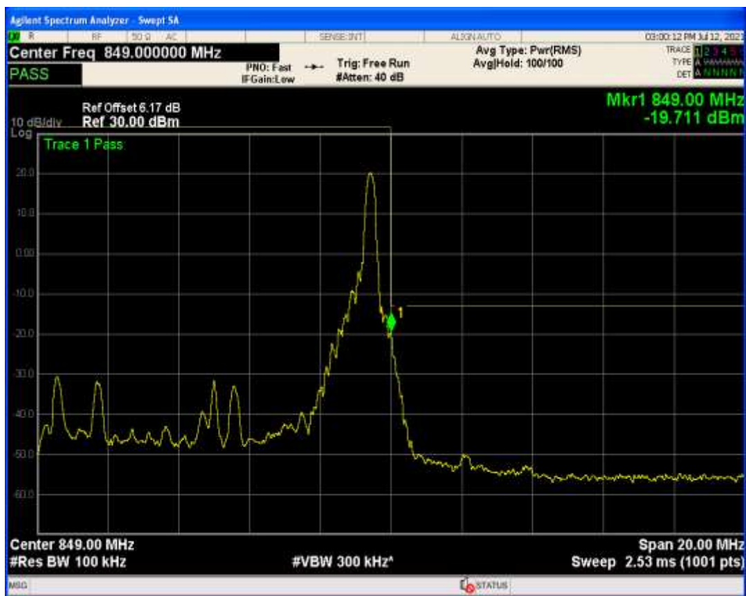
Band26b QPSK BW=10MHz Channel=26990 RB Size=50 Position=#0
