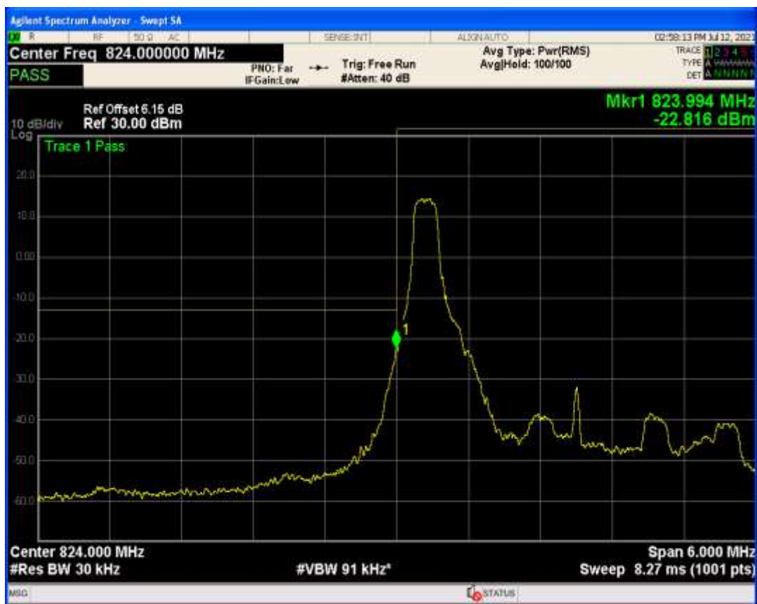
Band26b QAM16 BW=15MHz Channel=26965 RB Size=75 Position=#0
