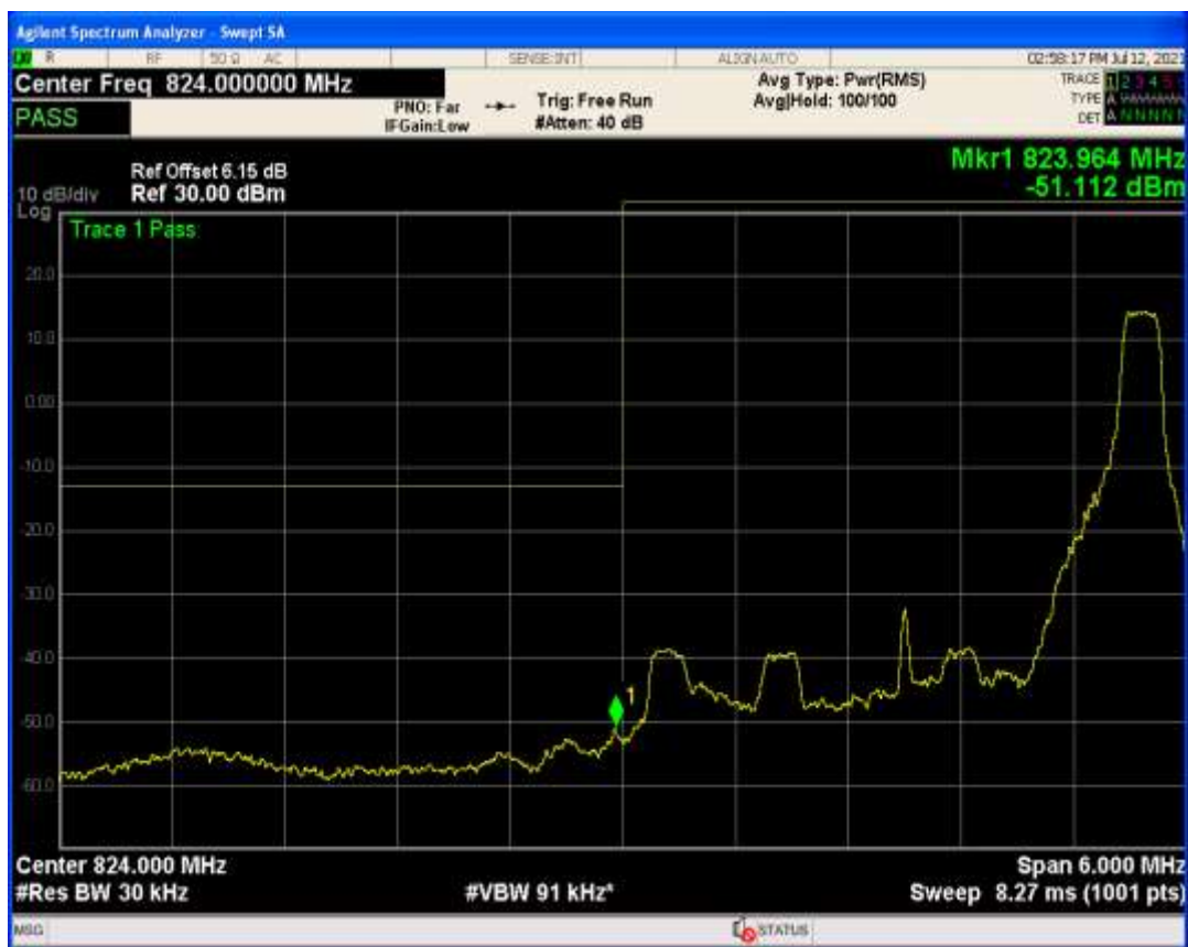
Band26b QAM16 BW=3MHz Channel=26805 RB Size=1 Position=#0
