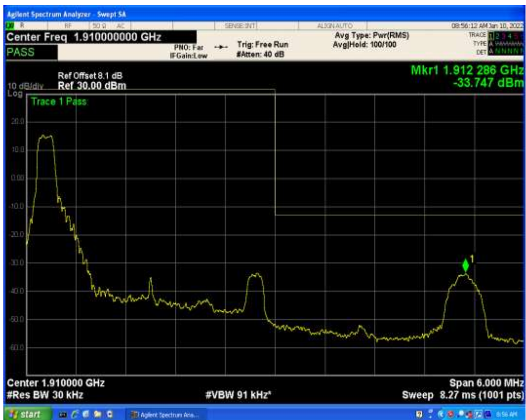
Band2 QPSK BW=3MHz Channel=19185 RB Size=15 Position=#0
