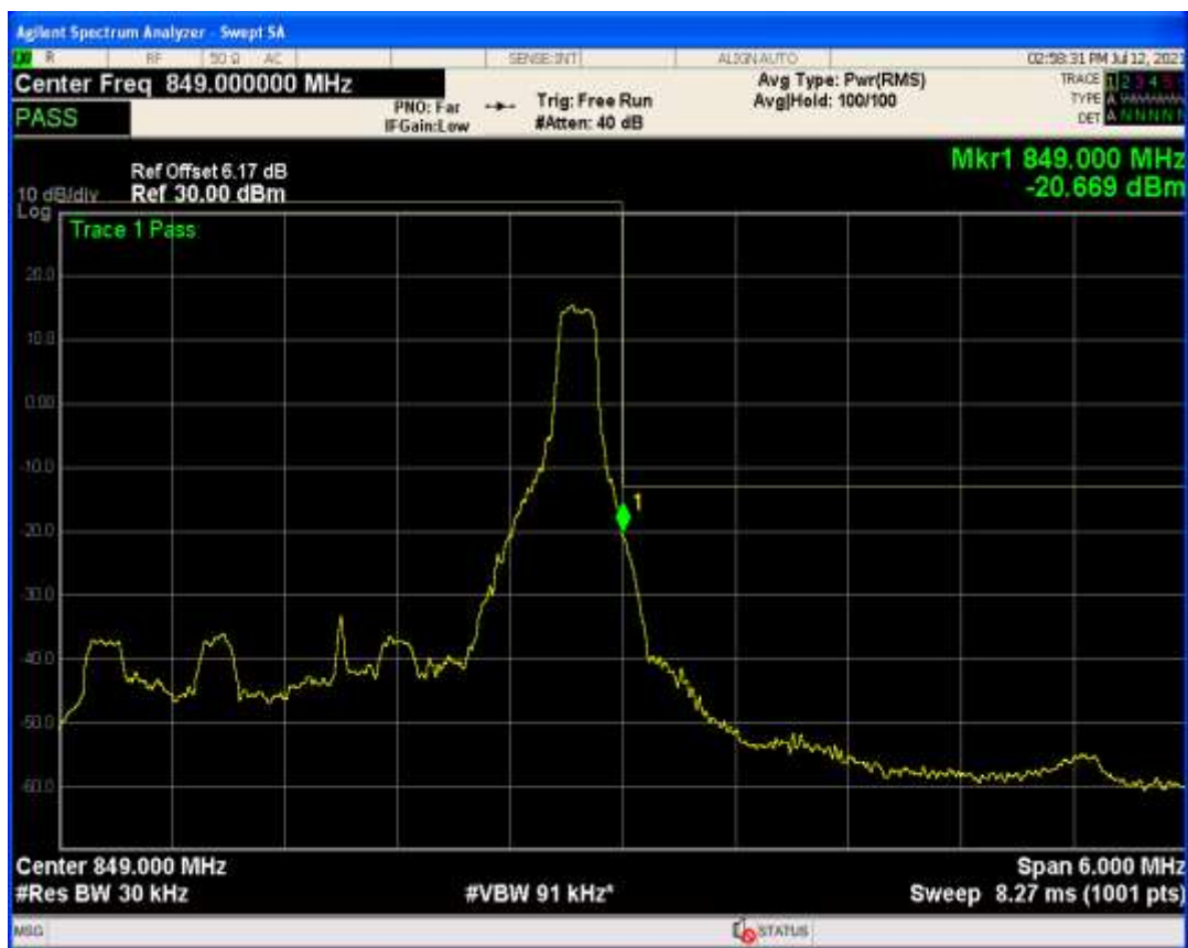
Band26b QPSK BW=3MHz Channel=27025 RB Size=15 Position=#0
