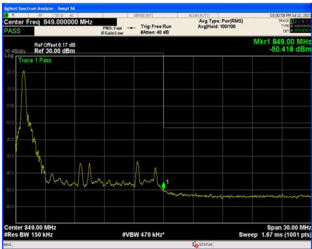
Band26b QPSK BW=3MHz Channel=26805 RB Size=15 Position=#0
