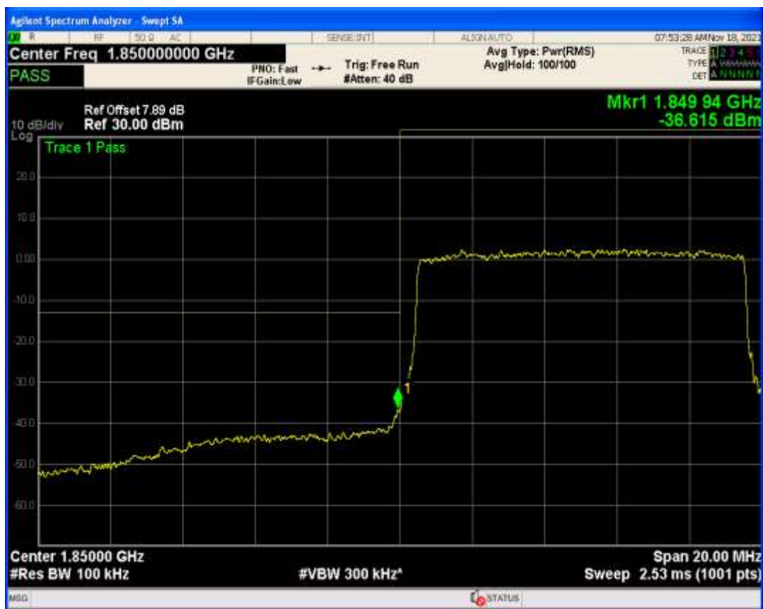
Band25 QAM16 BW=10MHz Channel=26640 RB Size=50 Position=#0
