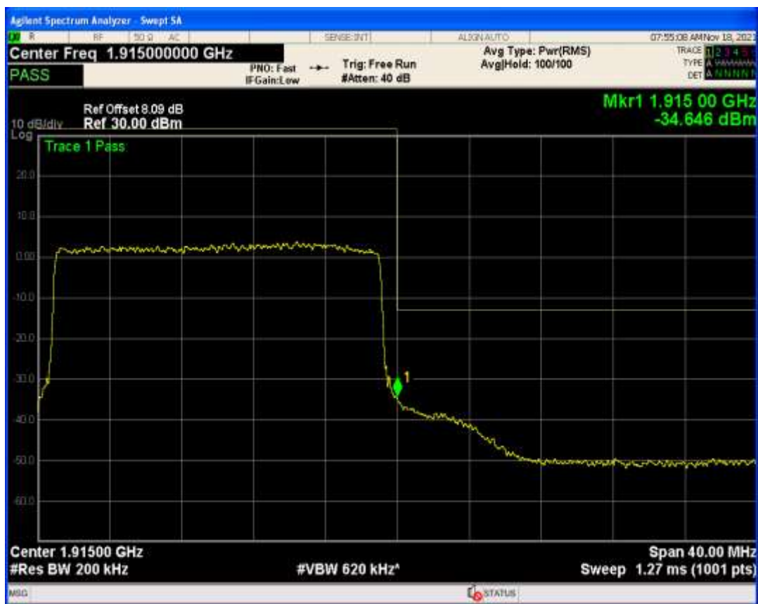
Band25 QPSK BW=20MHz Channel=26590 RB Size=1 Position=#Max
