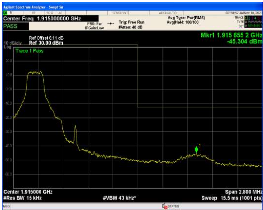
Band25 QPSK BW=20MHz Channel=26590 RB Size=100 Position=#0
