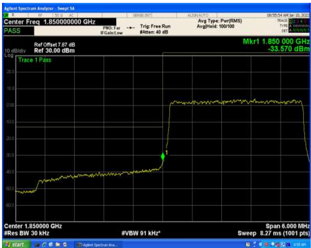
Band2 QPSK BW=3MHz Channel=18615 RB Size=1 Position=#Max
