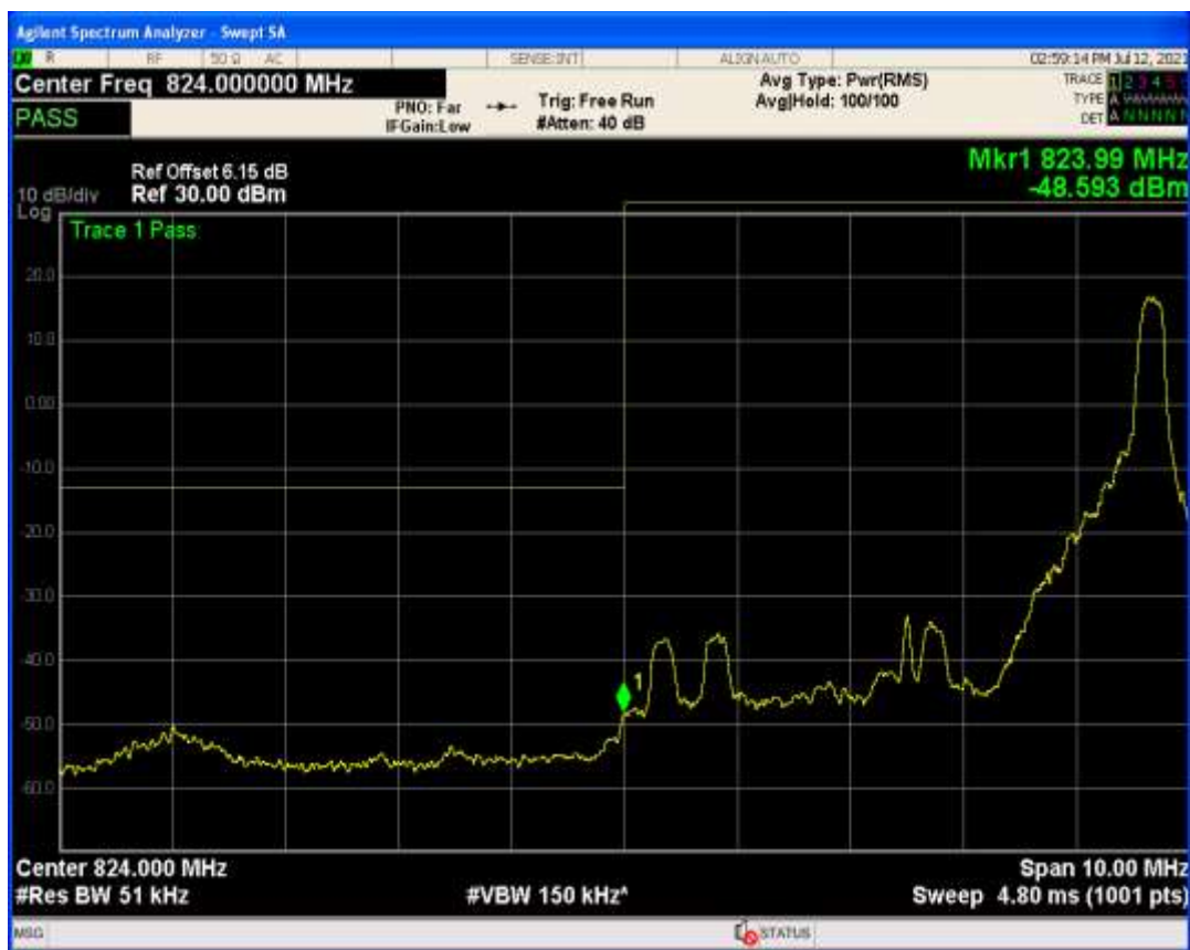
Band26b QAM16 BW=3MHz Channel=26805 RB Size=15 Position=#0
