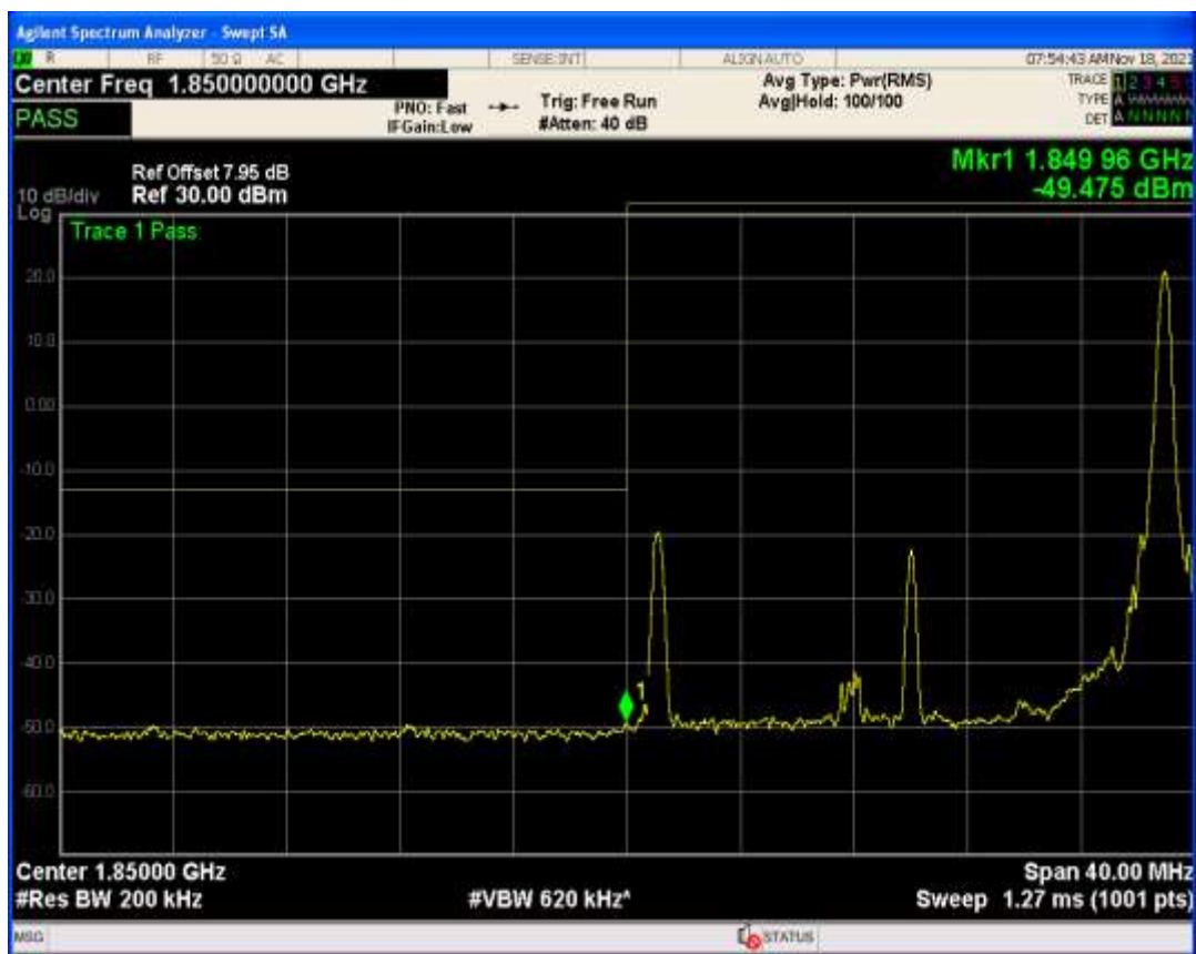
Band25 QPSK BW=20MHz Channel=26140 RB Size=1 Position=#0
