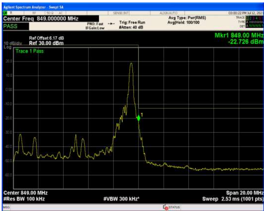
Band26b QAM16 BW=10MHz Channel=26840 RB Size=1 Position=#0
