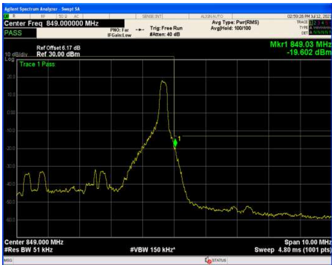
Band26b QPSK BW=5MHz Channel=27015 RB Size=25 Position=#0
