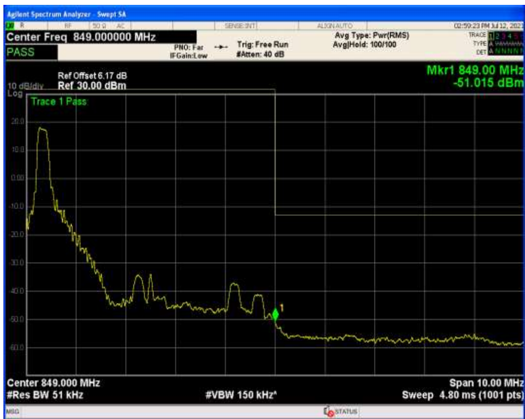
Band26b QPSK BW=15MHz Channel=26965 RB Size=1 Position=#Max
