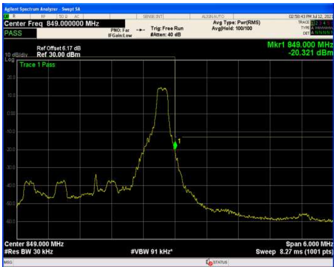
Band26b QAM16 BW=3MHz Channel=27025 RB Size=1 Position=#0
