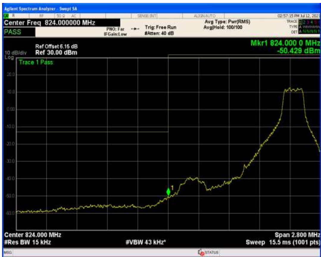
Band26b QAM16 BW=1.4MHz Channel=26797 RB Size=1 Position=#0
