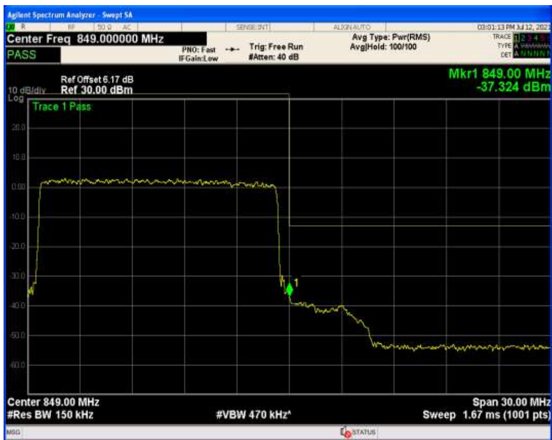
Band26b QPSK BW=10MHz Channel=26840 RB Size=50 Position=#0
