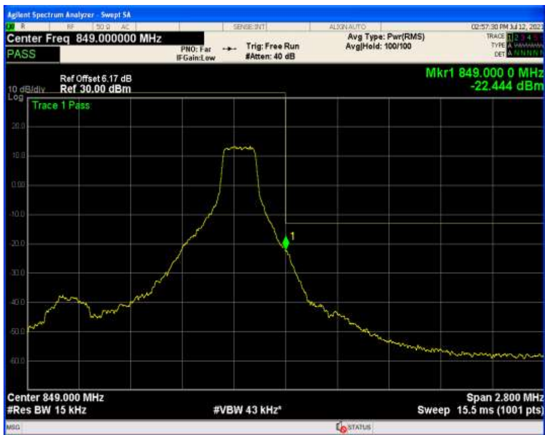
Band26b QPSK BW=1.4MHz Channel=27033 RB Size=6 Position=#0
