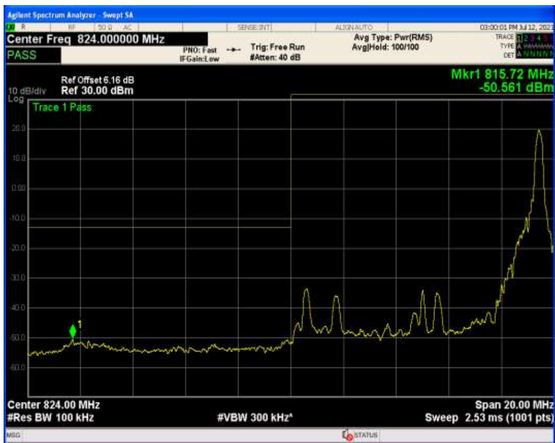
Band26b QAM16 BW=15MHz Channel=26865 RB Size=1 Position=#0
