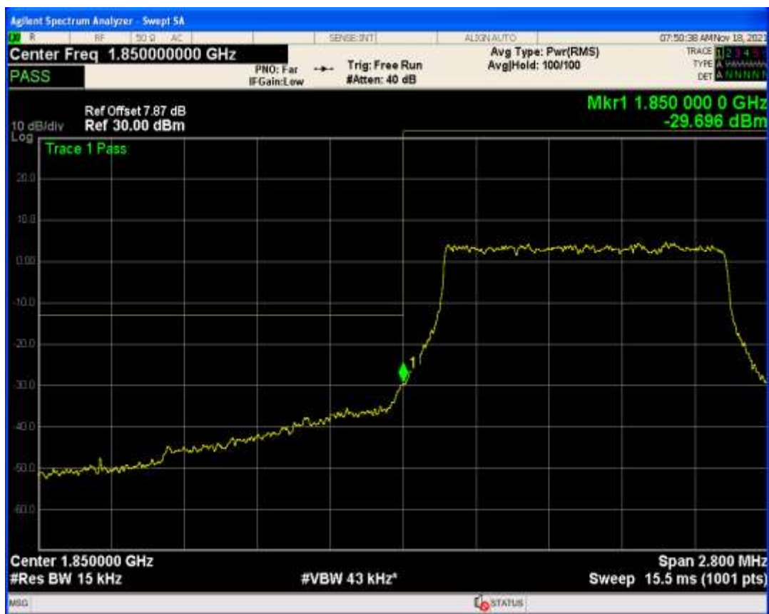
Band25 QPSK BW=1.4MHz Channel=26683 RB Size=6 Position=#0
