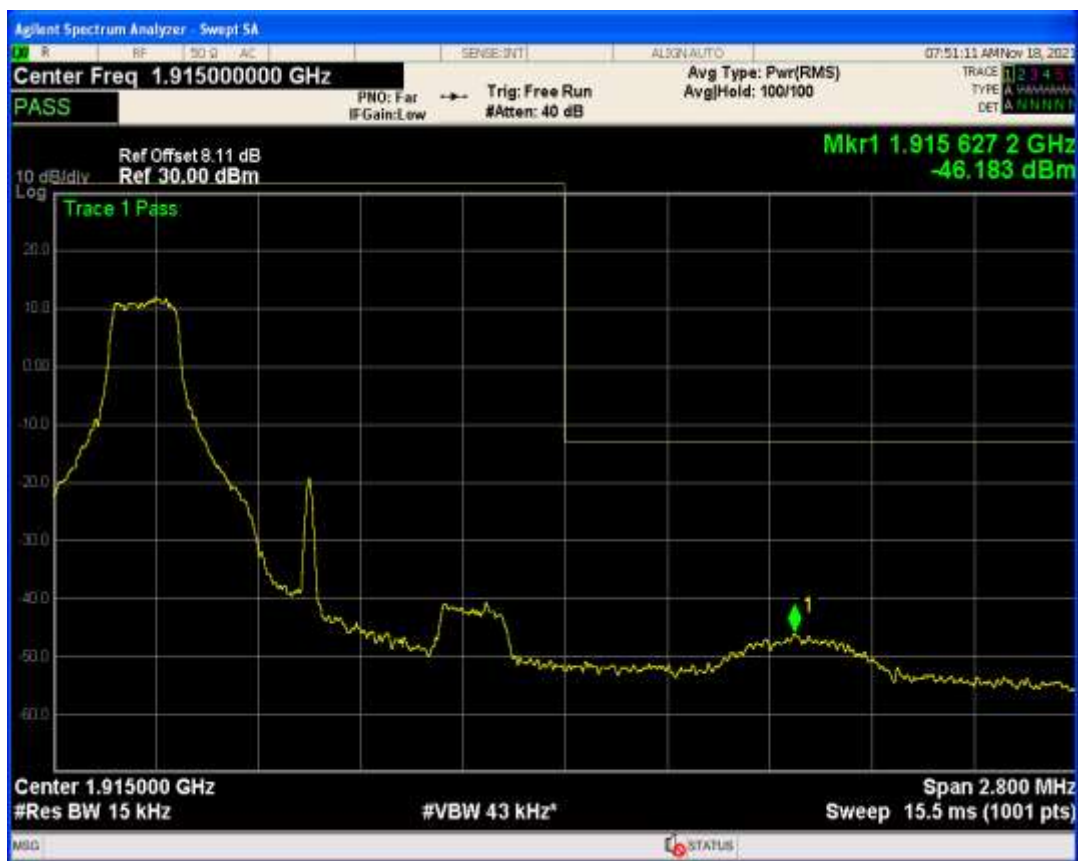
Band25 QAM16 BW=1.4MHz Channel=26683 RB Size=1 Position=#Max
