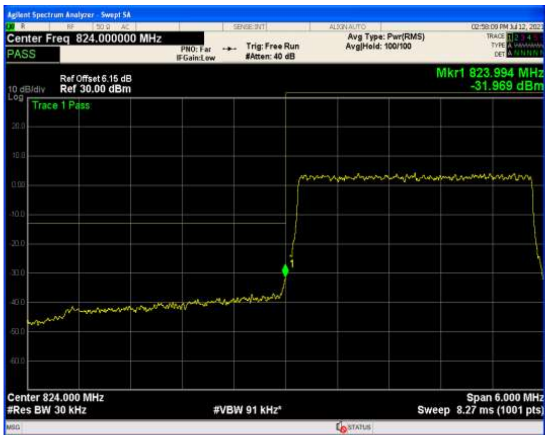
Band26b QPSK BW=3MHz Channel=27025 RB Size=1 Position=#0
