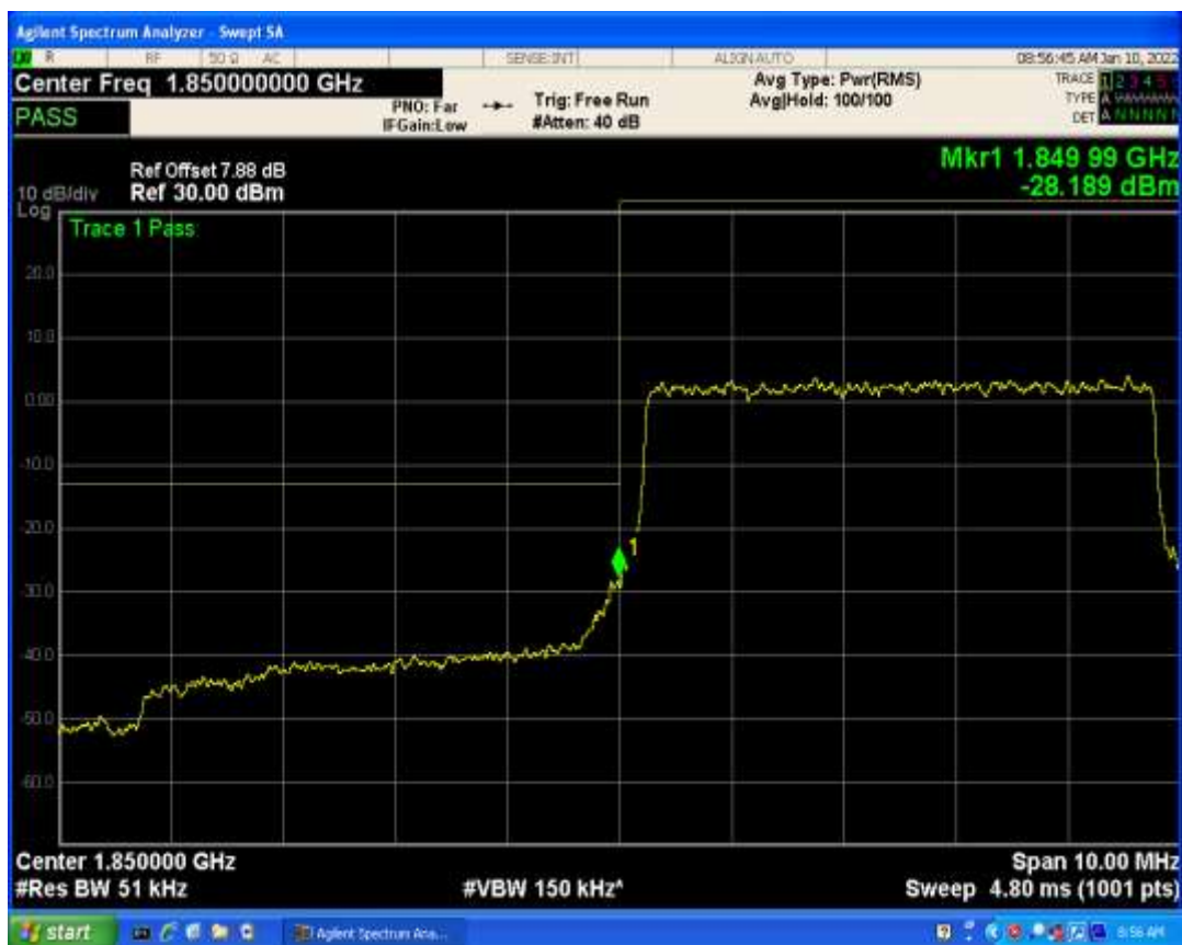
Band25 QAM16 BW=1.4MHz Channel=26683 RB Size=1 Position=#0
