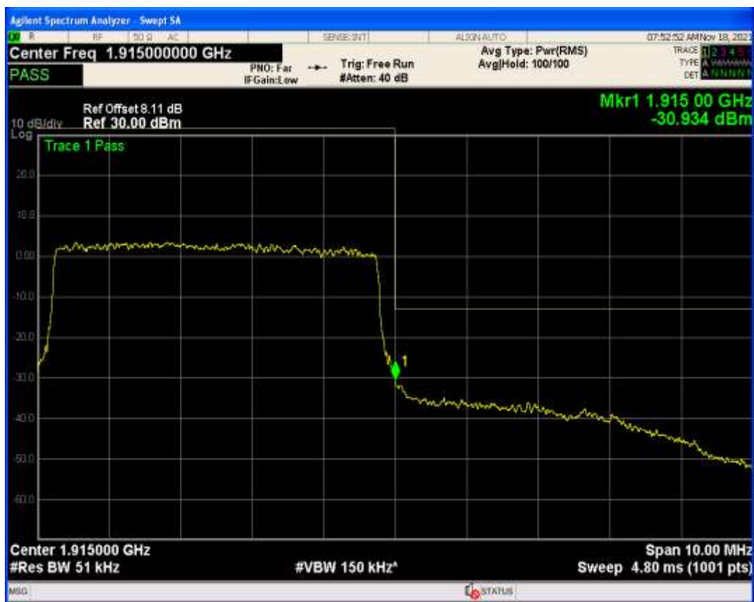
Band25 QPSK BW=5MHz Channel=26665 RB Size=1 Position=#Max
