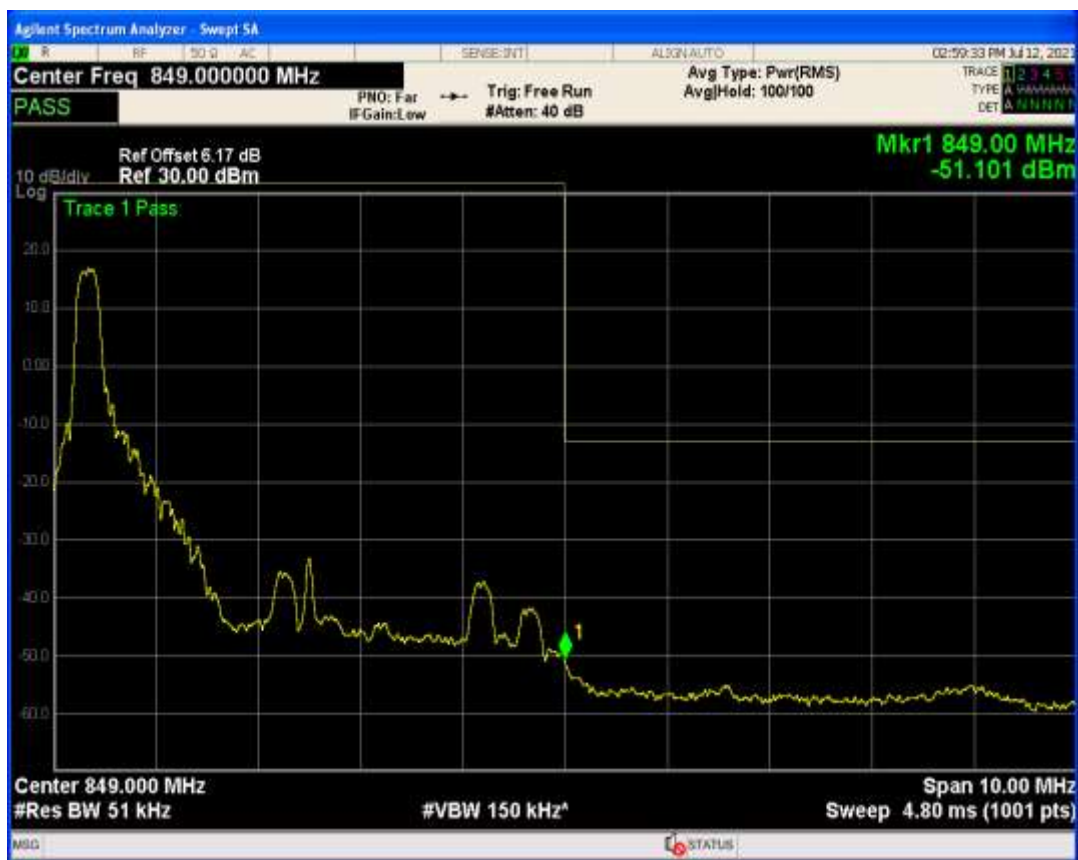
Band26b QAM16 BW=5MHz Channel=26815 RB Size=25 Position=#0
