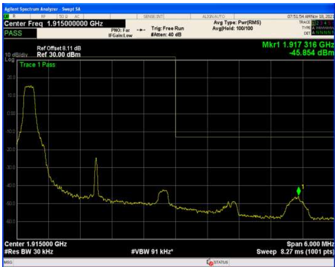
Band25 QPSK BW=3MHz Channel=26055 RB Size=15 Position=#0
