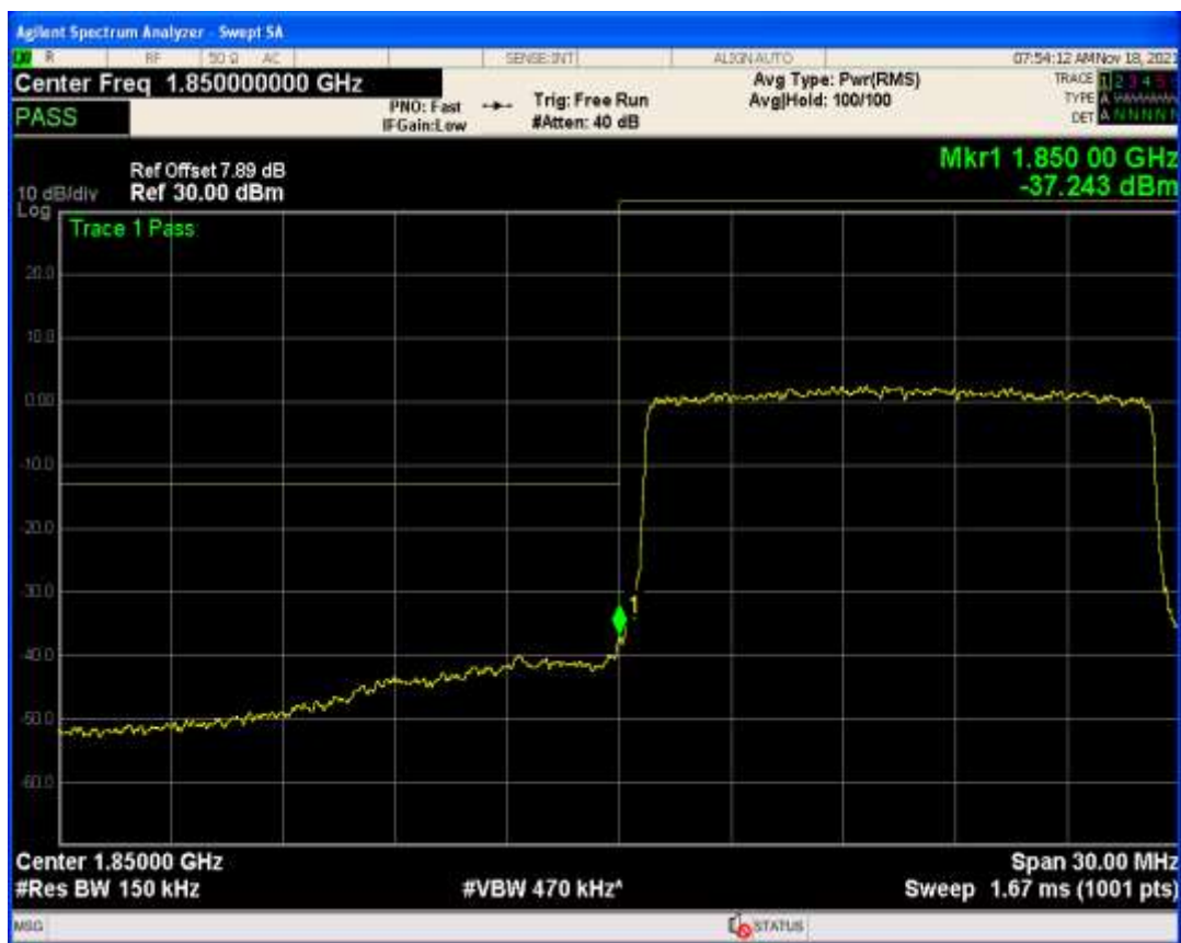
Band25 QAM16 BW=15MHz Channel=26115 RB Size=1 Position=#Max
