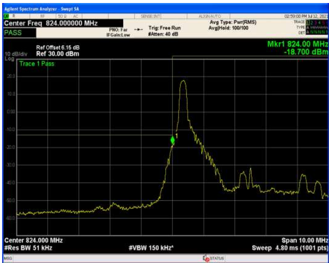
Band26b QPSK BW=5MHz Channel=26815 RB Size=1 Position=#Max
