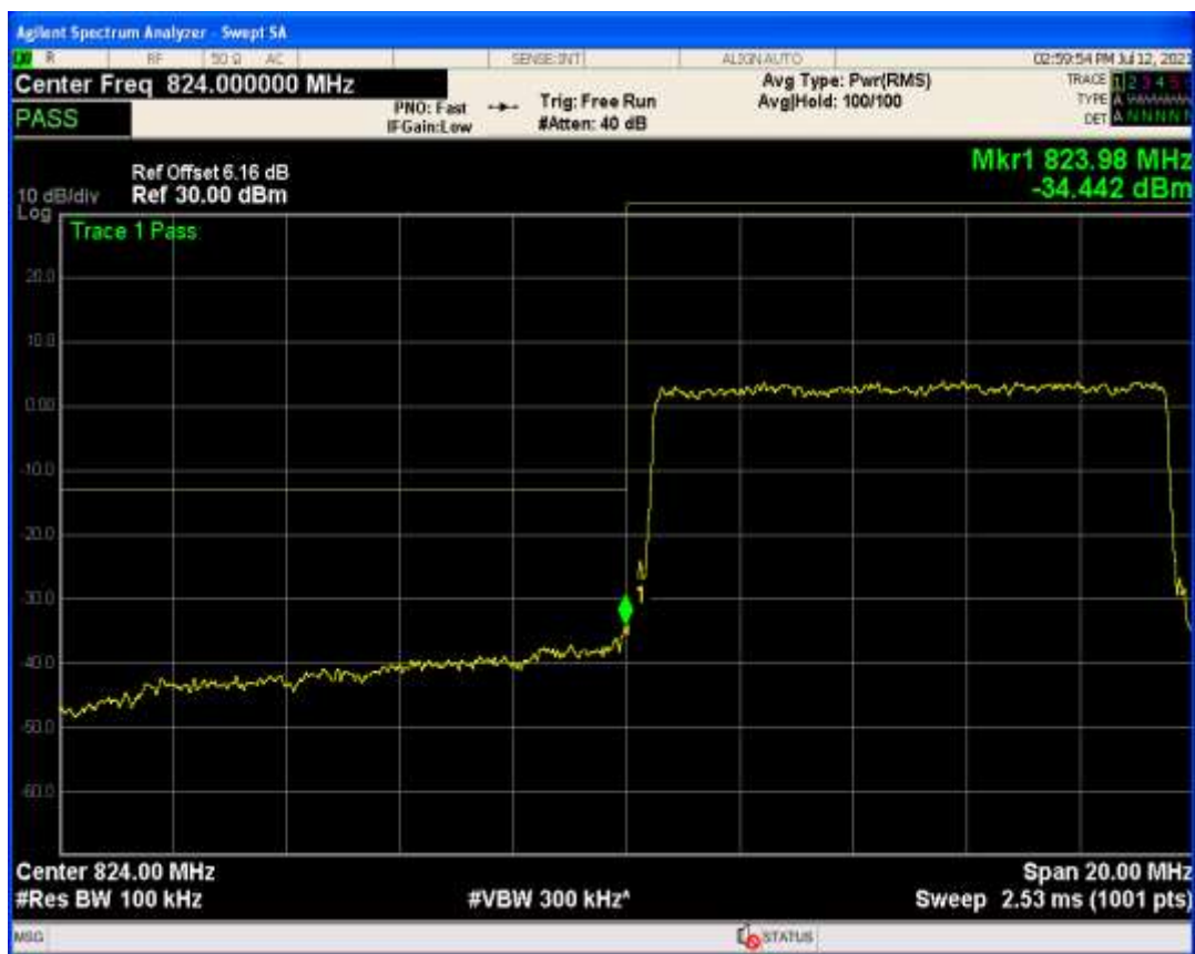
Band26b QPSK BW=10MHz Channel=26990 RB Size=1 Position=#0
