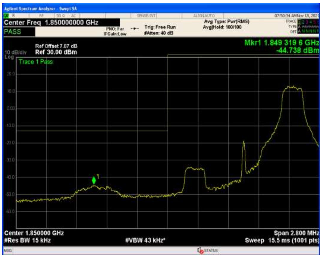
Band25 QPSK BW=1.4MHz Channel=26047 RB Size=1 Position=#0
