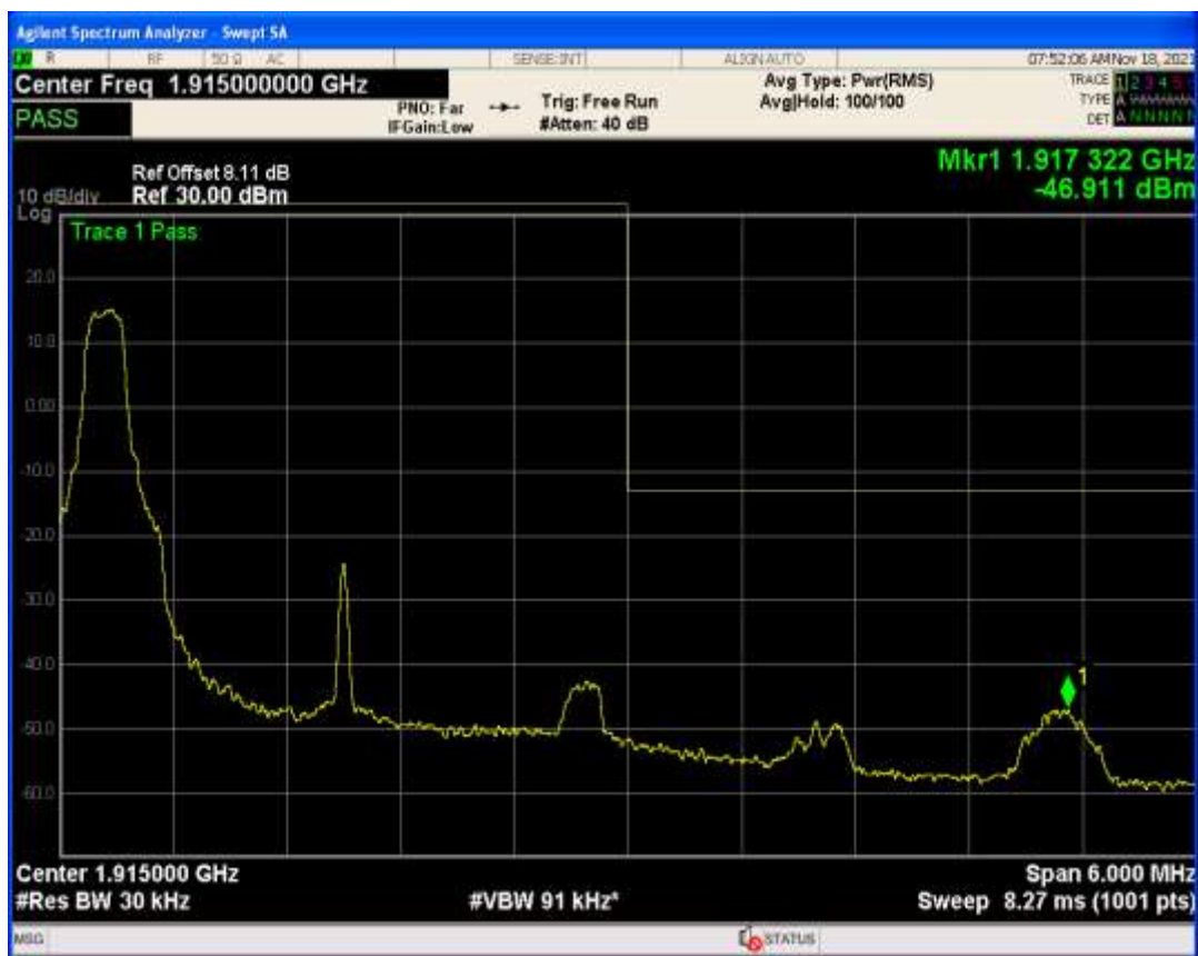
Band25 QAM16 BW=20MHz Channel=26590 RB Size=1 Position=#Max
