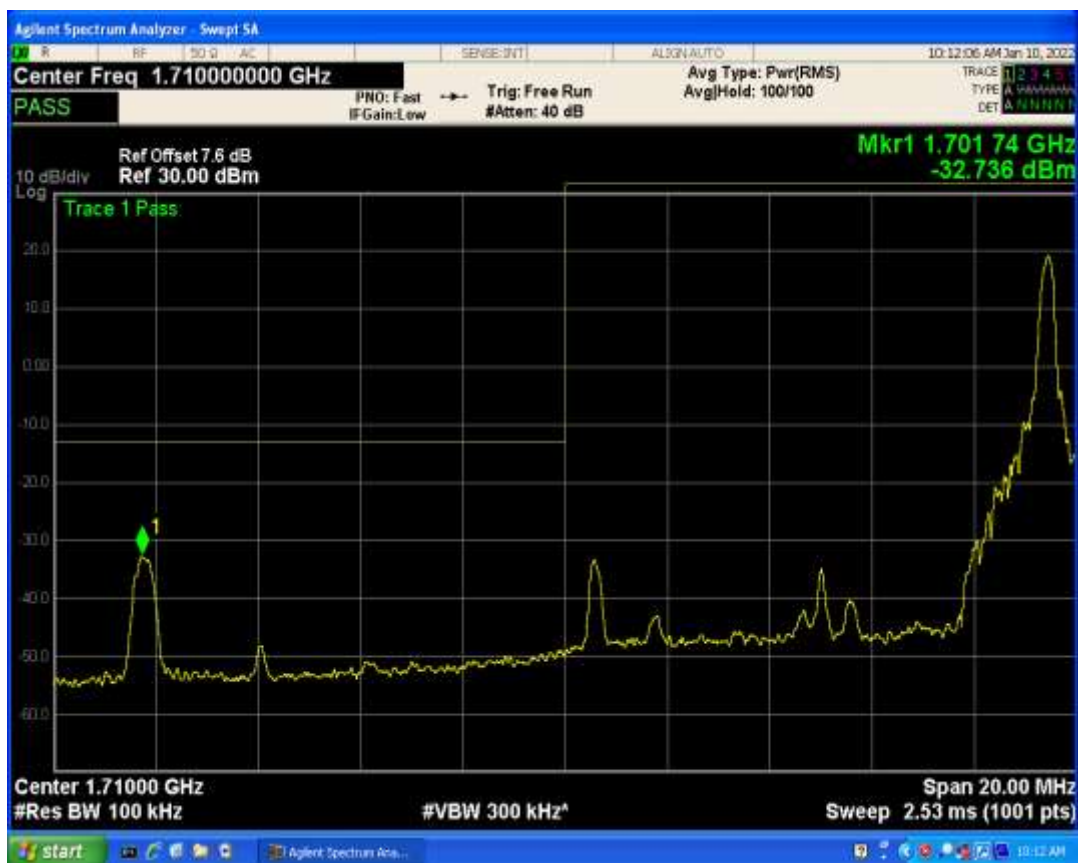
Band4 QAM16 BW=10MHz Channel=20000 RB Size=1 Position=#0
