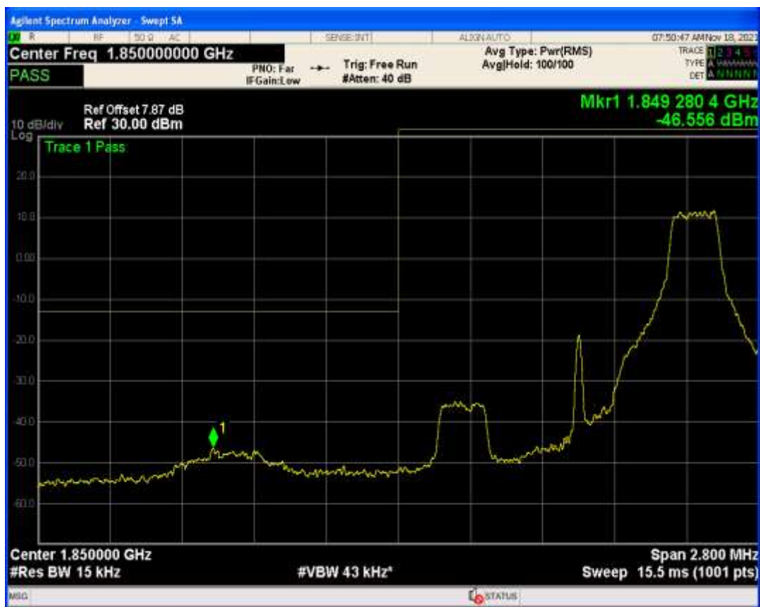
Band25 QAM16 BW=15MHz Channel=26615 RB Size=1 Position=#0
