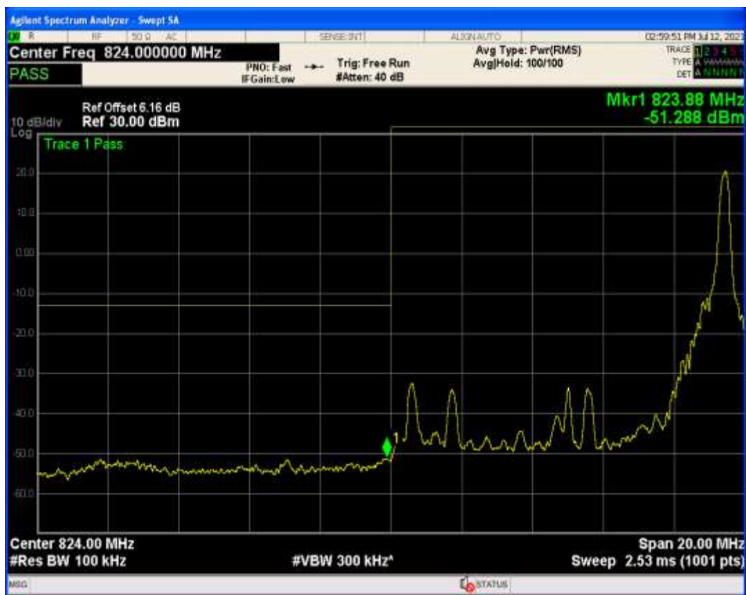
Band26b QPSK BW=15MHz Channel=26865 RB Size=1 Position=#0
