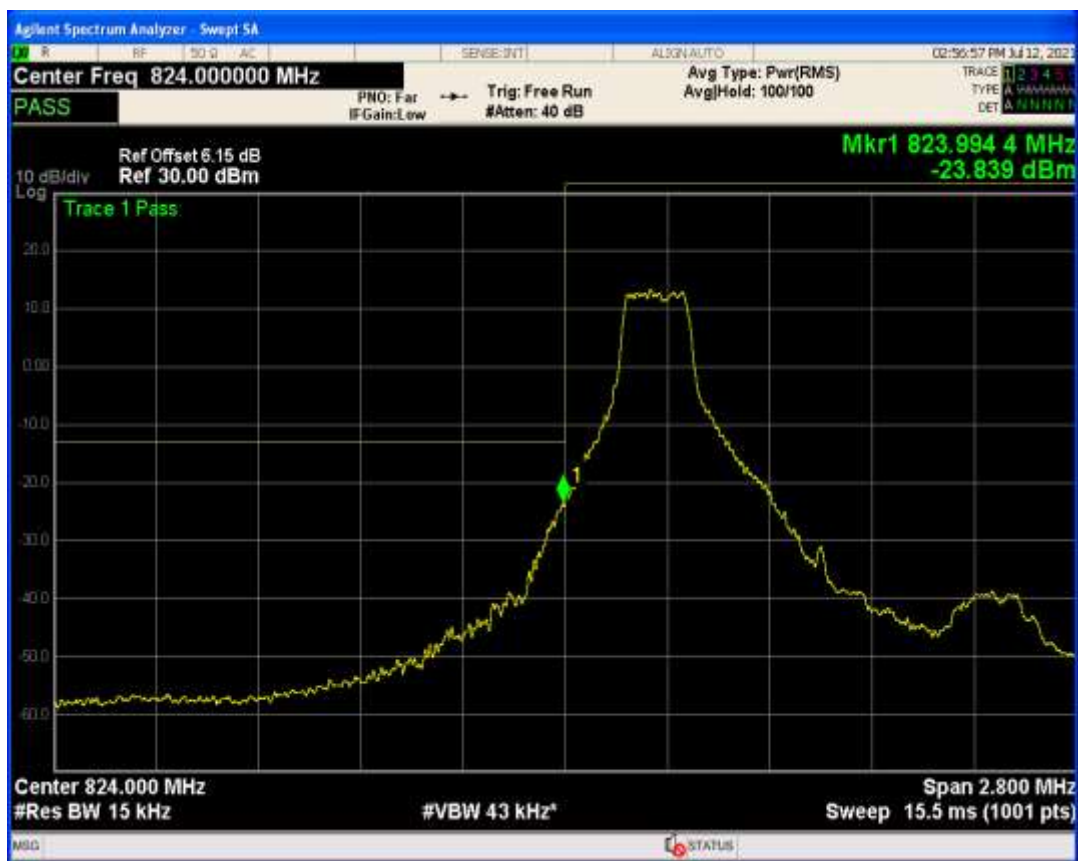
Band26b QPSK BW=1.4MHz Channel=26797 RB Size=1 Position=#Max
