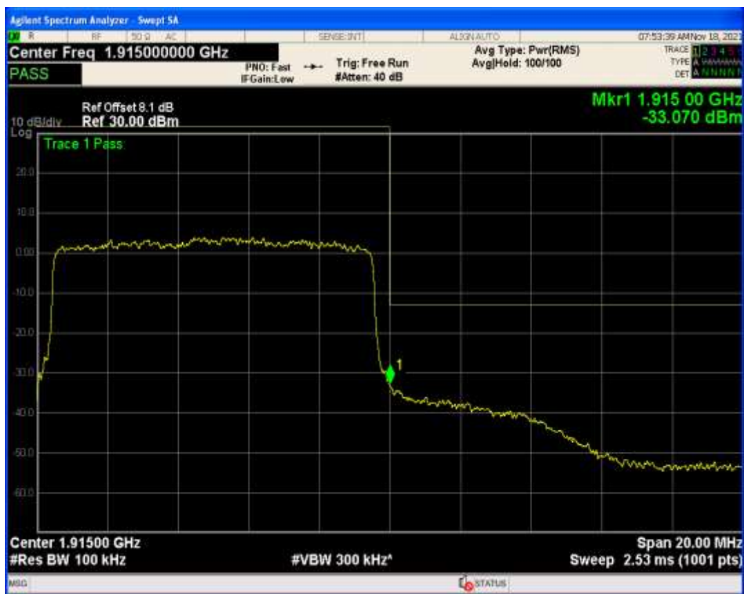
Band25 QPSK BW=10MHz Channel=26640 RB Size=1 Position=#Max
