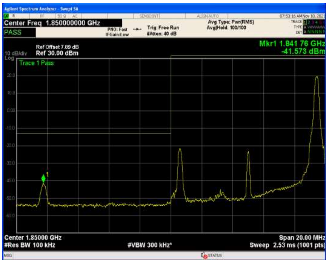
Band25 QPSK BW=10MHz Channel=26090 RB Size=1 Position=#0
