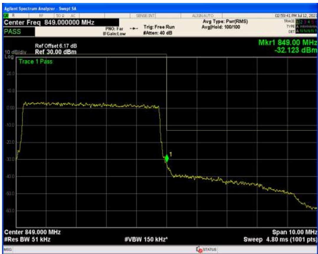
Band26b QPSK BW=1.4MHz Channel=27033 RB Size=1 Position=#Max
