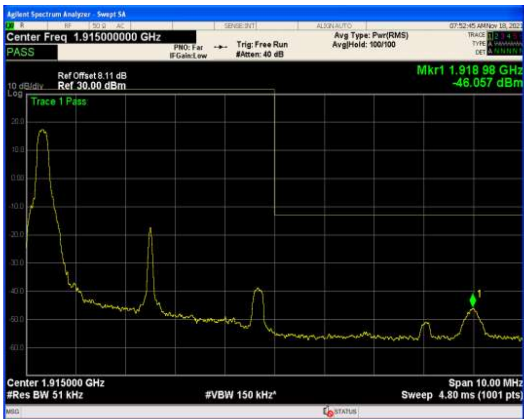
Band25 QPSK BW=5MHz Channel=26065 RB Size=25 Position=#0
