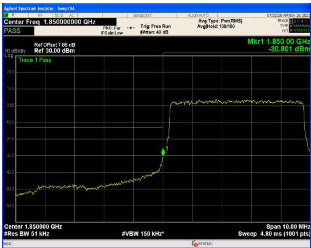
Band25 QPSK BW=5MHz Channel=26665 RB Size=25 Position=#0
