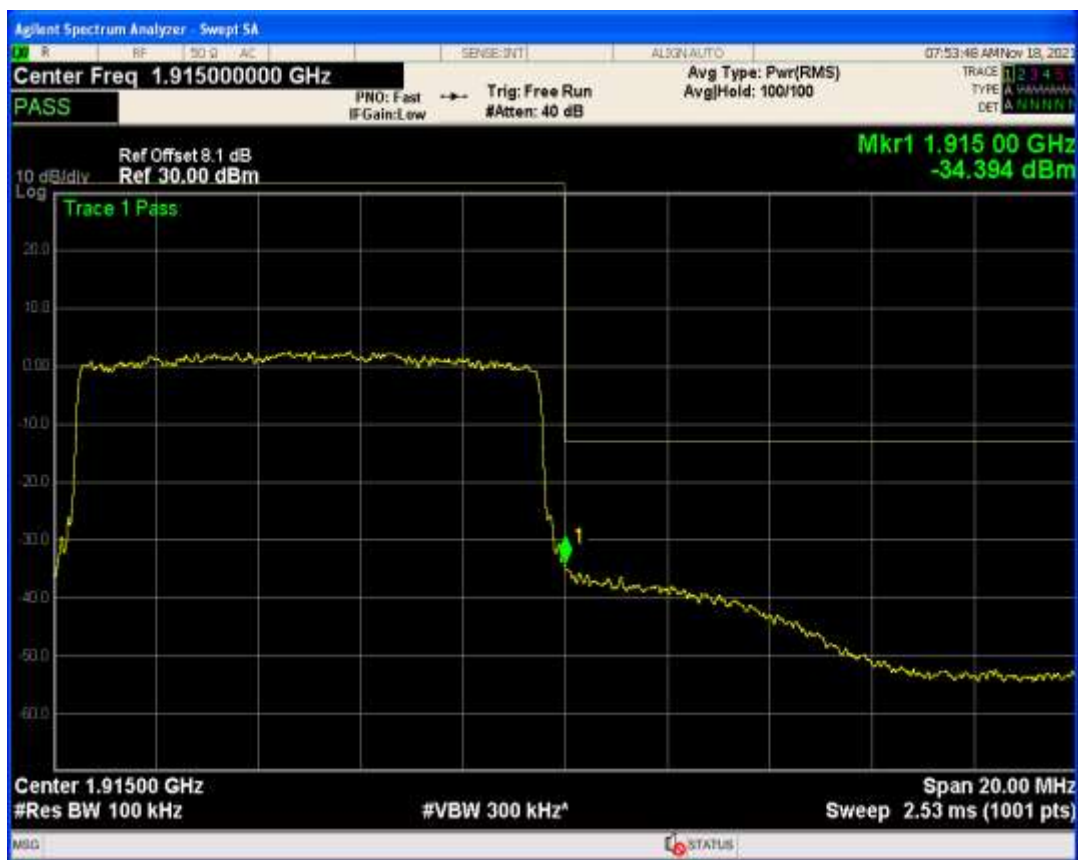
Band25 QAM16 BW=10MHz Channel=26640 RB Size=1 Position=#Max
