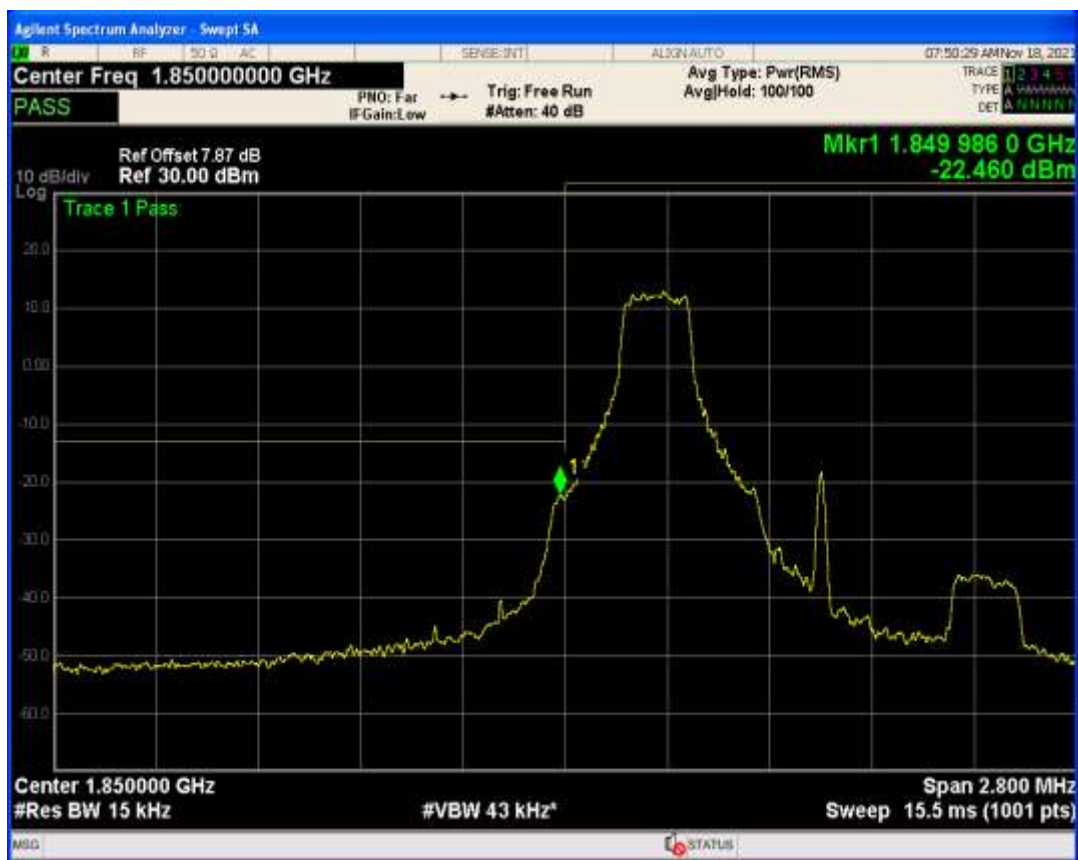
Band25 QAM16 BW=5MHz Channel=26665 RB Size=25 Position=#0
