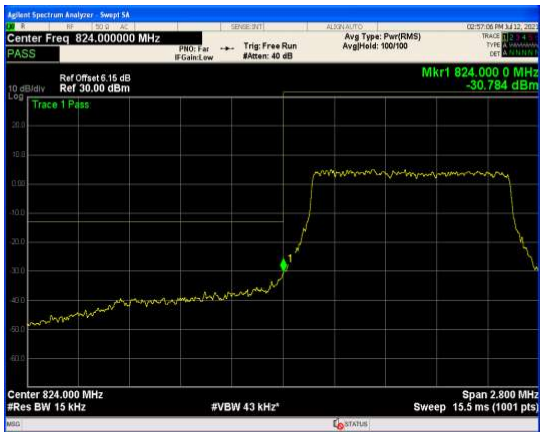
Band26b QPSK BW=1.4MHz Channel=27033 RB Size=1 Position=#0
