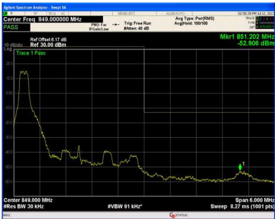
Band26b QAM16 BW=5MHz Channel=26815 RB Size=1 Position=#0
