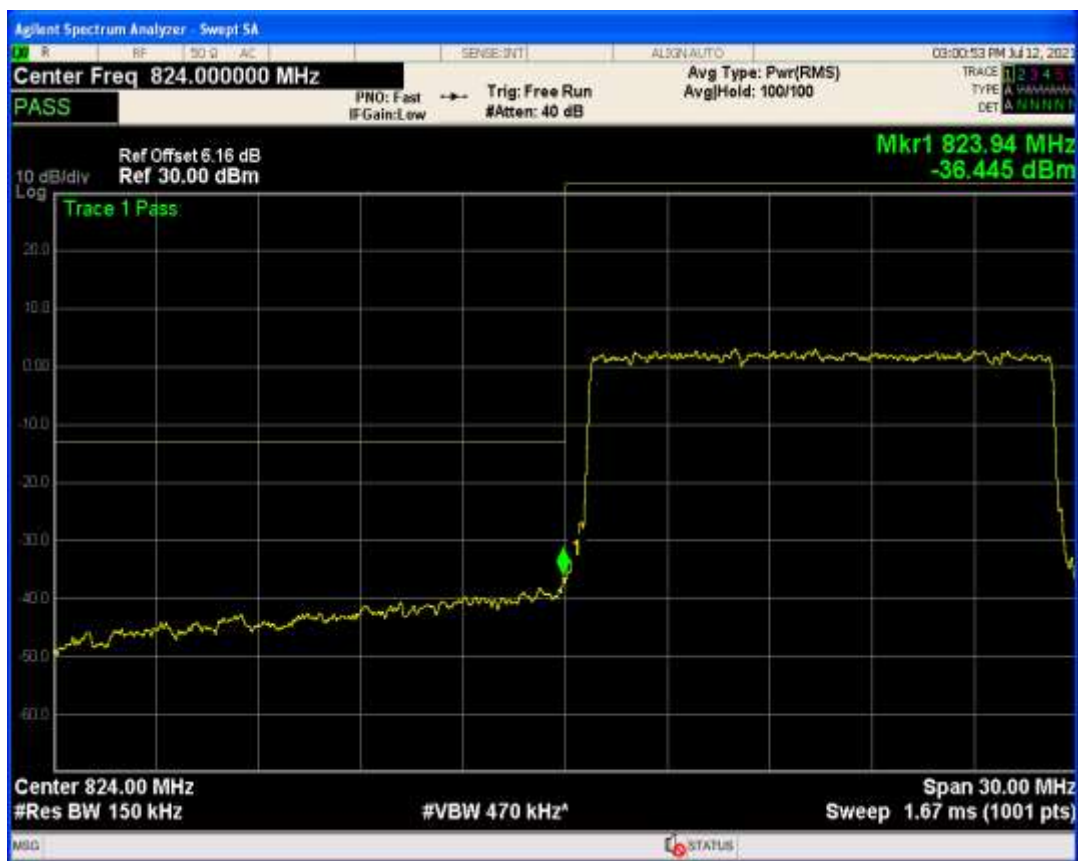
Band26b QAM16 BW=15MHz Channel=26865 RB Size=1 Position=#Max
