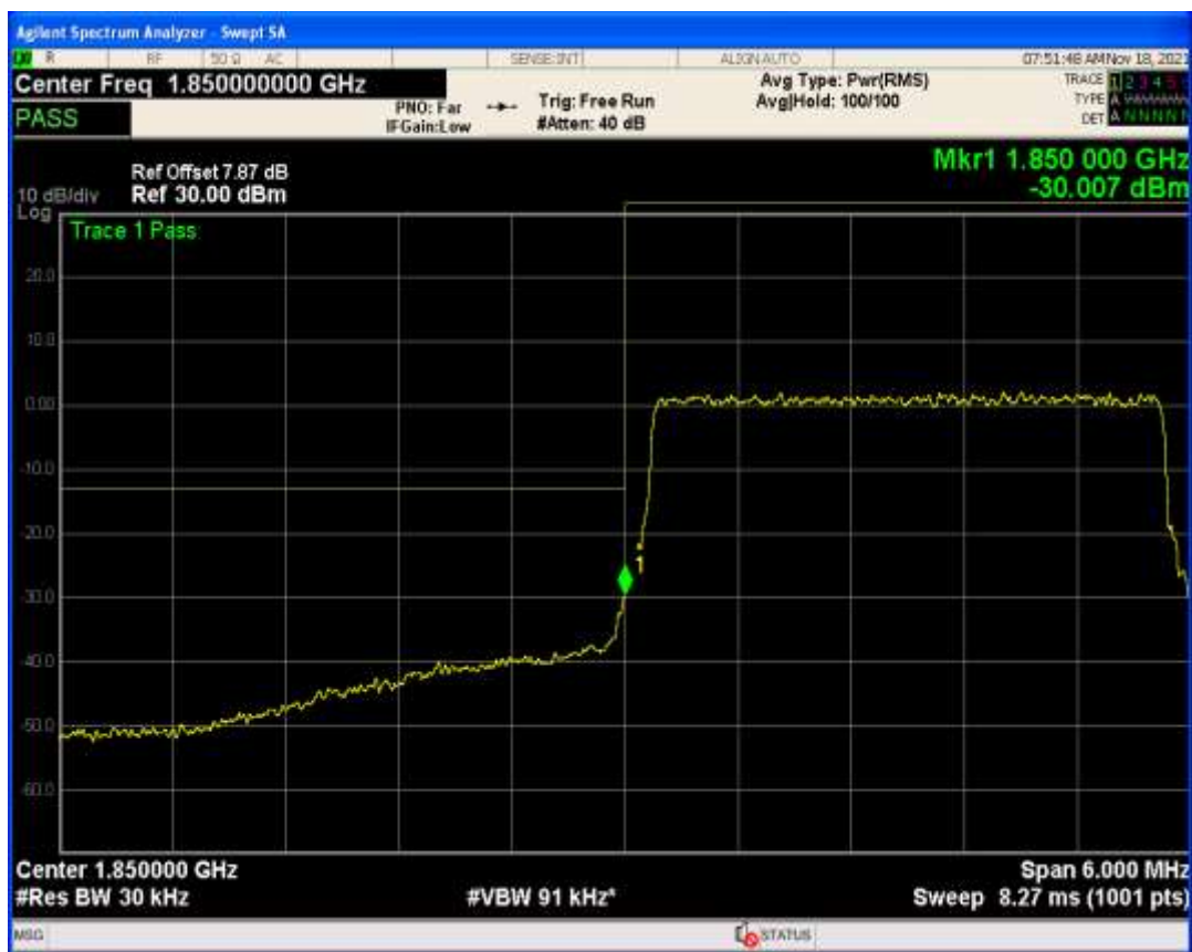
Band25 QAM16 BW=3MHz Channel=26055 RB Size=1 Position=#Max
