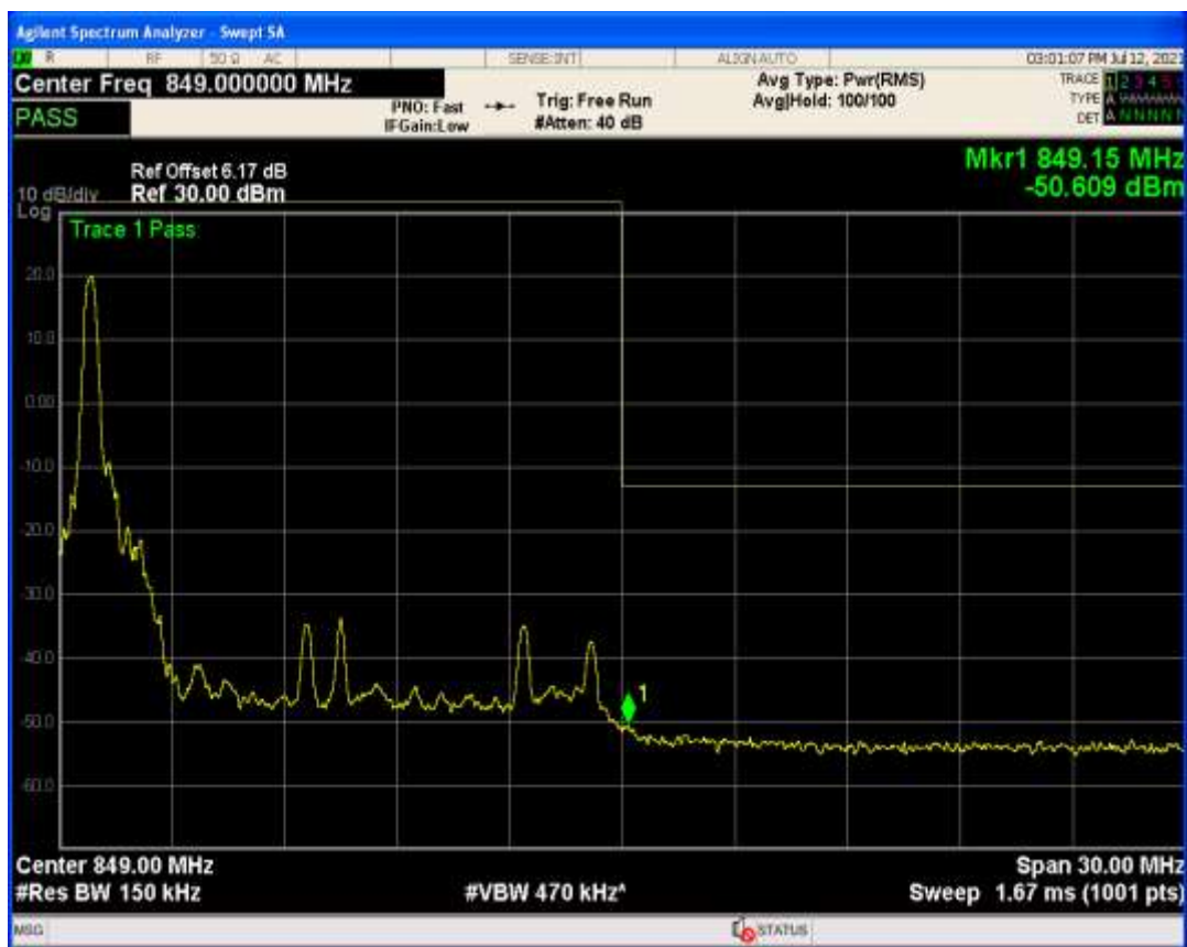
Band26b QAM16 BW=15MHz Channel=26865 RB Size=75 Position=#0
