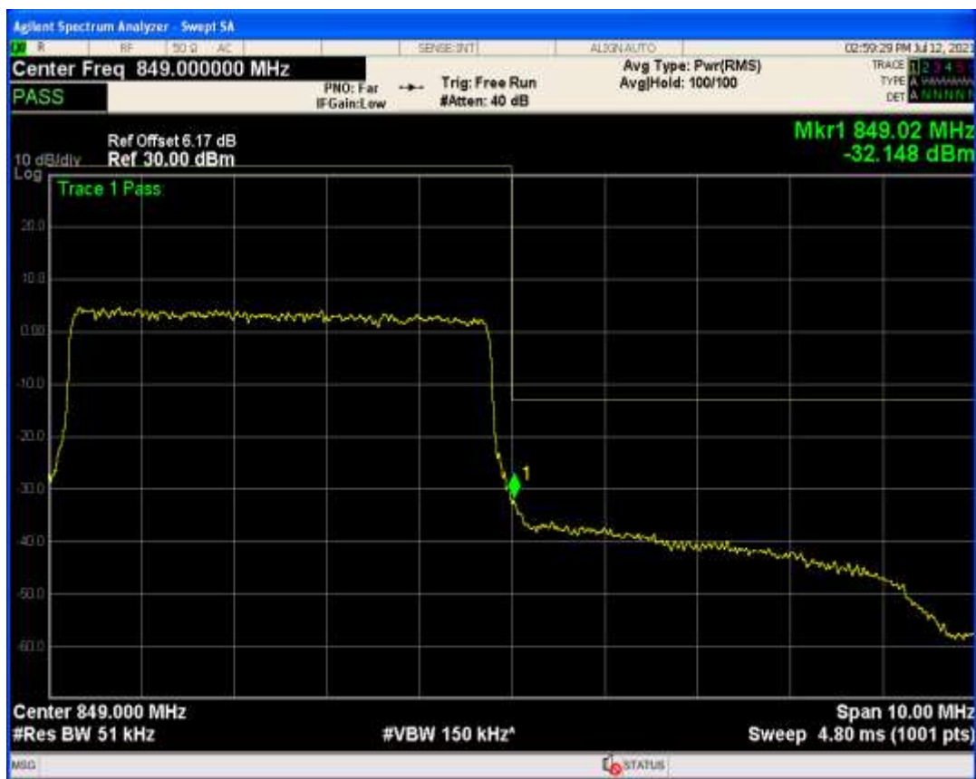
Band26b QPSK BW=5MHz Channel=26815 RB Size=25 Position=#0
