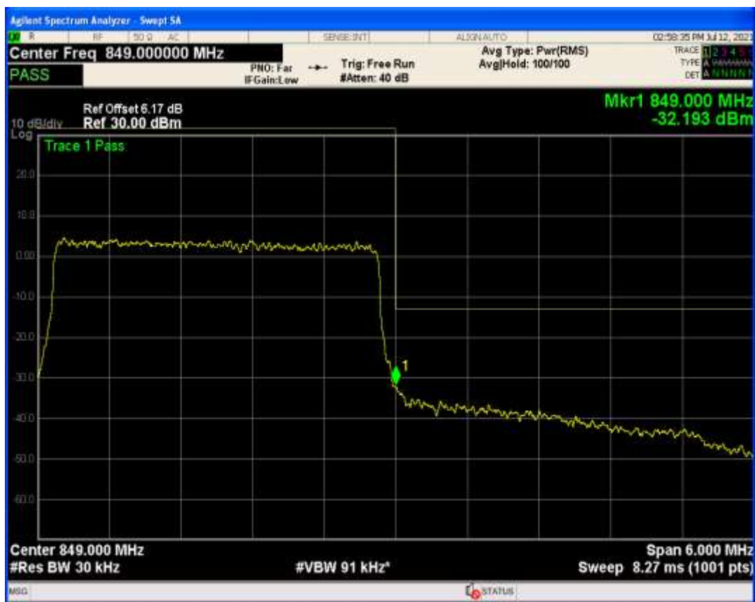
Band26b QPSK BW=5MHz Channel=27015 RB Size=1 Position=#Max
