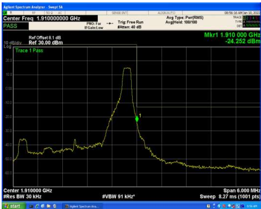
Band2 QPSK BW=3MHz Channel=18615 RB Size=1 Position=#0
