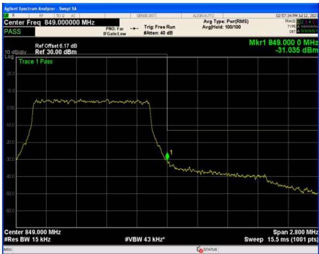
Band26b QPSK BW=1.4MHz Channel=26797 RB Size=6 Position=#0
