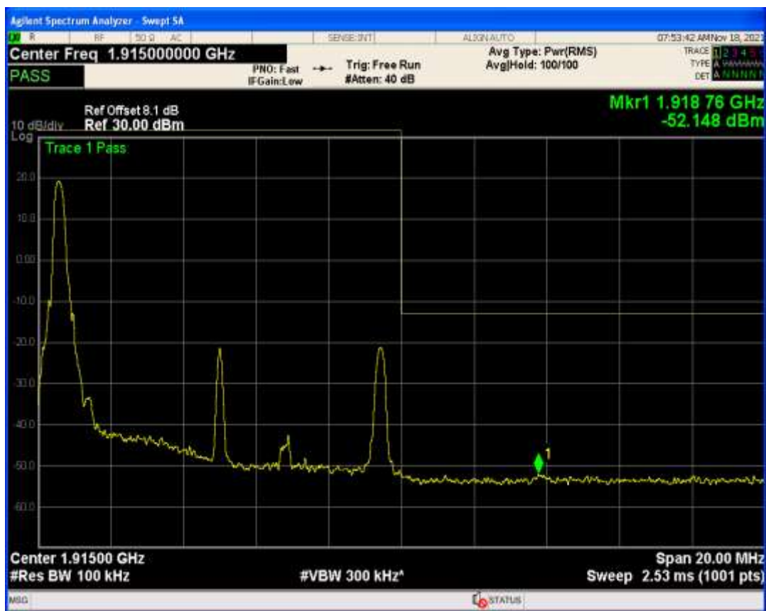
Band25 QAM16 BW=5MHz Channel=26065 RB Size=1 Position=#0
