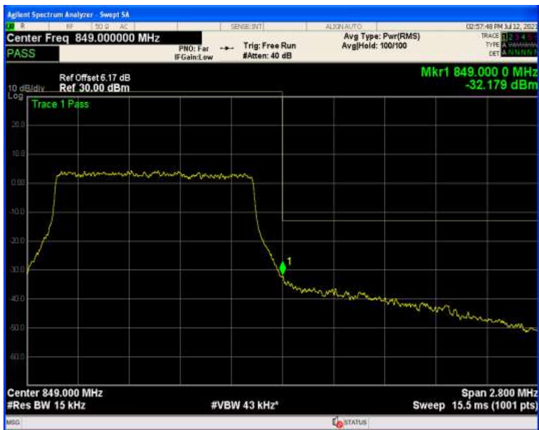
Band26b QAM16 BW=1.4MHz Channel=27033 RB Size=1 Position=#Max
