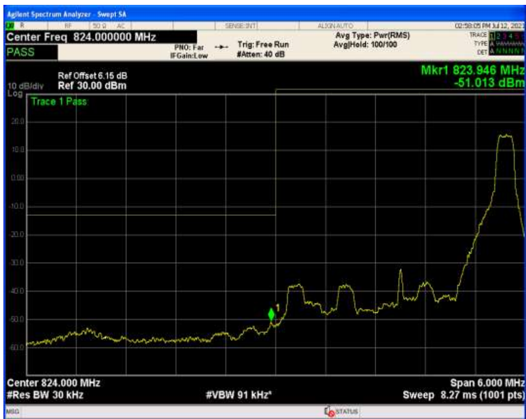
Band4 QAM16 BW=1.4MHz Channel=20393 RB Size=6 Position=#0
