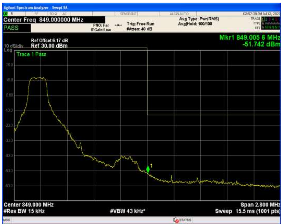
Band26b QAM16 BW=3MHz Channel=27025 RB Size=15 Position=#0
