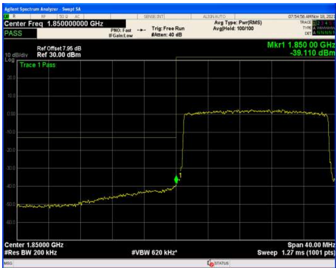
Band25 QAM16 BW=20MHz Channel=26590 RB Size=100 Position=#0
