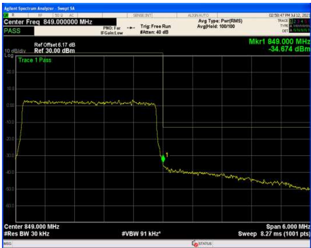
Band26b QAM16 BW=3MHz Channel=27025 RB Size=1 Position=#Max
