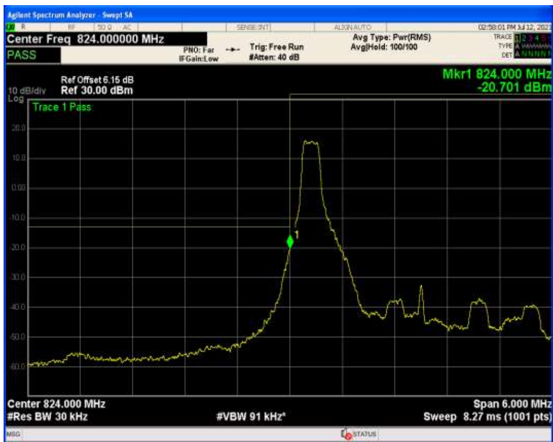
Band26b QPSK BW=3MHz Channel=26805 RB Size=1 Position=#Max
