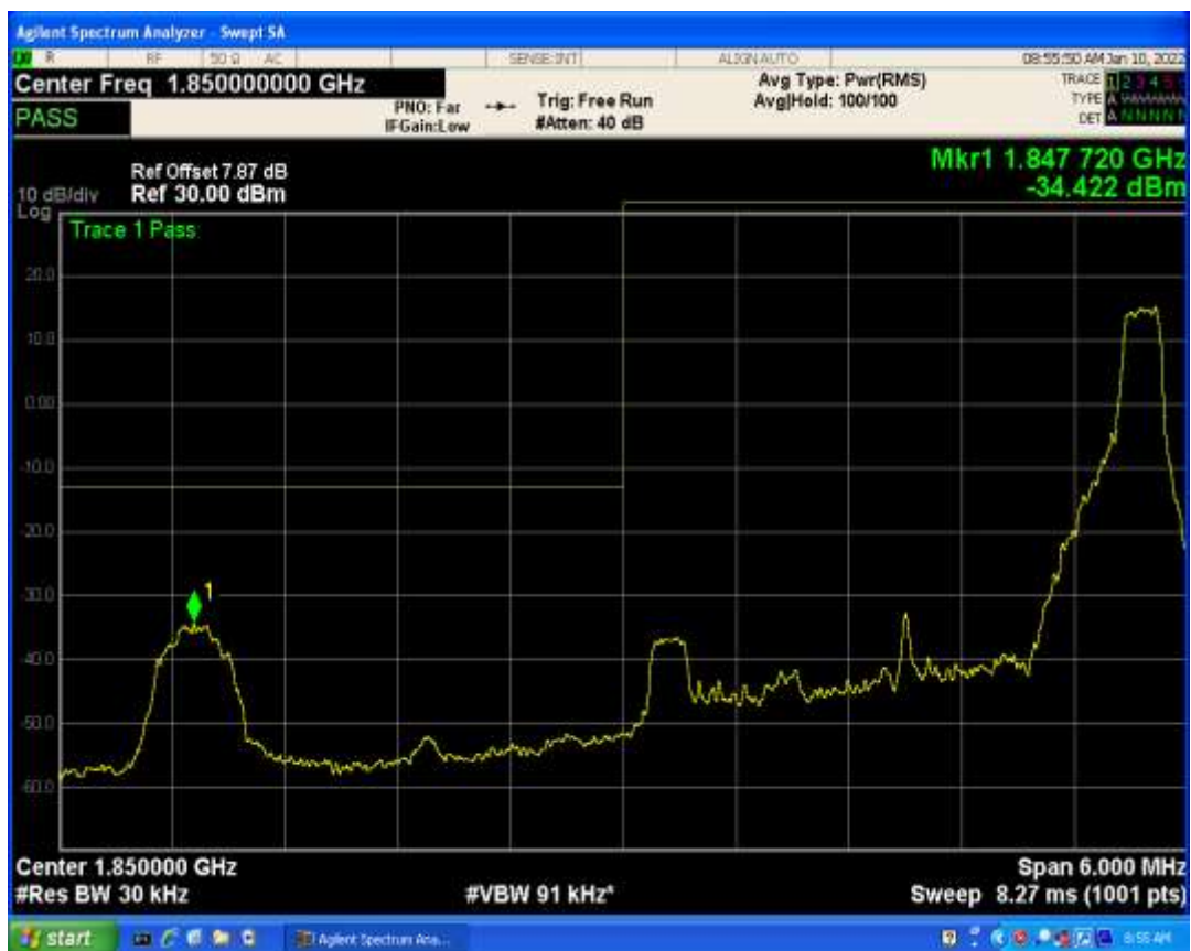
Band2 QPSK BW=3MHz Channel=19185 RB Size=1 Position=#0
