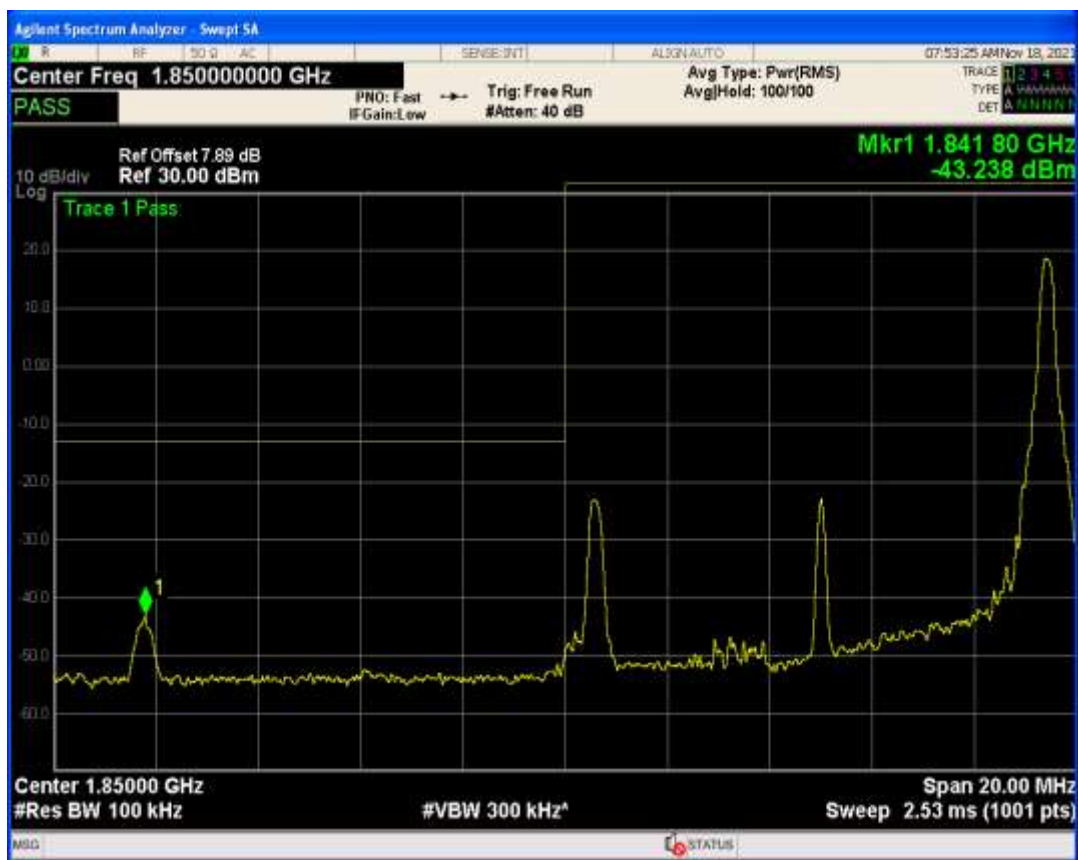
Band25 QAM16 BW=10MHz Channel=26090 RB Size=1 Position=#0
