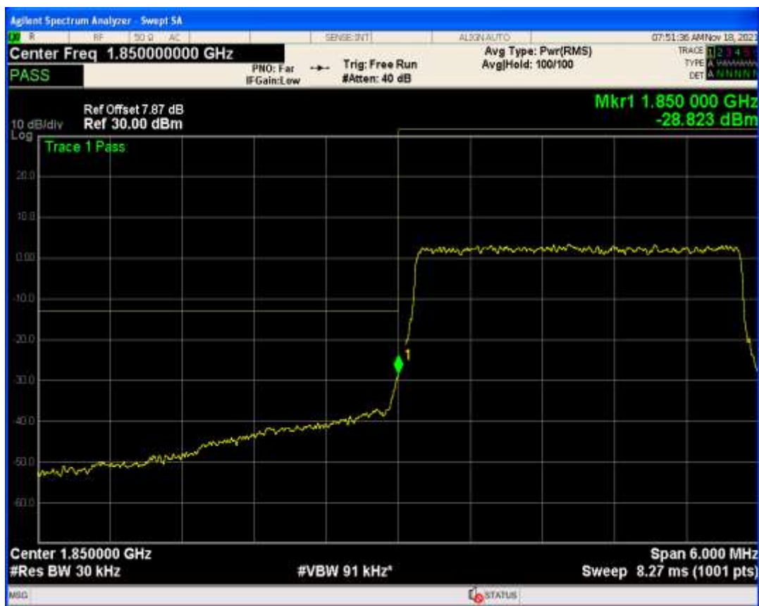
Band25 QPSK BW=3MHz Channel=26055 RB Size=1 Position=#Max
