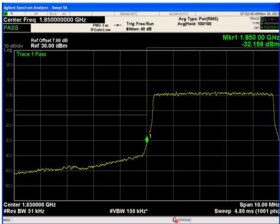
Band25 QAM16 BW=3MHz Channel=26675 RB Size=1 Position=#0
