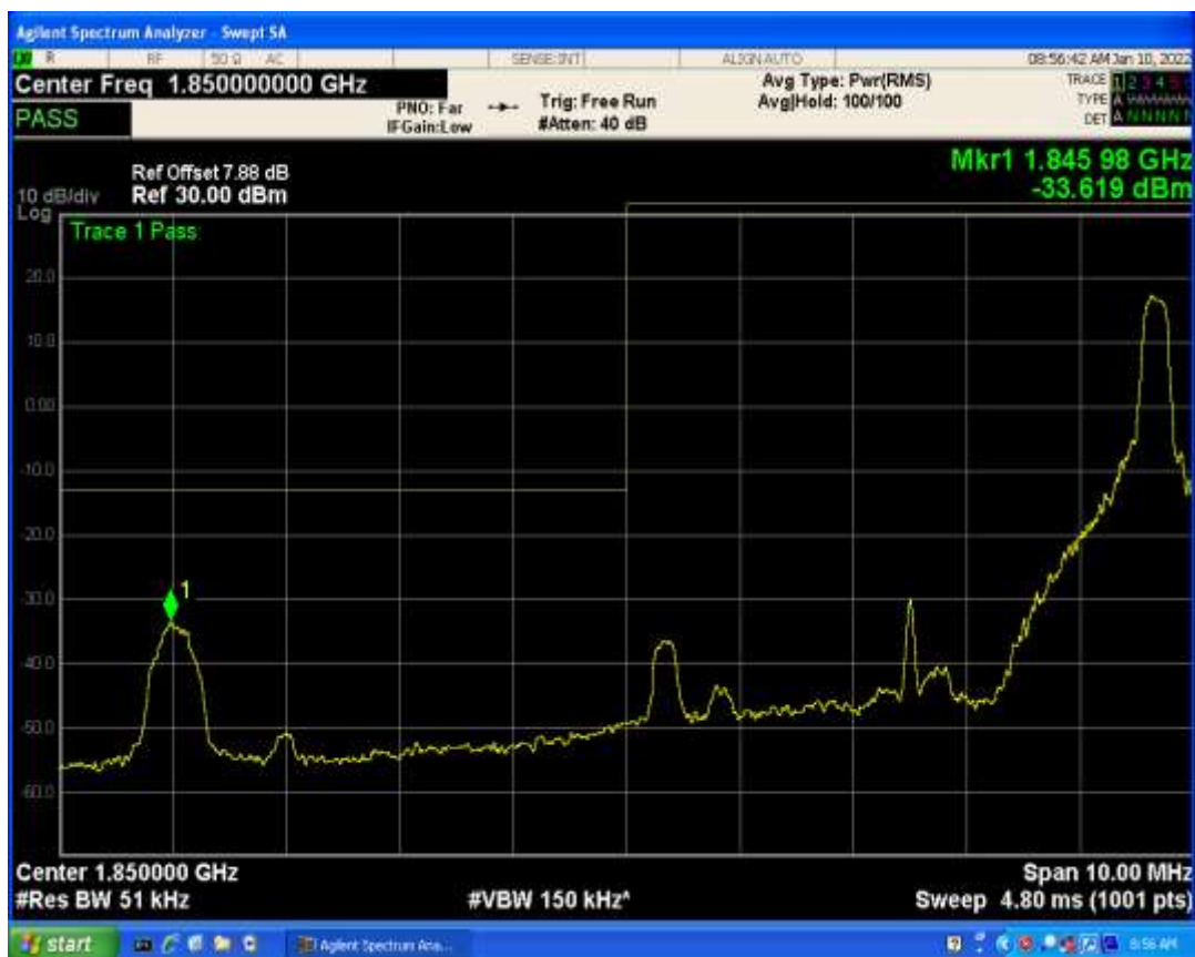
Band2 QPSK BW=5MHz Channel=18625 RB Size=25 Position=#0
