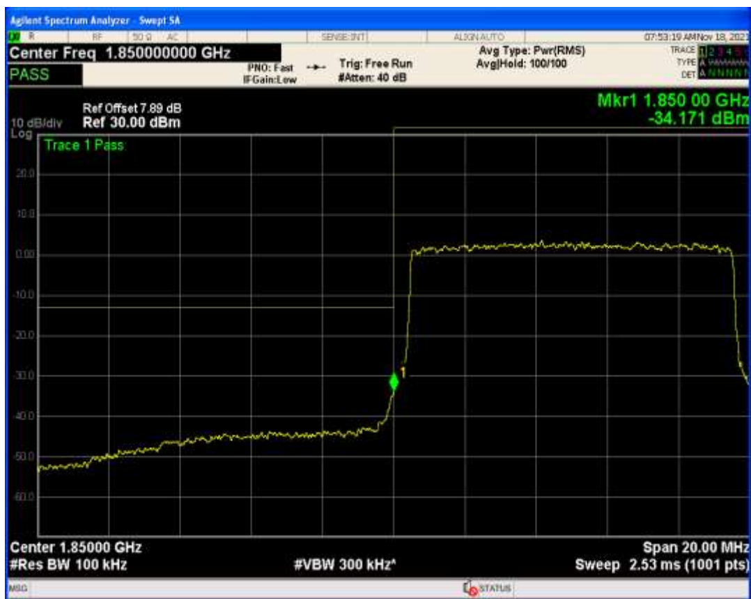
Band25 QPSK BW=10MHz Channel=26090 RB Size=1 Position=#Max
