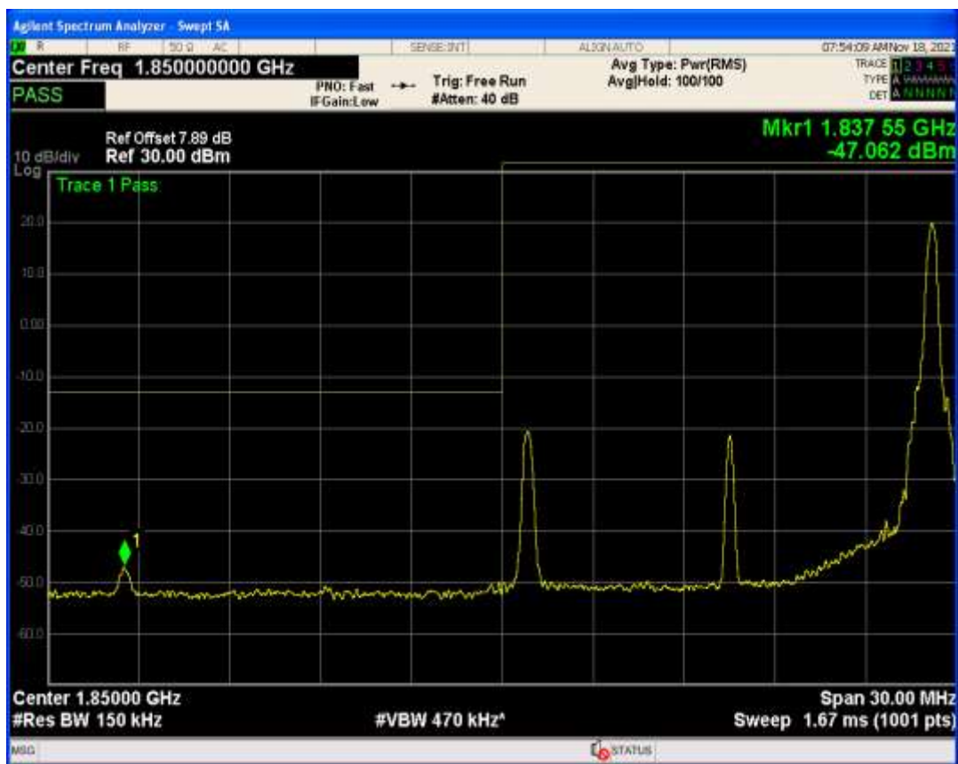
Band25 QAM16 BW=15MHz Channel=26615 RB Size=1 Position=#Max
