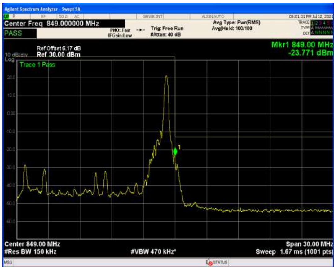
Band26b QPSK BW=15MHz Channel=26965 RB Size=75 Position=#0
