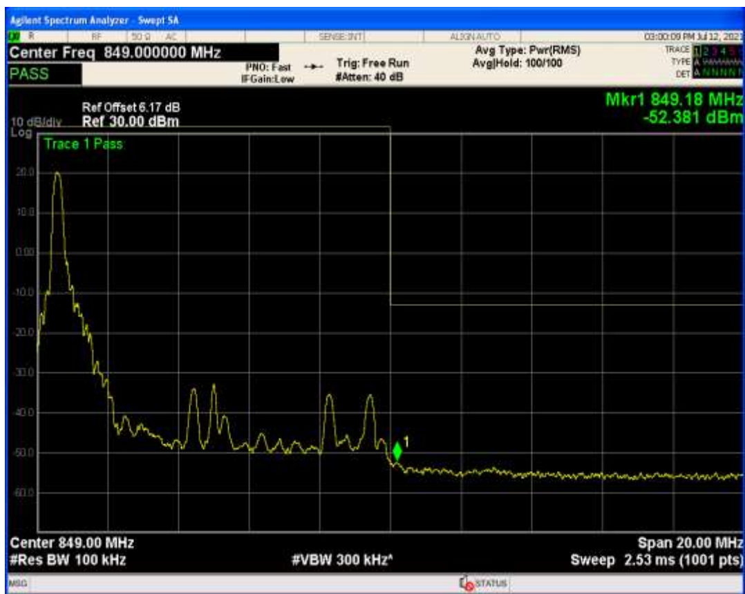
Band26b QPSK BW=10MHz Channel=26840 RB Size=1 Position=#0
