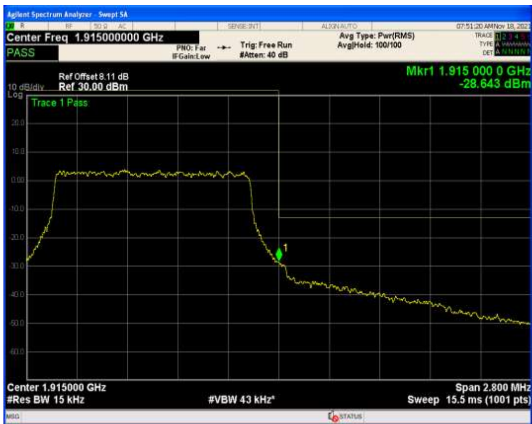
Band25 QAM16 BW=10MHz Channel=26090 RB Size=50 Position=#0
