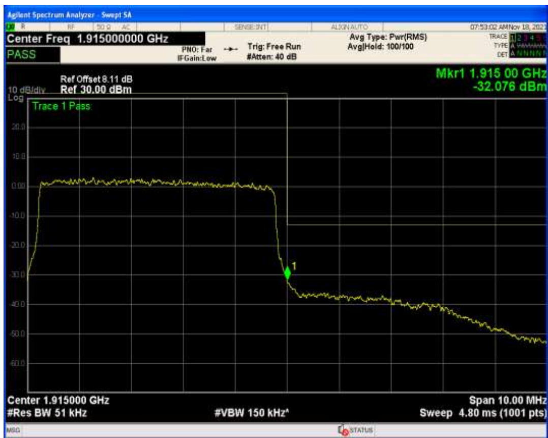
Band25 QPSK BW=1.4MHz Channel=26047 RB Size=6 Position=#0
