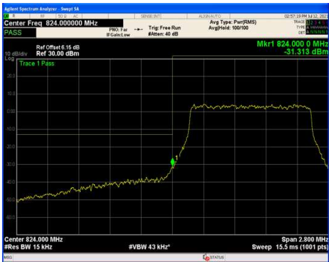
Band26b QAM16 BW=1.4MHz Channel=26797 RB Size=1 Position=#Max
