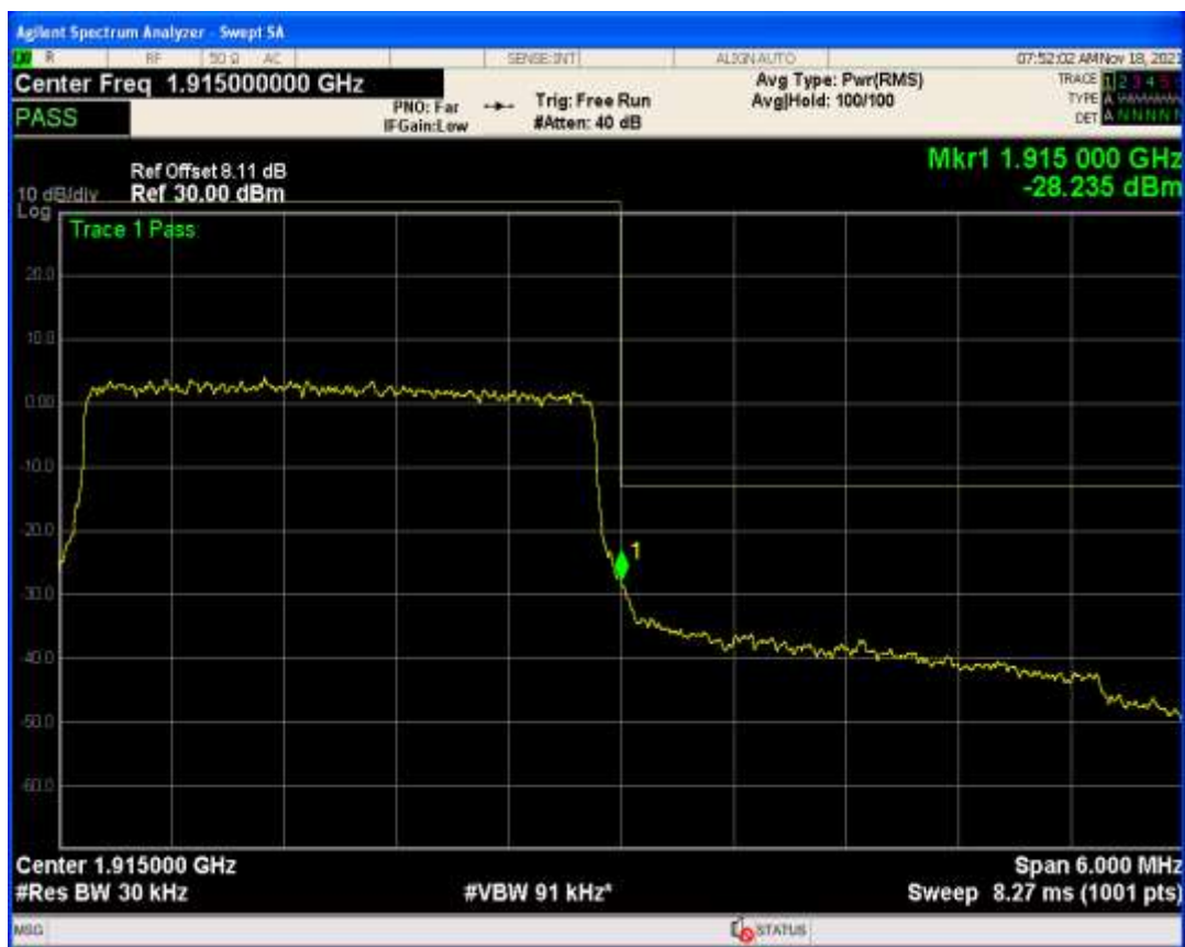
Band25 QPSK BW=3MHz Channel=26675 RB Size=1 Position=#Max
