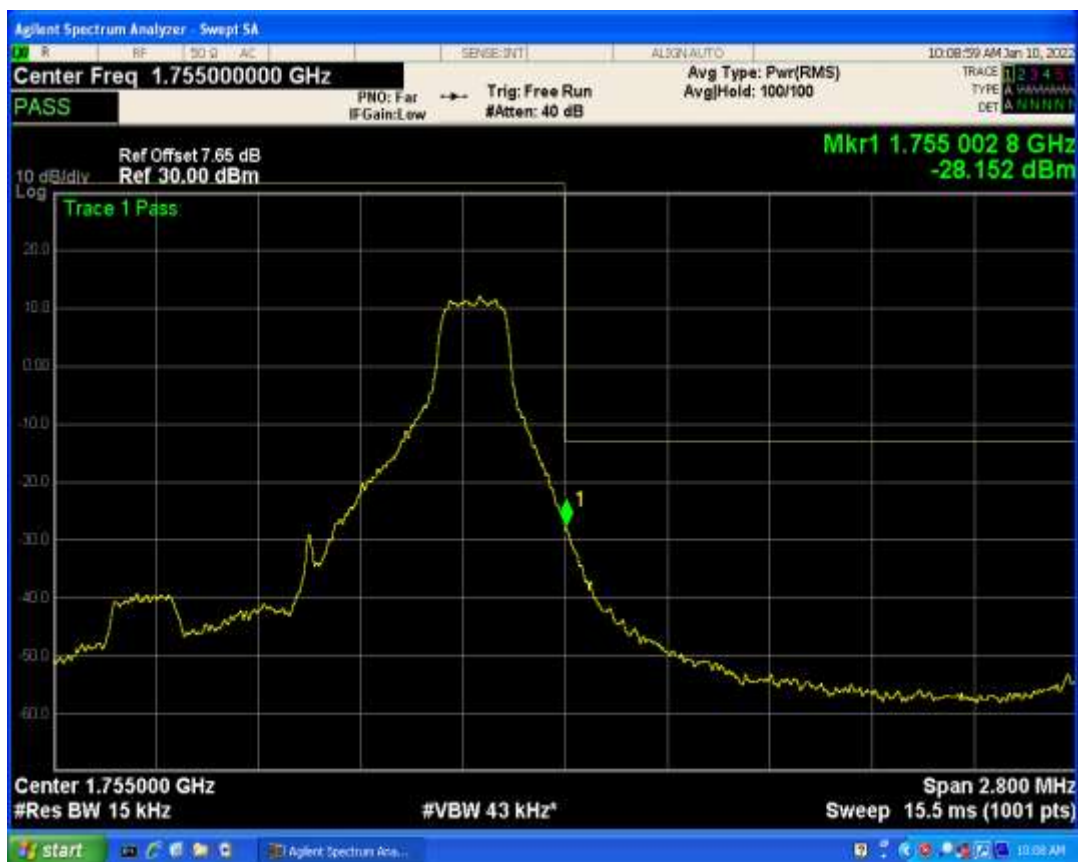
Band4 QAM16 BW=10MHz Channel=20000 RB Size=1 Position=#Max
