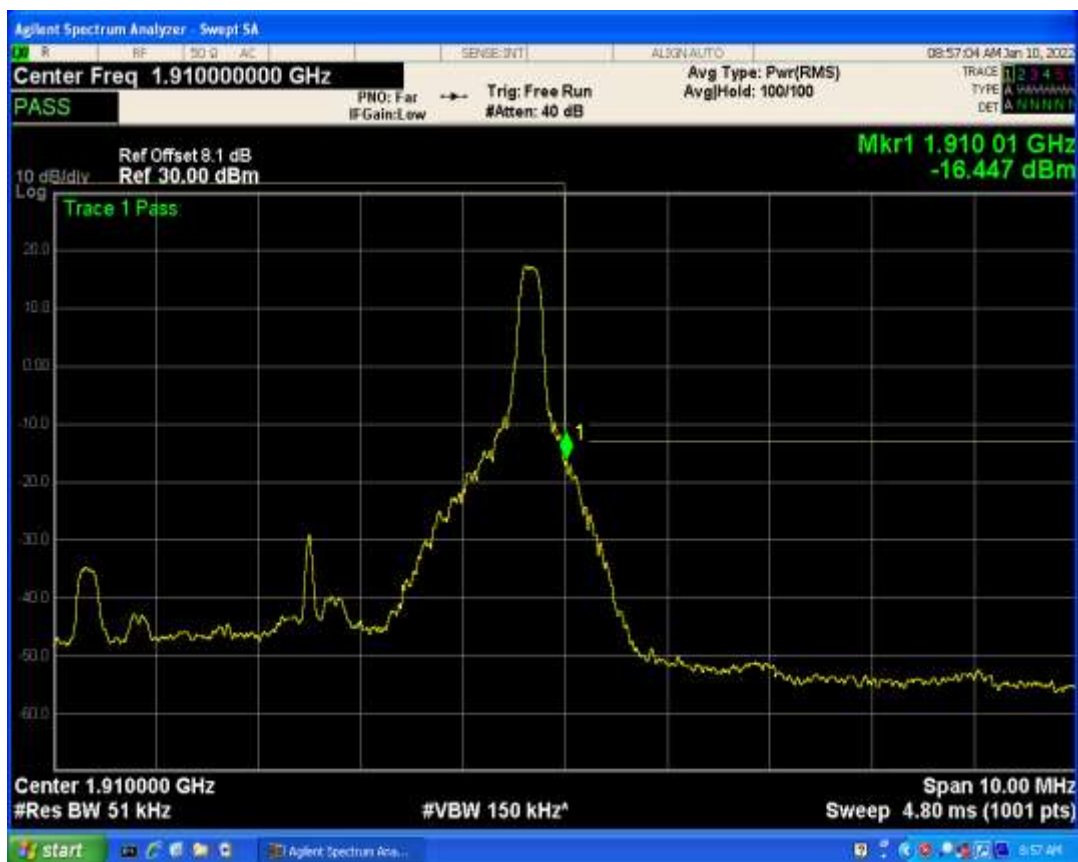
Band2 QPSK BW=5MHz Channel=19175 RB Size=25 Position=#0
