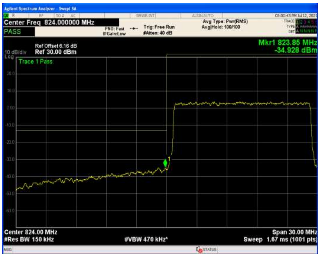
Band26b QPSK BW=15MHz Channel=26965 RB Size=1 Position=#0
