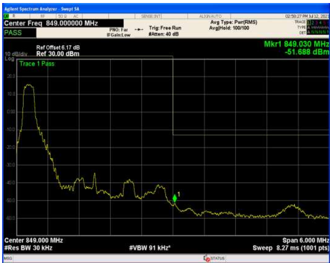
Band26b QPSK BW=3MHz Channel=26805 RB Size=1 Position=#0
