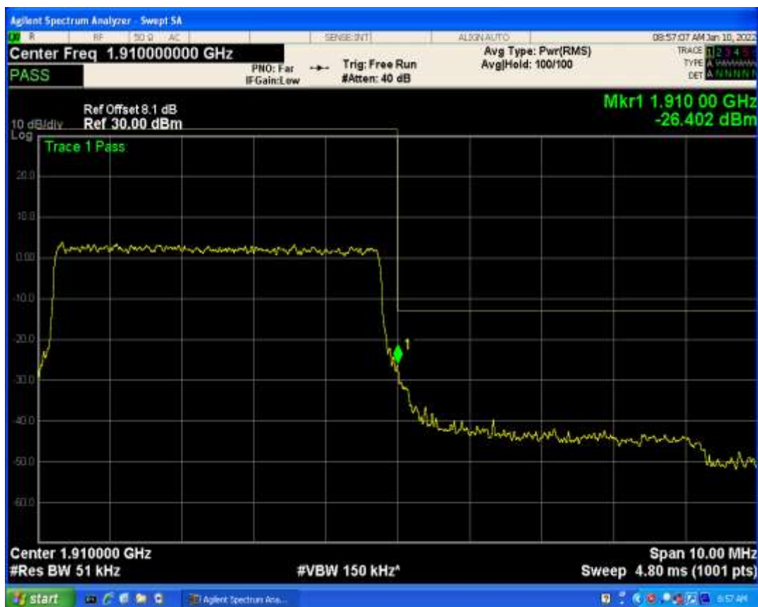
Band2 QPSK BW=5MHz Channel=18625 RB Size=1 Position=#0
