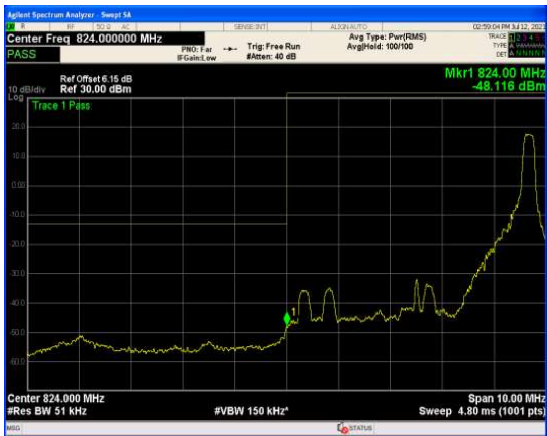
Band26b QPSK BW=3MHz Channel=27025 RB Size=1 Position=#Max
