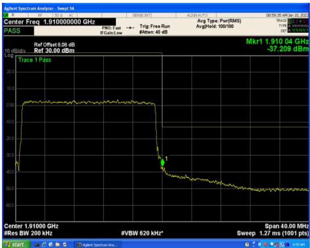
Band2 QPSK BW=20MHz Channel=19100 RB Size=1 Position=#Max
