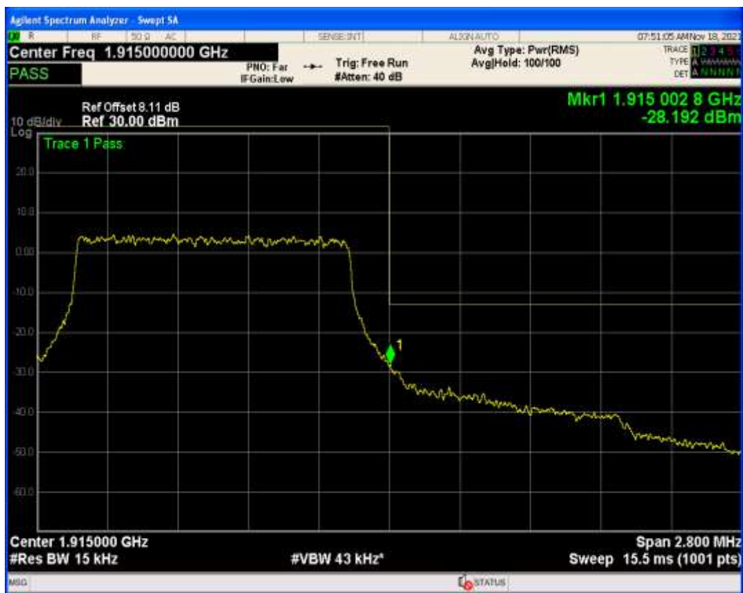
Band25 QPSK BW=1.4MHz Channel=26683 RB Size=1 Position=#Max
