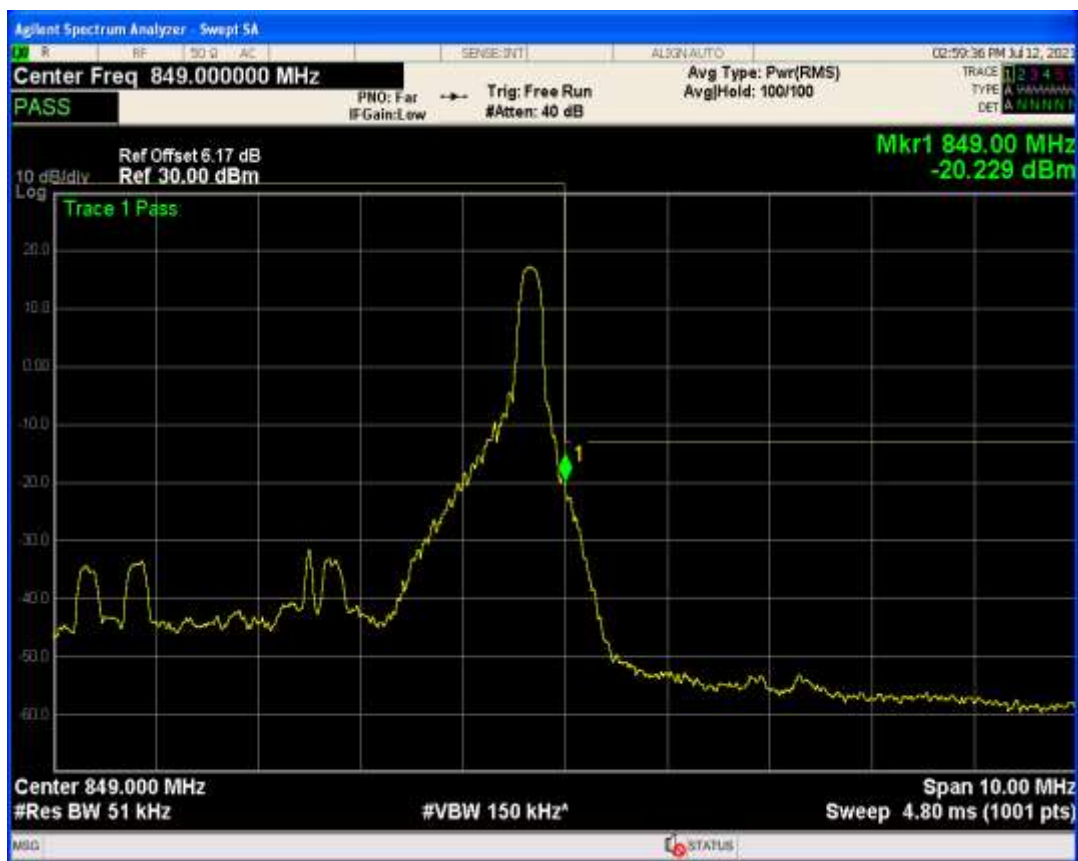
Band26b QAM16 BW=5MHz Channel=27015 RB Size=25 Position=#0
