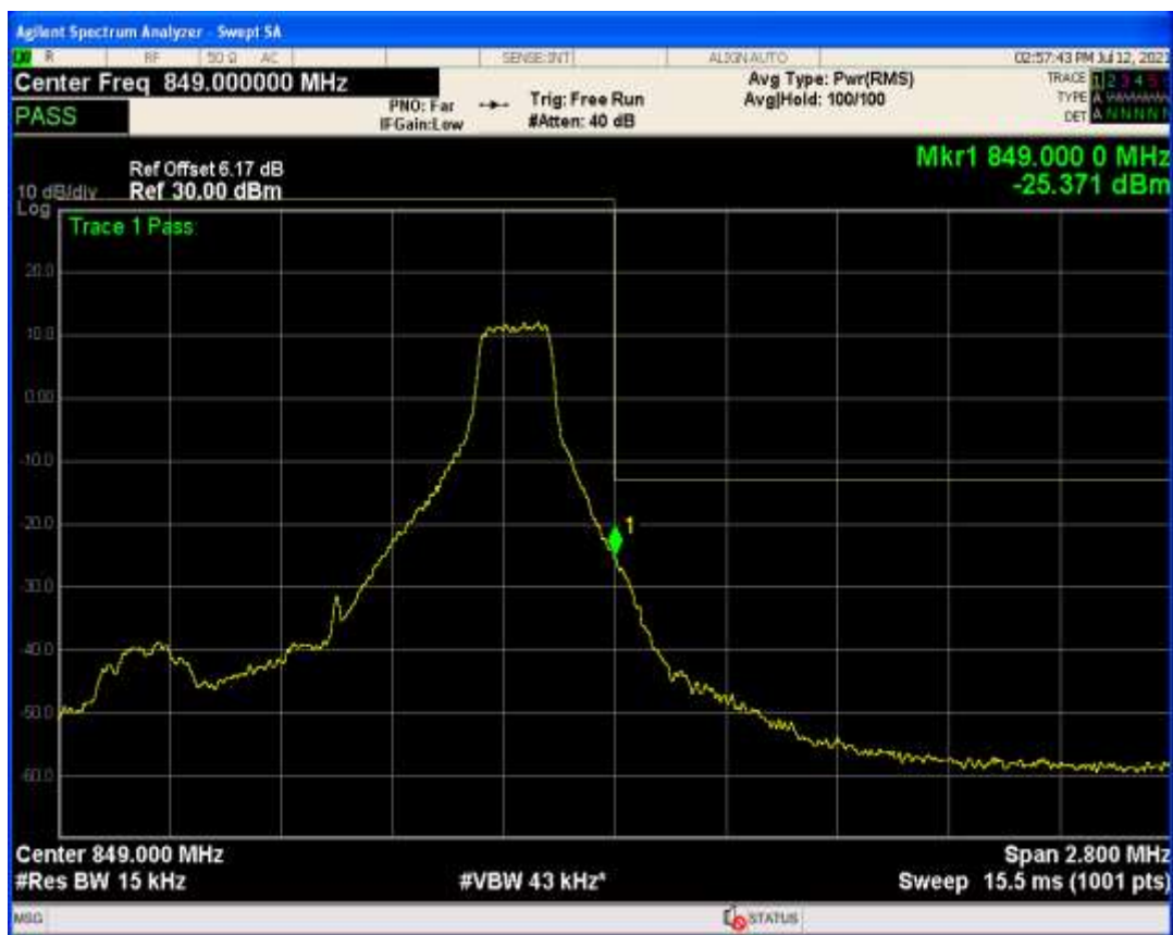
Band26b QAM16 BW=1.4MHz Channel=27033 RB Size=1 Position=#0
