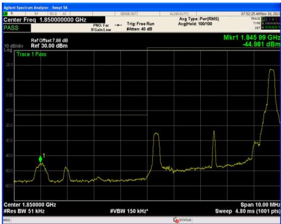
Band25 QPSK BW=5MHz Channel=26065 RB Size=1 Position=#0
