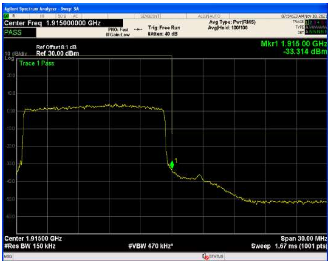
Band25 QPSK BW=5MHz Channel=26665 RB Size=1 Position=#0
