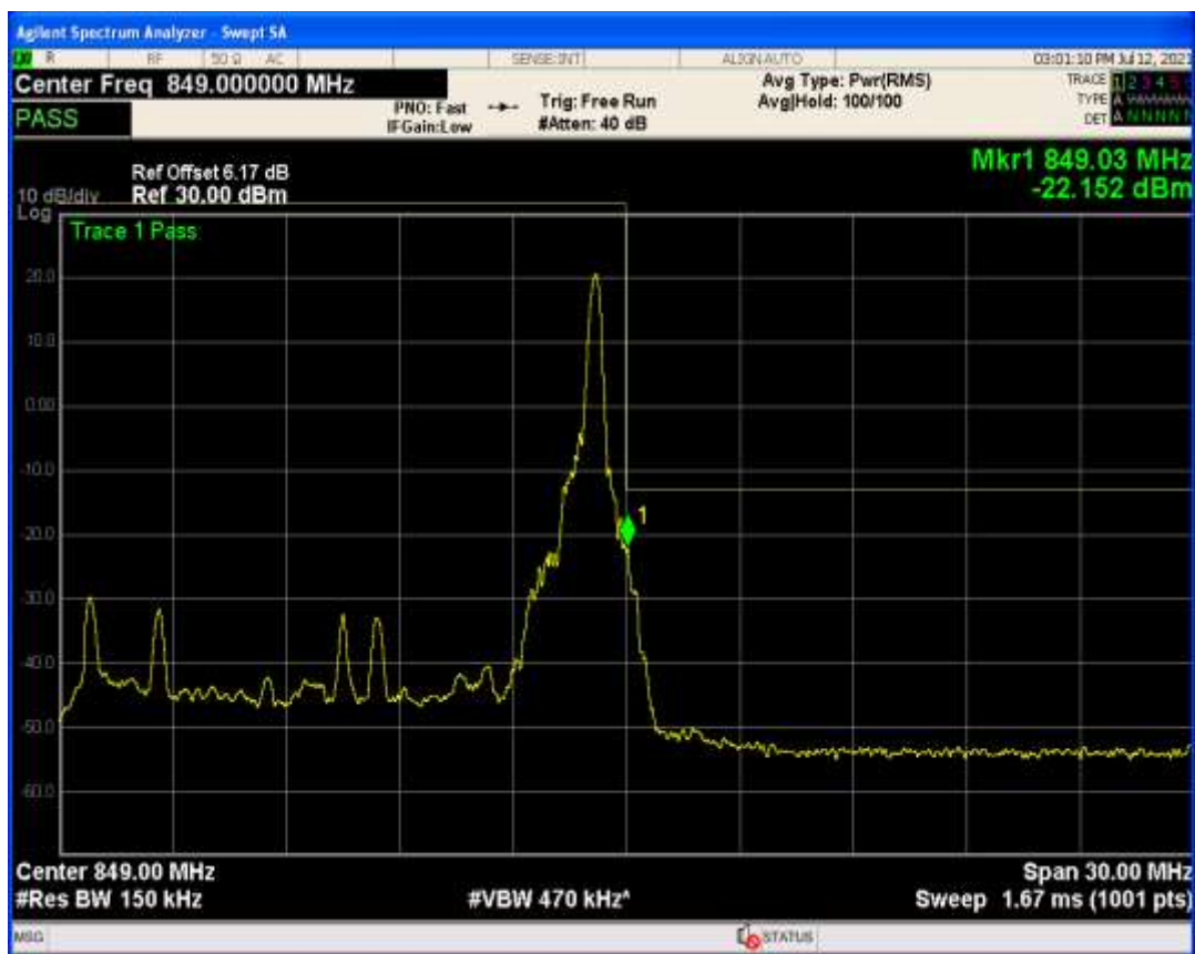
Band26b QAM16 BW=3MHz Channel=26805 RB Size=1 Position=#Max
