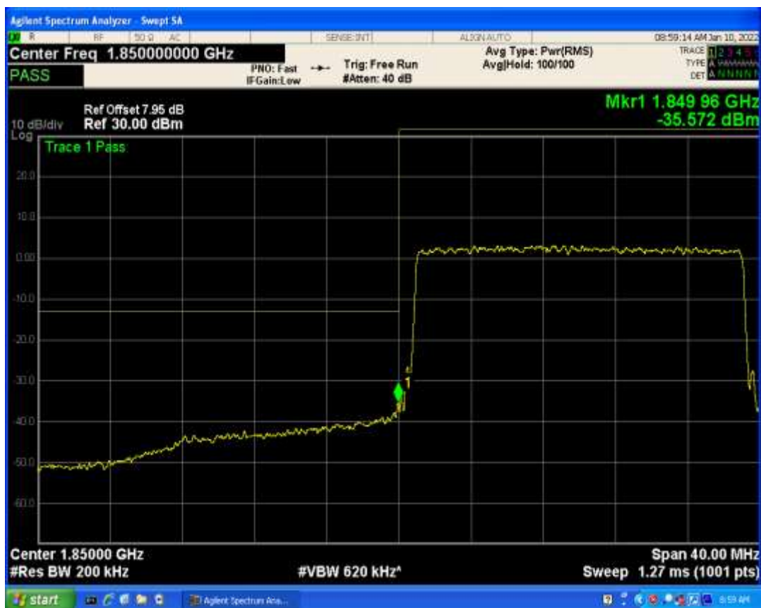
Band2 QPSK BW=20MHz Channel=18700 RB Size=1 Position=#Max
