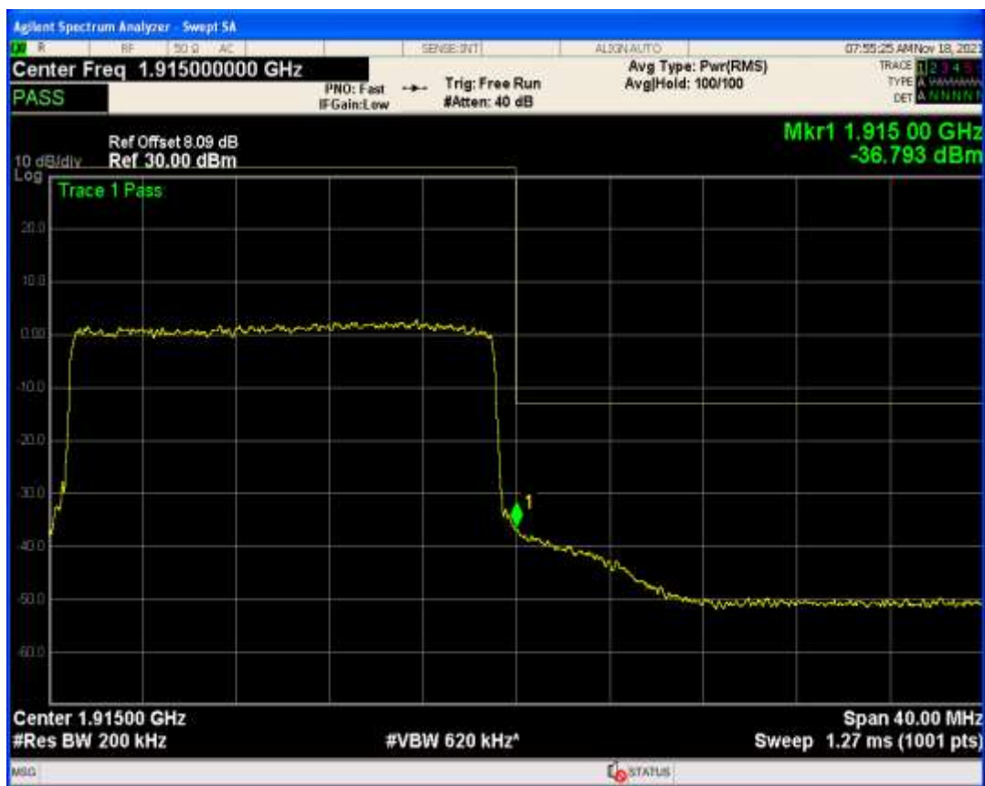
Band25 QAM16 BW=3MHz Channel=26055 RB Size=15 Position=#0
