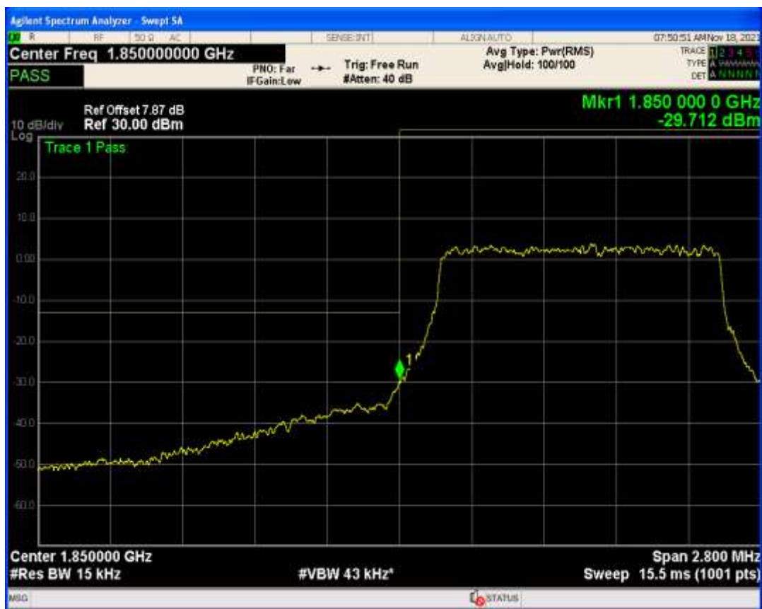
Band25 QAM16 BW=1.4MHz Channel=26047 RB Size=1 Position=#0
