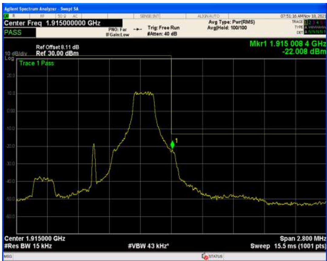
Band25 QAM16 BW=1.4MHz Channel=26047 RB Size=6 Position=#0
