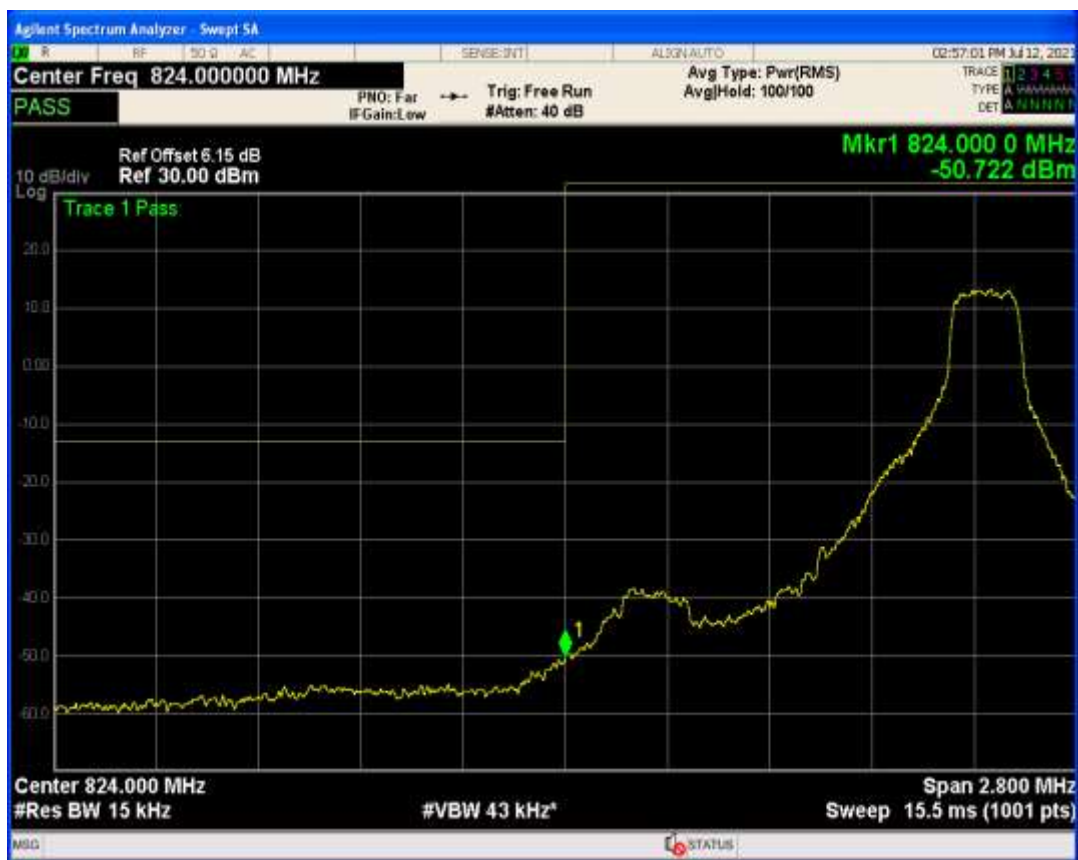
Band26b QAM16 BW=5MHz Channel=27015 RB Size=1 Position=#Max
