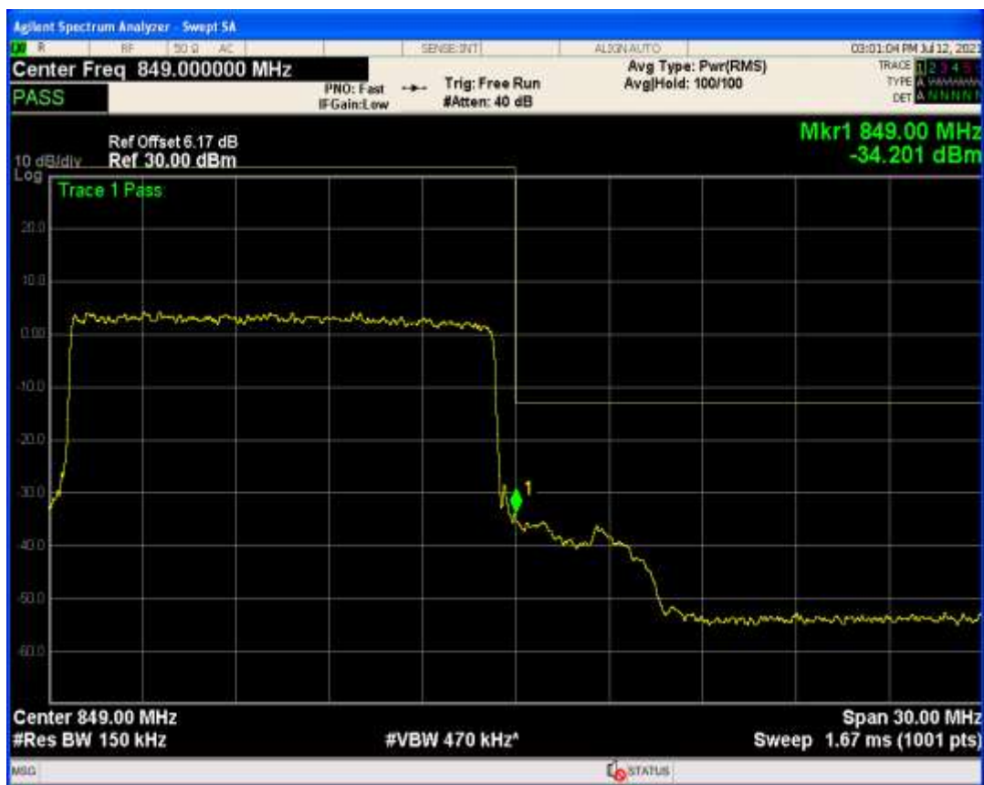
Band26b QPSK BW=15MHz Channel=26865 RB Size=75 Position=#0
