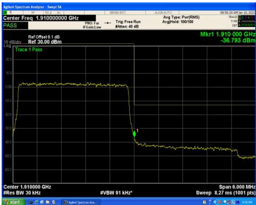
Band2 QPSK BW=3MHz Channel=19185 RB Size=1 Position=#Max
