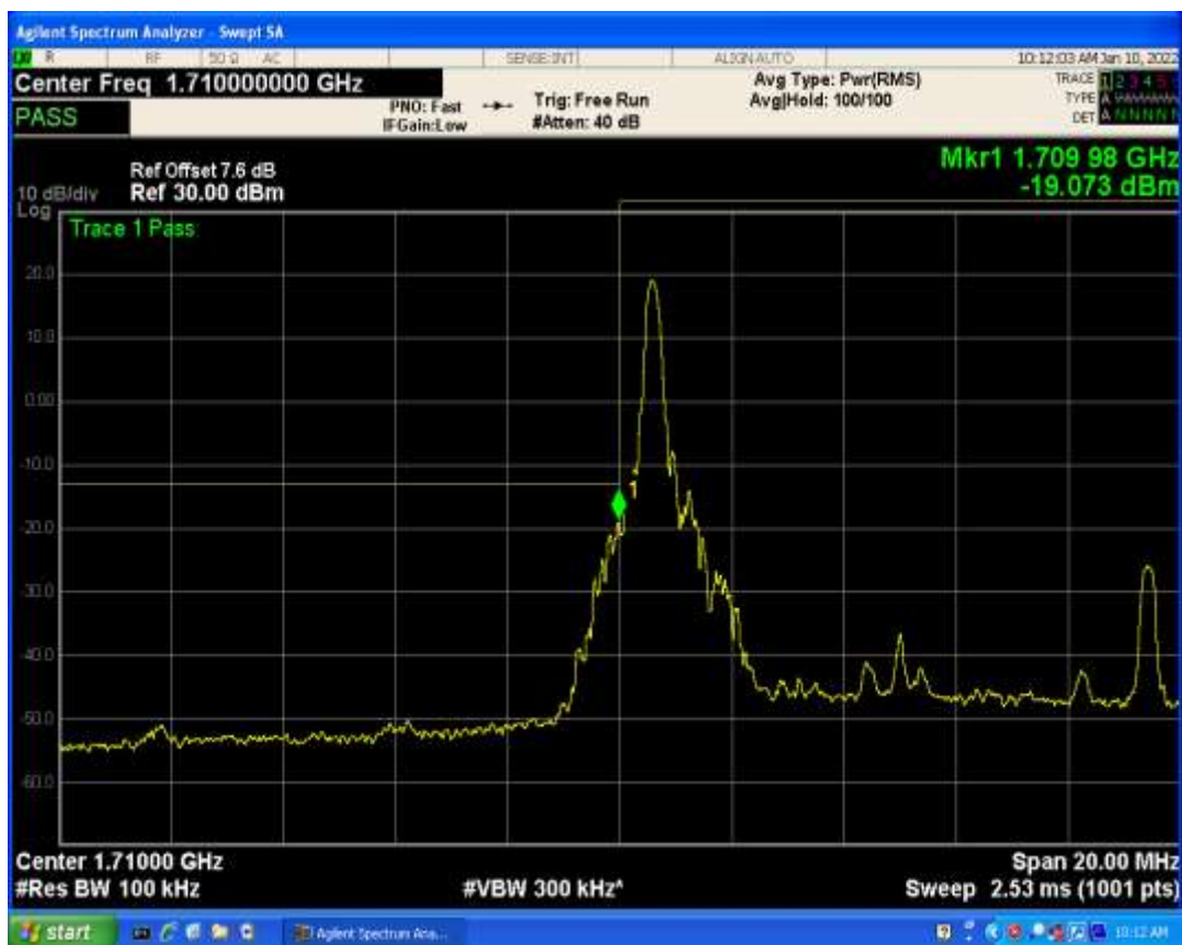
Band4 QAM16 BW=1.4MHz Channel=19957 RB Size=1 Position=#Max
