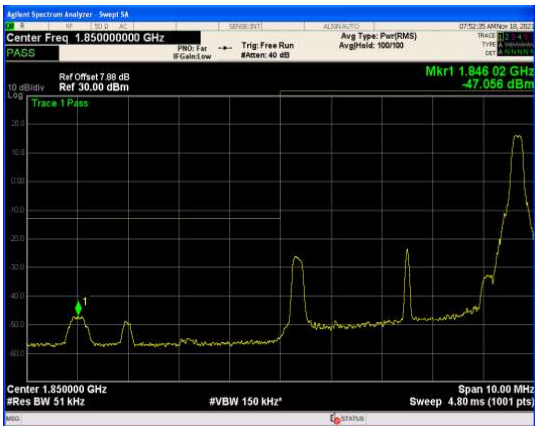
Band25 QAM16 BW=5MHz Channel=26665 RB Size=1 Position=#Max
