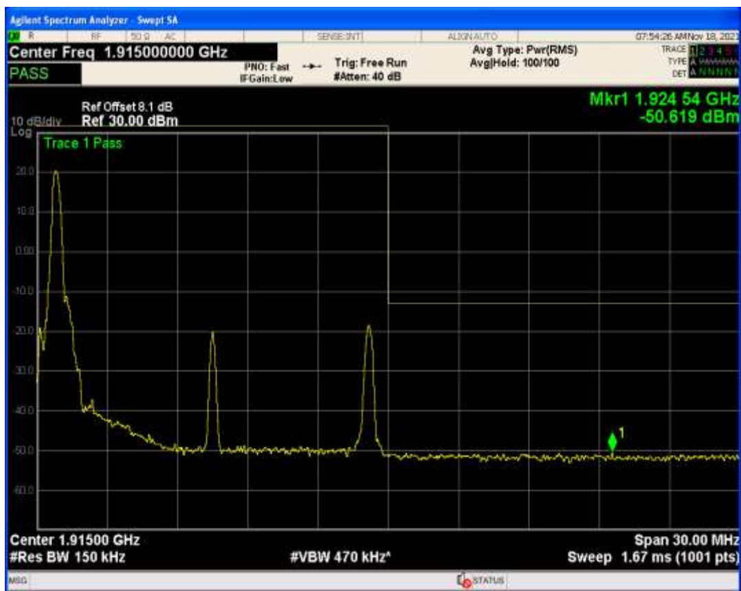
Band25 QAM16 BW=15MHz Channel=26115 RB Size=75 Position=#0
