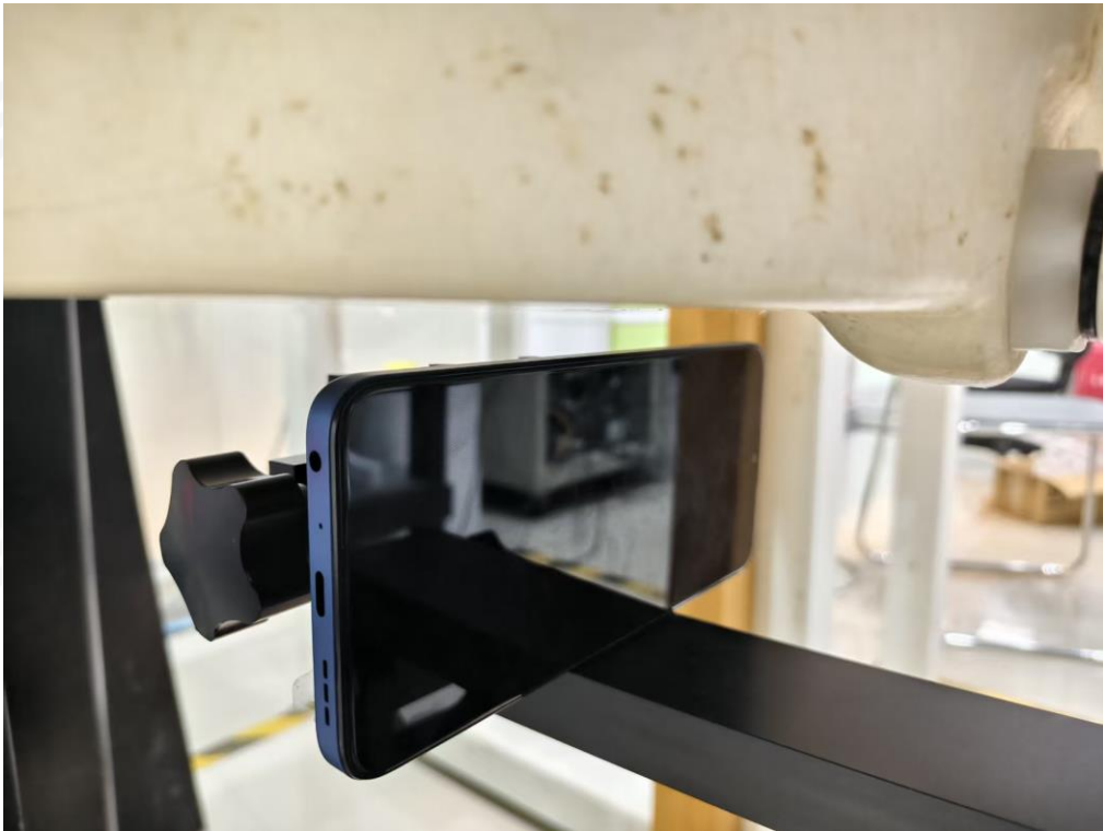
Body Left side(separation distance is 10mm)
