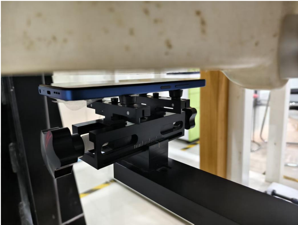
Body Front side(separation distance is 10mm)
