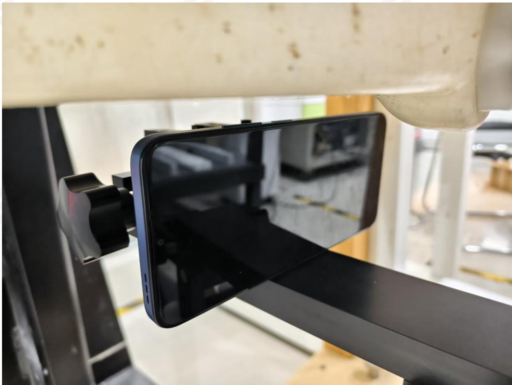
Body Right side(separation distance is 10mm)
