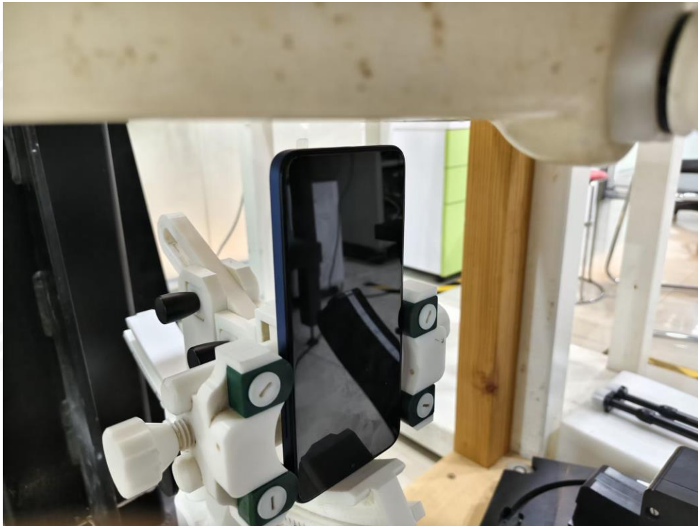
Body Bottom side(separation distance is 10mm)
