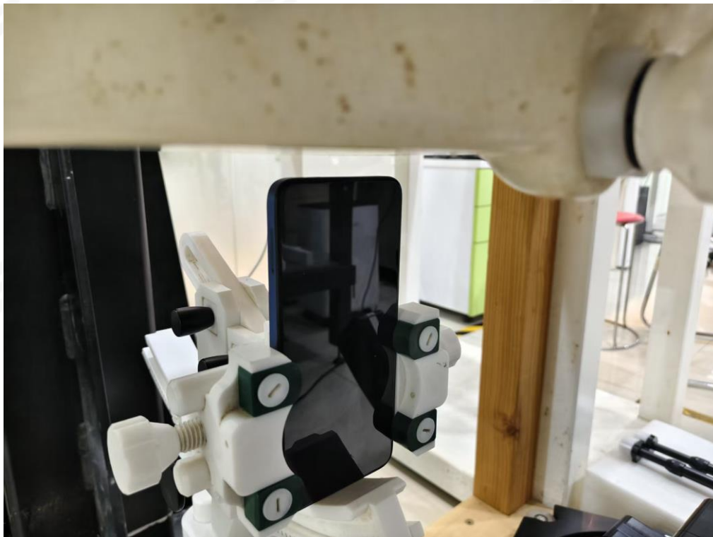
Body Top side(separation distance is 10mm)
